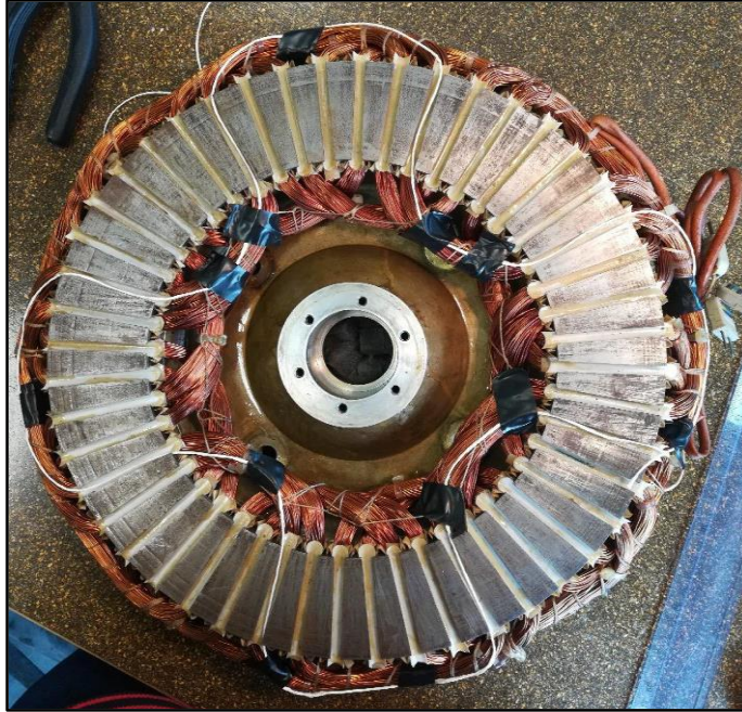
Figure 2-1: A photograph of the stator of the existing SMAFPM
