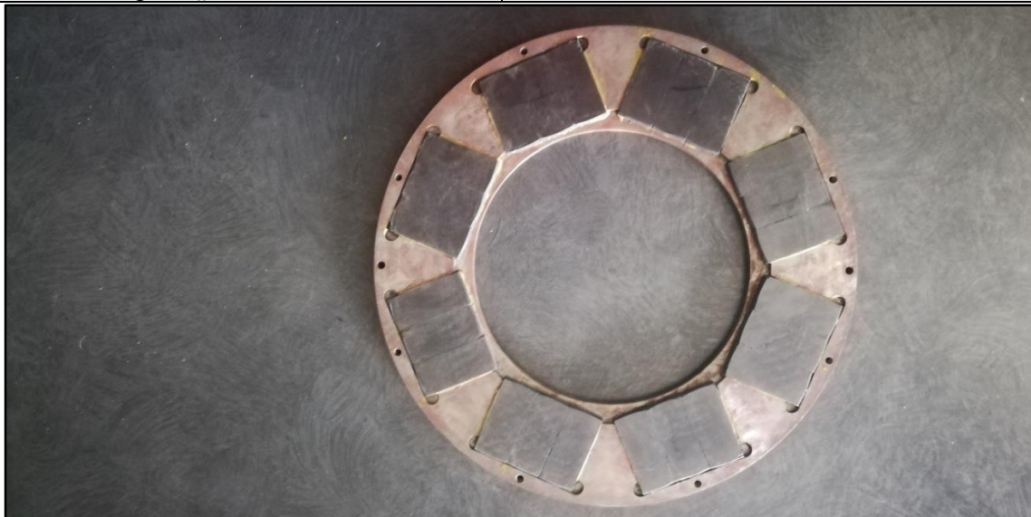
Figure 2-4: A photograph of the existing SMAFPM rotor
