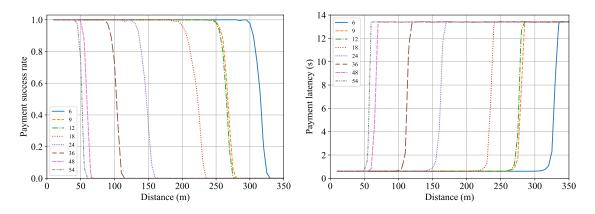
Figure 5.10: Payment success rate and latency of payments from resource-constrained devices connected via 802.11g wireless channels with different bitrates in Mb/s. When frame retransmission is deactivated, the success rate decreases with the distance from the entry node due to higher bit error rates. With retransmission, the average payment latency increases with the distance from the entry node.
