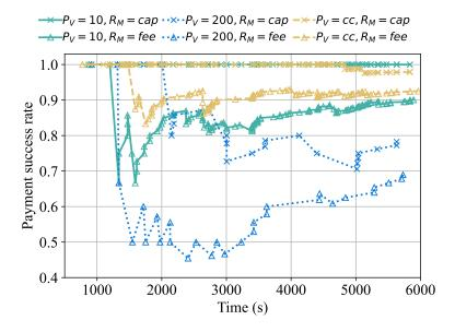
Figure 5.8: Payment success rate in our simulated PCN for several payment values  $(P_V)$  and routing methods  $(R_M)$ . The results demonstrate that Dijkstra's shortest path approach with channel capacities as weights is more effective than the Lightning Network's fee minimization approach for all cases.
