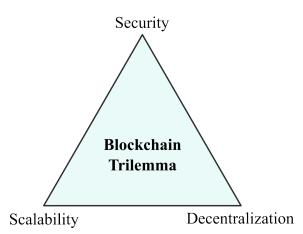
Figure 2.3: Illustration of the trilemma observed in blockchain-based systems. The trilemma states that no consensus protocol can simultaneously provide security, scalability (measured in transaction throughput), and decentralization (measured in the number of nodes participating in consensus). Graphically, all blockchains correspond to a point inside the trilemma triangle.
