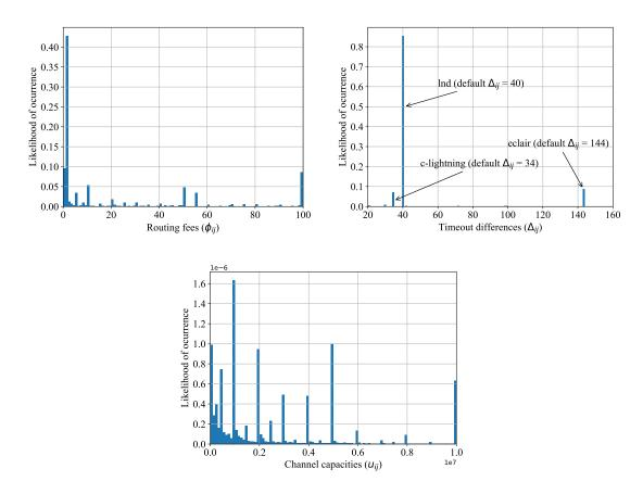
Figure 6.5: Distributions of routing fees  $(\phi_{ij})$ , HTLC-resolution delays  $(\Delta_{ij})$ , and channel capacities  $(u_{ij})$  in the Lightning Network snapshot. The peaks in  $\Delta_{ij}$ correspond to the default values of the main Lightning Network implementations [4– 6].
