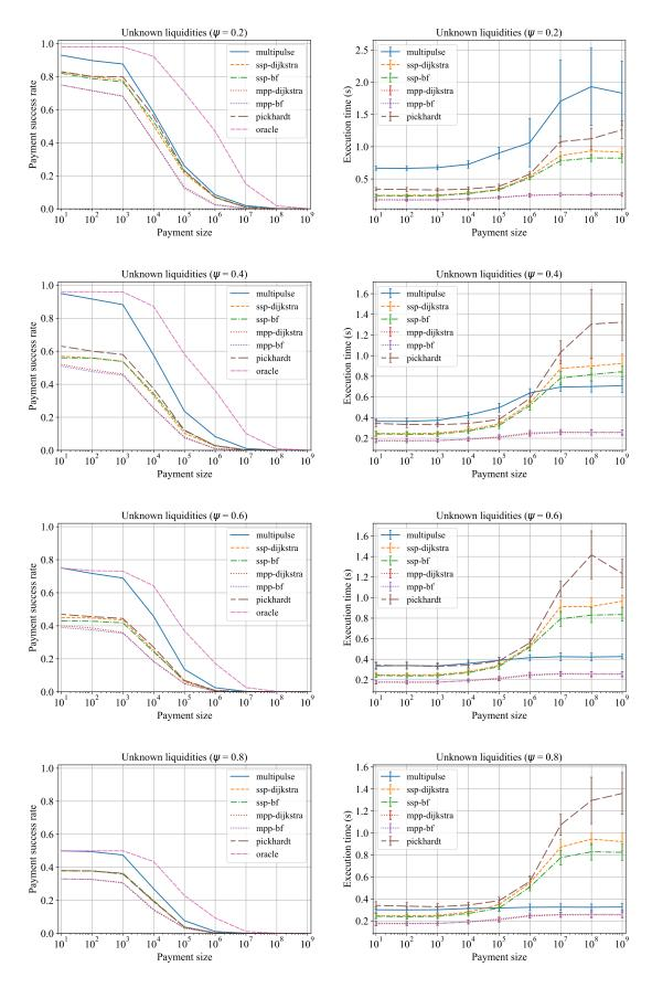
Figure 6.8: Comparison between MultiPulse and other pathfinding algorithms in the literature considering unknown liquidities.
