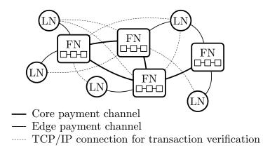
Figure 4.1: An example of a hybrid payment channel network. The light nodes (LN) represent wireless resource-constrained devices, and the full nodes (FN) represent capable nodes that store a copy of the blockchain. Light nodes establish TCP/IP connections to multiple full nodes to verify the states of their channels in the blockchain.
