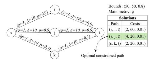
Figure 6.4: An example of constrained shortest path problem with three metrics: routing fees ( $\phi$ ), HTLC-resolution delays ( $\Delta$ ), and delivery probabilities (p). For clarity, we show the original probabilities instead of their negative logarithms, yielding a lower bound instead of an upper bound. The optimal solution is the path that minimizes the main metric while not violating any bounds.
