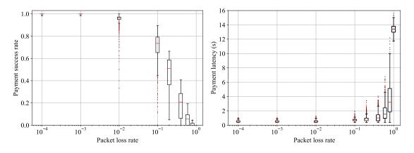
Figure 5.9: An analysis of two simulated transport protocols in PCNsim. On the left, the payment success rate degrades when sending payments over a UDP-like protocol that does not retransmit packets. On the right is the payment latency versus packet loss rate when adopting a TCP-like protocol that attempts to retransmit packets. The results show that unreliable communication channels impact the efficiency of payment channels.
