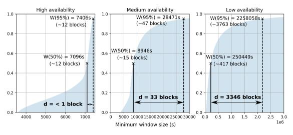
Figure 4.4: Lock time window sizes for all levels of availability with 6-block confirmation. When the availability is high, the distance d between the 50% and 95% thresholds remains below one block time, which indicates a small window is safe for most users. For medium and low availability, the distance increases significantly and forces the user to select a time window that better fits his/her security and delay needs.
