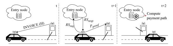
Figure 6.3: An example of a time-sensitive electronic toll collection application that adopts the proposed payment scheme. The application leverages the reduced confirmation latency to open the toll gate without stopping the car.
