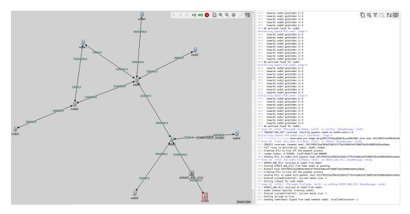
Figure 5.6: A graphical example of a PCN in our core simulator. The simulator displays logs for each node and channel in the network.
