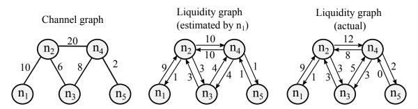
Figure 6.1: The graph structures involved in payment routing. The numbers represent edge capacities. Each node  $n_i$  transforms the public channel graph into a local liquidity graph that estimates the actual liquidities in the network.
