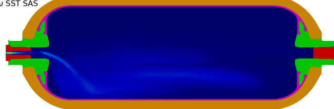
Figure 7: Scenario D10Q2. Comparison of the effective thermal diffusivity fields predicted by the k - \omega SST (upper panels) and k - \omega SST SAS (lower panels) turbulence models, at time instant: (A) 200 s, (B) 400 s and (C) 600 s.
