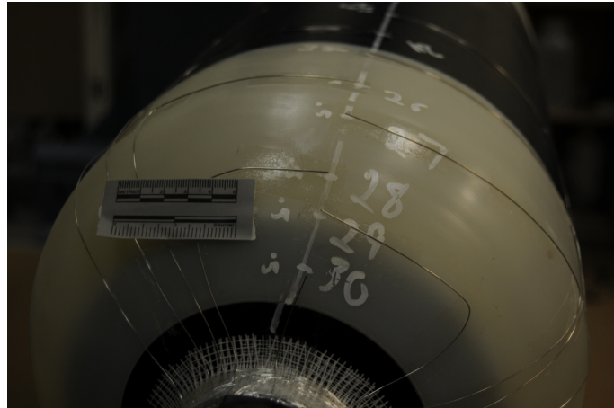
Figure 6.22 – Experimental set-up of the probes placed on the liner external surface, in contact with the composite warp for the type IV 37 L tank.
