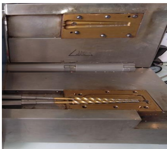
Figure IV-20 : Configuration du micro-compoundeur Thermo Scientific Haake MiniLab
