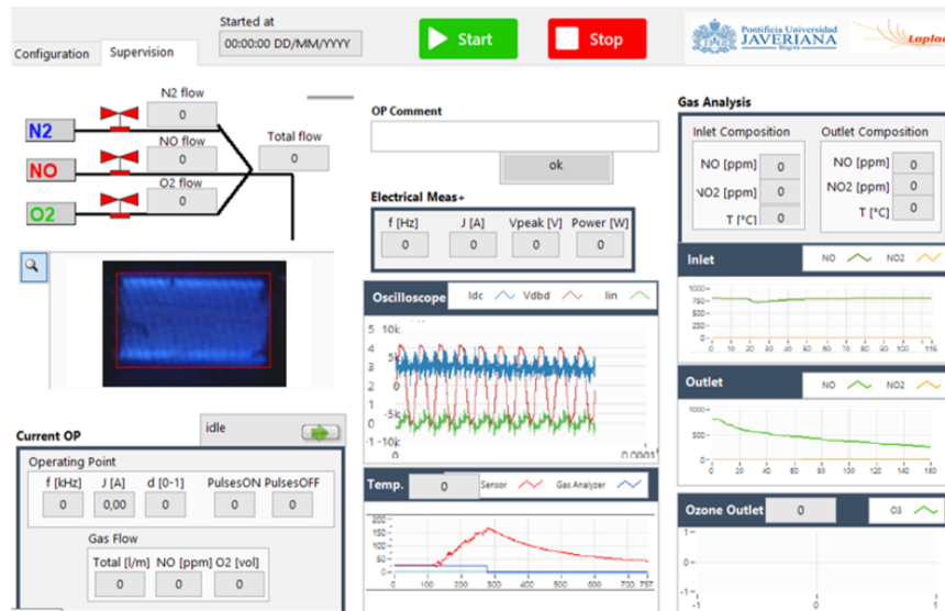
Figure 5.7: Control interface: Supervision Tab
