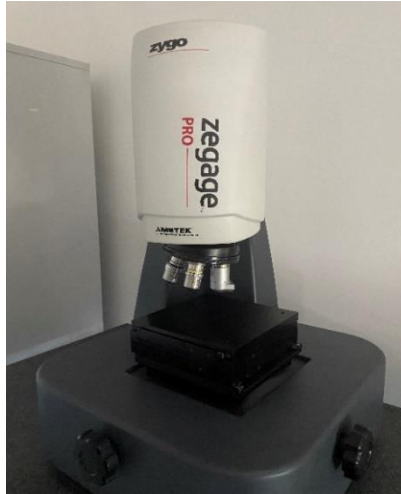
Figure 3.27: ZeGage non-contact interferometer (a), and depth scans for the volume calculation
