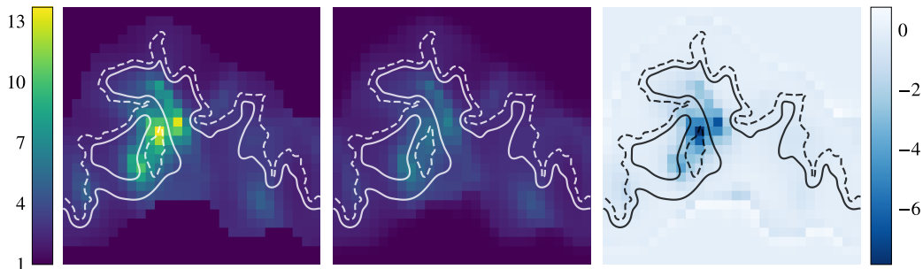
Figure 8.10: Sample slices of wrinkling factor before (left) and after (middle) corrections for flame-flame interactions, with isolines of c = 0.1 (dashed), c = 0.9 (solid). The difference between the corrected and uncorrected fields is shown on the right.
