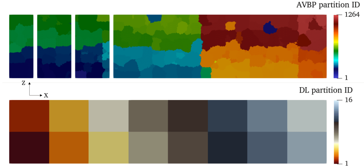
Figure 7.2: AVBP and DL partitioning on a y -normal slice at y = 1 cm. Top: AVBP partitioning (the white strips correspond to the 3 obstacle grids) with 1264 processes. Bottom: DL partitioning with 16 processes.
