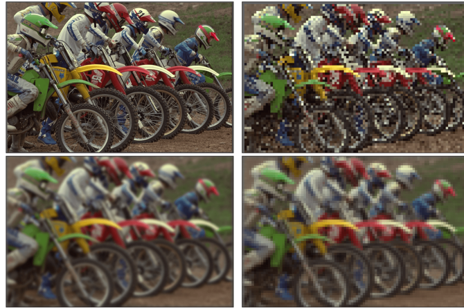
Figure 4.2: Effect of pre-filtering on aliasing of an RGB image. Top left: original image, top right: aliased image, bottom left: filtered image, bottom right: filtered and downsampled image.
