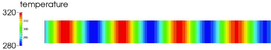
Figure 5.4: Instantaneous temperature flow field of the 2D test case.
