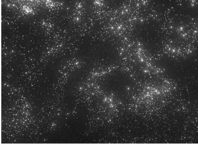
Figure 2.2: Experimental image of a laser sheet going through a spray at St = 0.6 for isotropic homogeneous turbulence, showing the preferential droplet segregation phenomenon, taken from [320].
