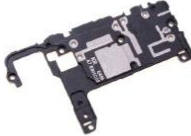
Figure 1.18: Antenna module of Samsung Galaxy Note 10 fabricated using LDS
