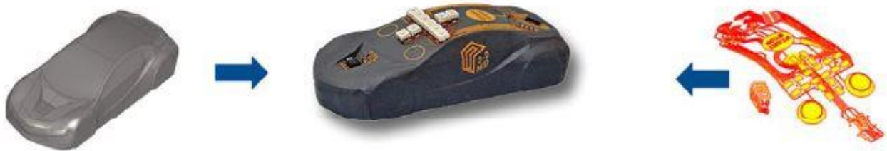
Figure 0.2: Example of a plastronic device assembling from plastic model (left) and electric circuit (right) [8]
