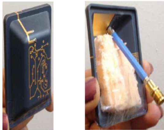
Figure 1.19: 3D PIFA antenna on LCP Vectra E820i fabricated by LDS
