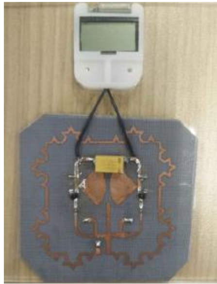
Figure 2.4: Designed EM energy harvester in [65]
