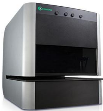
Figure 3.14: X-ray fluorescence of Bowman used to measure the conductor's thickness
