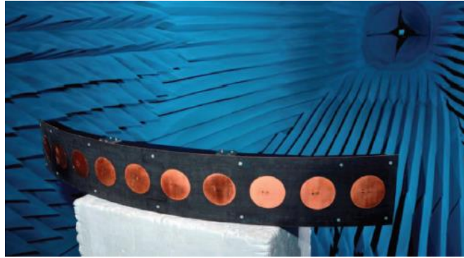
Figure 1.23: The nonplanar patch array with copper plated elements on a 3D-printed substrate [50]
