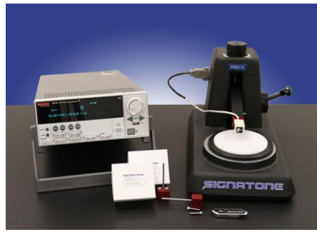
Figure 3.17: Four probe station by Signatone used to measure the resistivity of conductor
