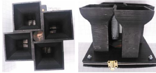
Figure 1.26: Printed of array horn antennas by PLA material [54].
