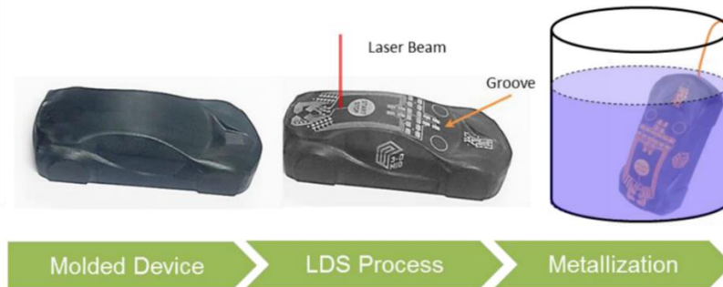
Figure 1.13: Steps of fabricating the object using LDS [8]
