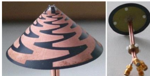
Figure 1.22: Log-periodic four arm antenna realized on MID substrate [49].
