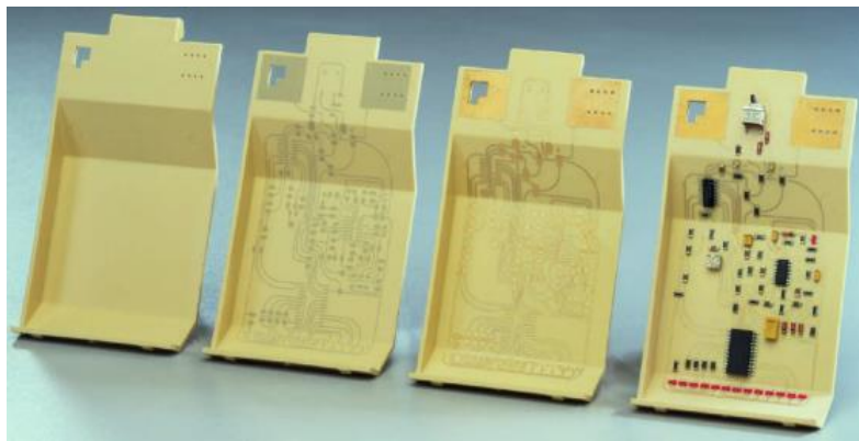
Figure 1.14: Different steps of realizing a plastronic device using LDS: molding, activation, metallizing and components mounting [40]
