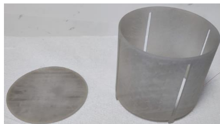
Figure 3.7: The objects with the treated surfaces (the surfaces turned to black because of the treatment process).
