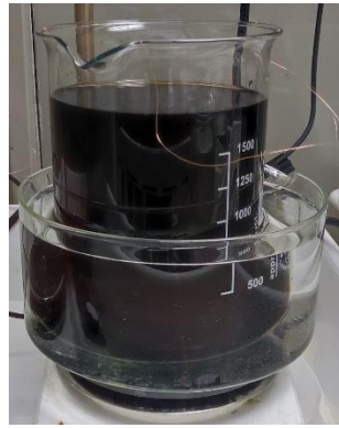
Figure 3.8: The objects are immersed in the tank of Pd.
