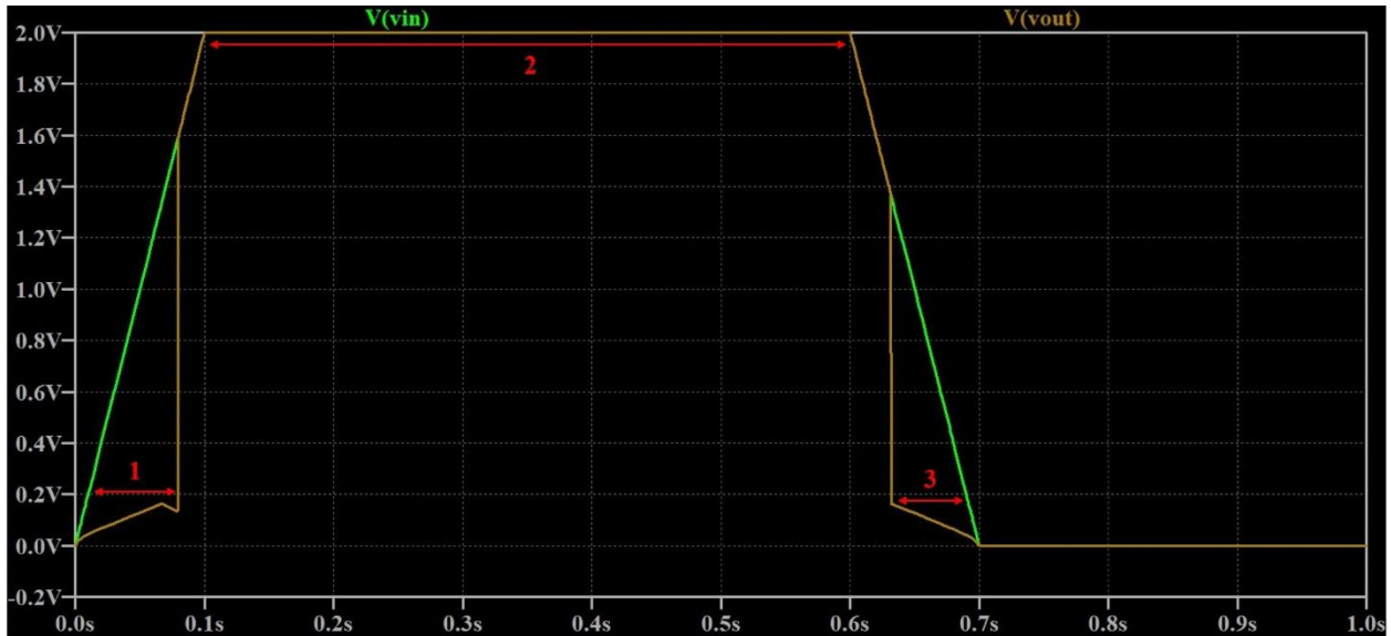
Figure 5.22: Simulated waveform results of Under-Voltage-Lock-Out
