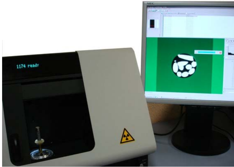
Fig. 4-9. X-ray tomography device (Skyscan 1174 type) used in this study
