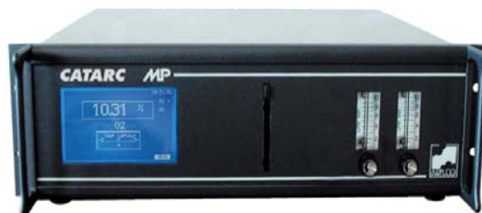
Fig. 4-3. Katharometer used in this study (CATARC MP – R)
