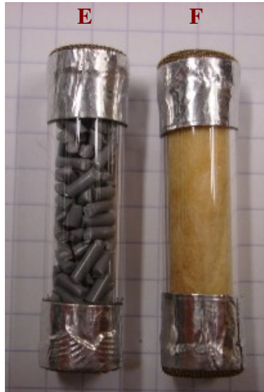
Fig. 4-23. Cylindrical samples filled with different materials producing different tortuosity but the same porosity \varepsilon=66\% (E: cylindrical material and F: glass wool)
