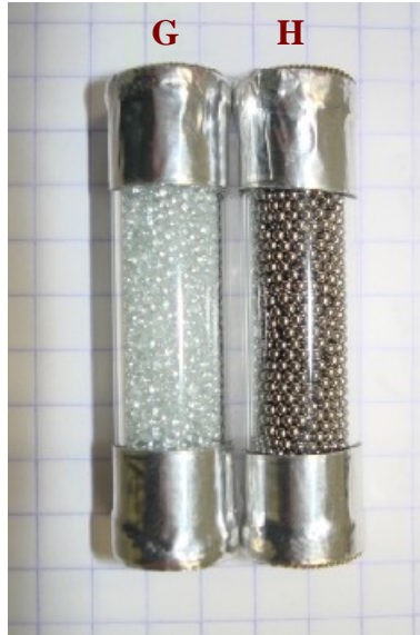
Fig. 4-18. Cylindrical samples filled with different materials (H: stainless steel, G: glass spheres and \varepsilon=42.5 )
