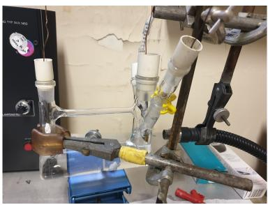
Figure 6.19: Photograph of the setup used for photoelectrochemical measurements.
