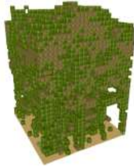
Figure 3-6: 25 m x 25 m turbid mockup derived from LiDAR point cloud of SERC forest (USA) with pure green voxels (leaves or wood) and mixed brown voxels (leaves and wood).
