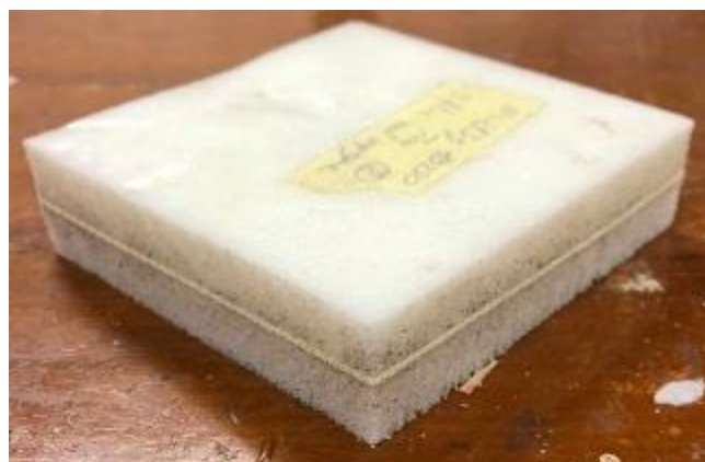
Figure A- 4: Structure with three aramid plies in the middle after being cut
