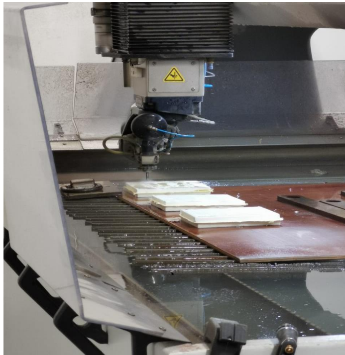
Figure A- 3: Hybrid structure cutting process with a water jet machine
