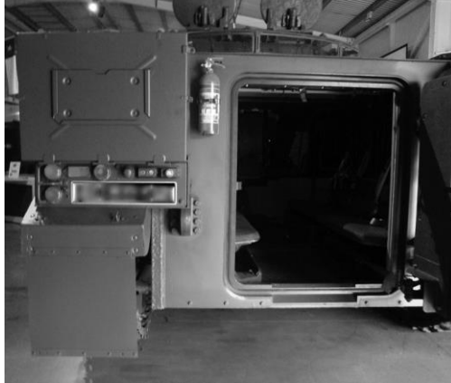
Figure I-8: Rear of a military vehicle made from an aluminum alloy plate [18].
