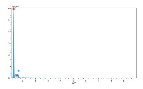
Figure 4.20: SEM-EDX spectrum for virgin CBD electrode.
