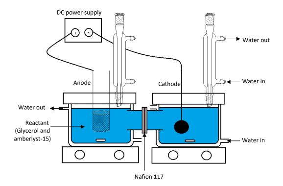
Figure 3.2: Electrochemical set-up (two-compartment reactor).
