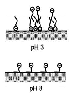
**Figure 2.3.** Effect of pH on the rejection of anion species on charged membrane (Childress *et al.*, 2000).
