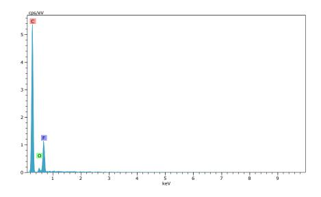
Figure 4.17: SEM-EDX spectrum for virgin ACC electrode.
