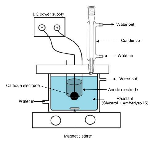
Figure 3.1: Electrochemical set-up (one-pot reactor).
