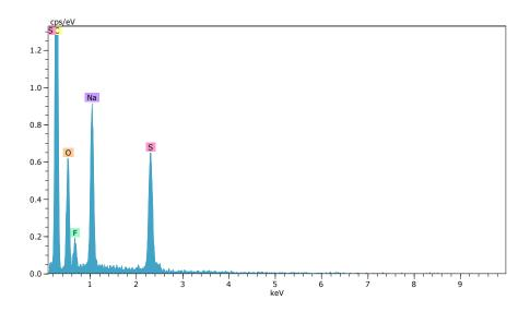
Figure 4.18: SEM-EDX spectrum for ACC electrode after the electrochemical reaction.
