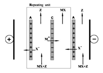
**Figure 2.5.** Schematic represents the electro-dialysis process for concentrate organic acids or organic salts. MX: organic acid or salt; Z: neutral substances or low concentration of inorganic salts (Huang *et al.*, 2007).
