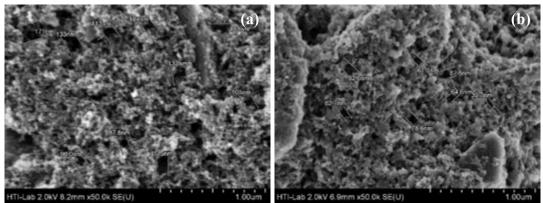
**Figure 4.16:** SEM images of (a) virgin ACC electrode and (b) ACC electrode after the electrochemical reaction.
