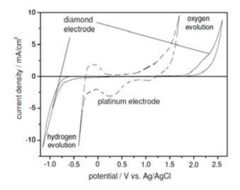
Figure 2.2. Cyclic voltammetry curves of platinum and diamond electrode in 0.2 M  $H_2SO_4$ , v = 0.1 Vs<sup>-1</sup> (Kraft, 2007).
