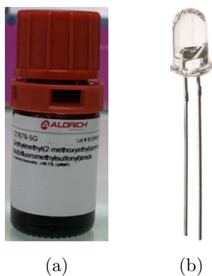
Figure 2.28: Different tools used for doping control. (a) Ionic liquid Diethylmethyl(2-methoxyethyl)ammonium bis(trifluoromethylsulfonyl)imide. (b) UV LED of wavelength \lambda = 375 nm.
