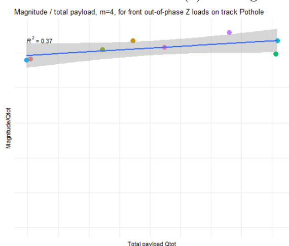
(b) Pothole track, front out-of-phase vertical loads
