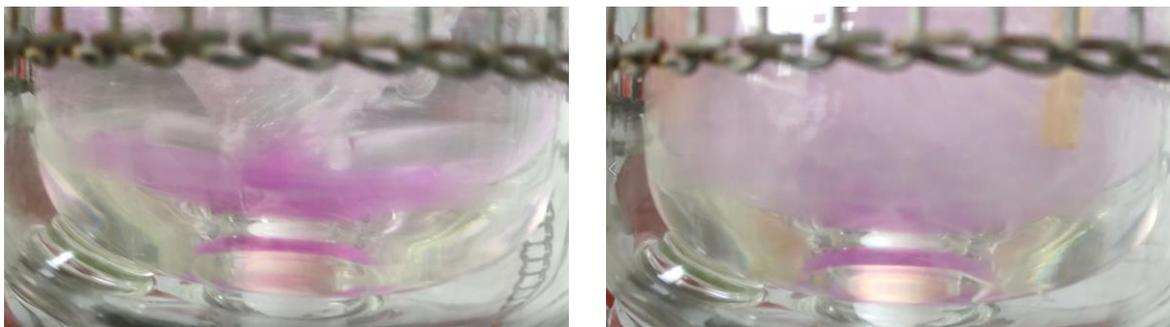
*Figure 4-11: snapshots of the two immiscible solvents being stirred at 400 rpm with a glass propeller without baffles (left) and with baffles (right)*
