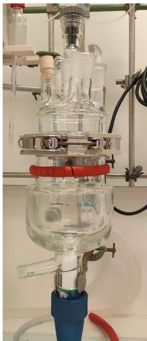
Figure 4-6: Picture of the HWS flat flange crystallizer use to perform spherical agglomeration of SAFIM
