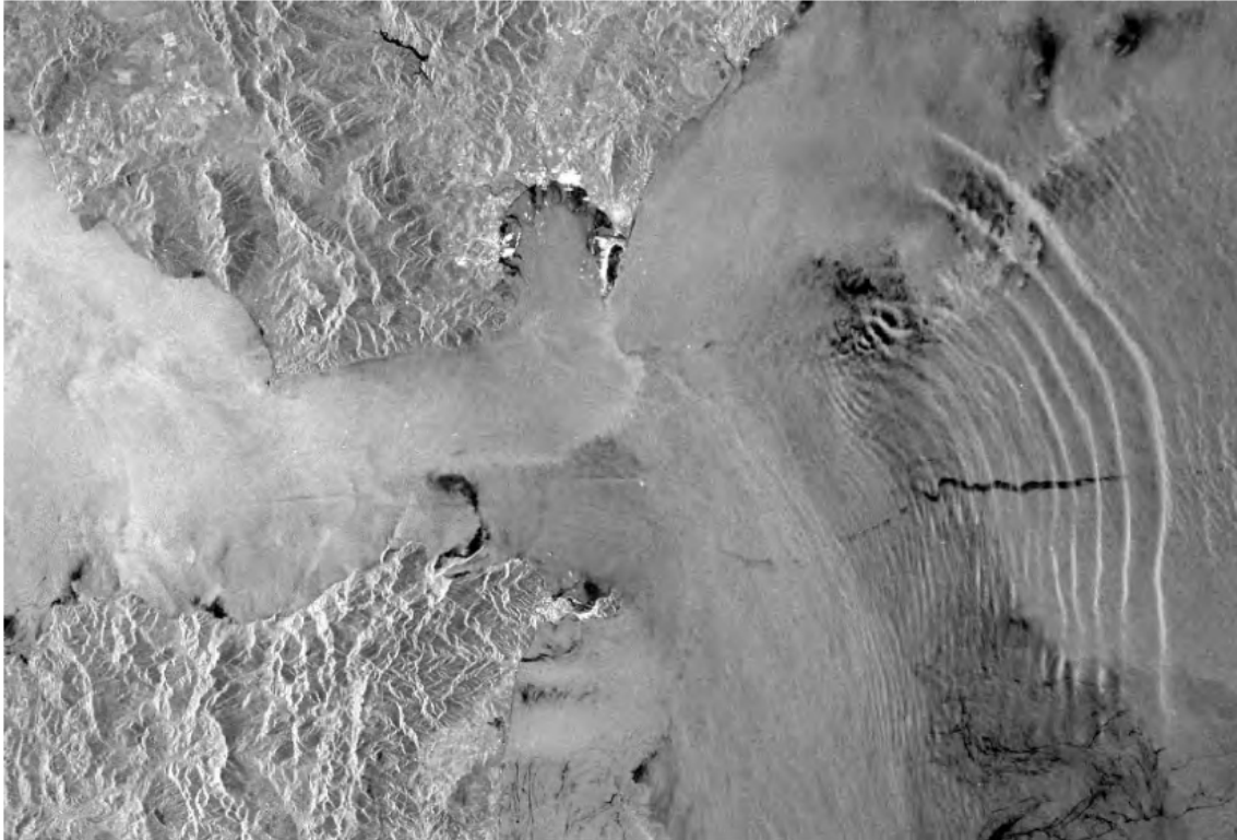
Figure 1.5: ERS-1 SAR image acquired on 1 January 1993 at 22:39 UTC (orbit: 7661) showing sea surface manifestations of a packet of internal solitary waves generated in the Strait of Gibraltar and propagating eastward into the Mediterranean Sea. The dark line intersecting the packet results from an oil spill, probably released from a ship. Imaged area: 100 km \times 50 km. ©ESA. Figure and legend from Alpers et al (2008)
