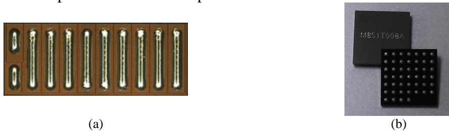
Figure 4.28 : Boîtiers de composants GaN (a) EPC - LGA (Linear Grid Array) (b) Fujitsu - BGA (Ball Grid Array)
