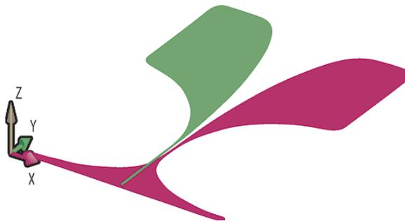
Figure I-19: Antenne Vivaldi antipodale [I-19]
