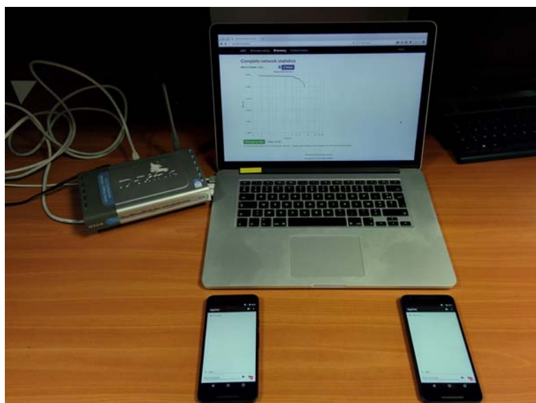
Figure 7.3: View of the actual system, made of a central computer, a WiFi access point and two real devices as Nexus 5X smartphones running the opportunistic application being tested.
