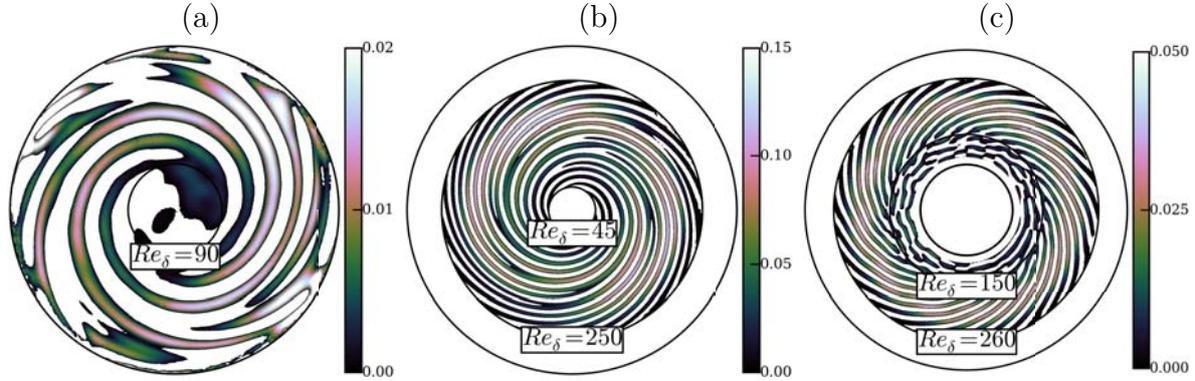
**Figure 3.8** – Snapshots of the dimensional axial velocity fluctuations  $\tilde{u}_z$  in the stationary disc boundary layer at  $z^* \simeq 1 - \delta/h$  for (a) **Case 1**, (b) **Case 2** and (c) **Case 3**. Labels indicate radial positions of interest and/or the radial extent of the patterns. Bold circles without labels mark the limits of the computational domain.
