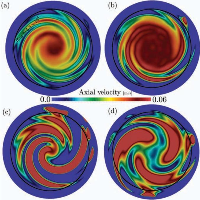
**FIGURE 13.**  $(r/R_1, \theta, z/h = 0.025)$  slice colored by  $u_z$  with relevant notations. From (a) to (d), configurations  $MR_1$  to  $MM_2$ , respectively.  $Re_{II}$  indicates the outermost Reynolds number of flow coherence observed in all four configurations.
