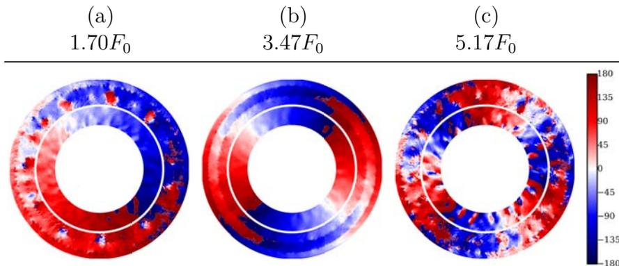
**Figure 4.30** – Isocontours of the phase of the pressure fluctuations  $\arg(\tilde{P}_s)$  for (a)-(b) the two major DMD modes and (c) the least noisy extra DMD mode constituting **Case 2**, sorted out by their respective frequencies.
