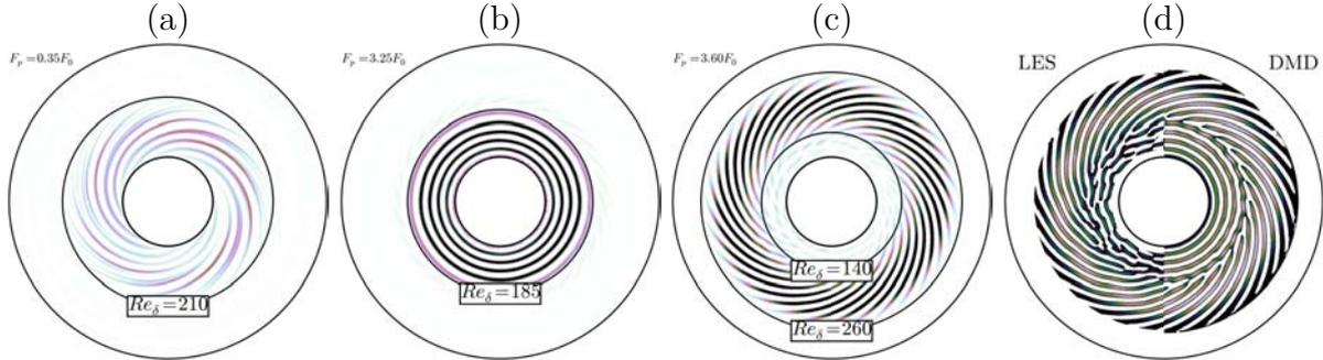
**Figure 3.15** – Isocontours of  $\tilde{u}_z \in [0, 0.05]$  at  $z^* = 1 - \delta/h$  (stator) for (a,b,c) the three major DMD modes constituting **Case 3** sorted out by their respective frequencies and (d) a composite made of the LES prediction compared to the combination of the three DMD modes. Values outside the colour range have been blanked out. To improve visibility, the colour scale has been inverted for (d).
