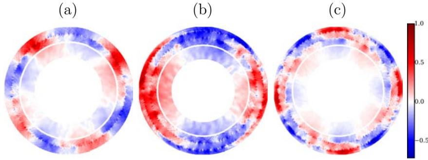
**Figure 4.33** – Isocontours of the pressure fluctuations  $\tilde{P}_s$  obtained by combination of the constituent DMD modes in (a) **Case 1**, (b) **Case 2** and (c) **Case 3**. The scalar fields have been normalized by their maximum values.
