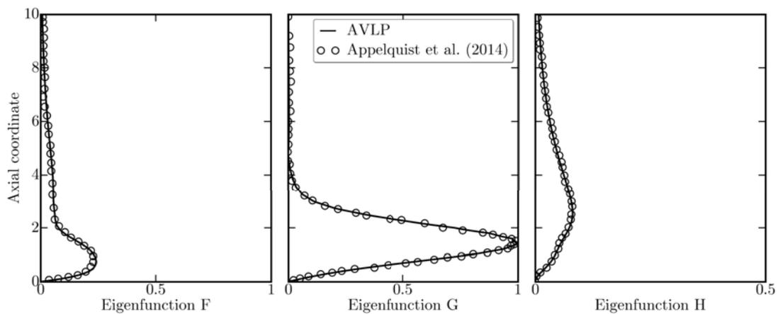
**Figure 2.19** – Eigenfunctions for  $Re_\delta = 430$ ,  $m = 32.35$ ,  $\alpha_r = 0.3618$ ,  $\omega = 0.0041i$ . Solid lines indicate the present results of AVLP. Local linear stability results from Appelquist & Imayama (2014) ( $\circ$ ) are given as reference.
