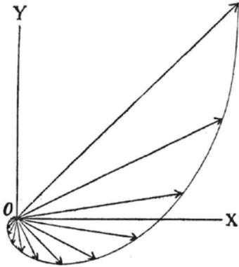
**Figure 2.1** – Illustration of the "Ekman spiral". The direction and velocity of the flow current at different depths within the boundary layer are represented by the arrows, the longest arrow referring to the surface where the drift-current is directed  $45^\circ$  to the right (resp. left) of the velocity of the wind in the northern (resp. southern) hemisphere. The direction of the  $y$ -axis is the direction of the wind-velocity relative to the water. Source: [Ekman \(1905\)](#).
