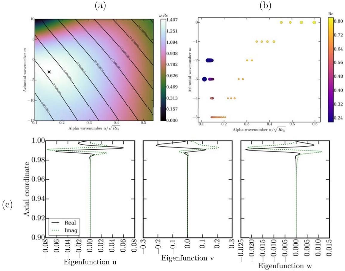
**Figure 3.26** – Results of the temporal stability analysis ( $\alpha_i = 0$ ) in **Case 1**, ‘stator branch’. (a) Amplification rate  $\omega_i Re$  map overlaid with frequency  $-\omega_r Re$  contours at  $Re = 0.495$ . (b) Progression of the most amplified point with the local Reynolds number  $Re$  (marker colour), characterized by the value of the amplification rate (marker size). (c) Example of eigenvector taken at the maximum of amplification.
