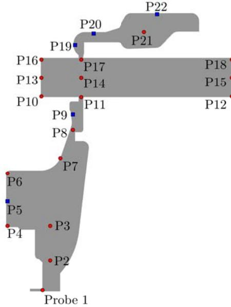
**Figure 4.22** – Locations of the numerical probes. Each symbol corresponds to 60 equireparted azimuthally. Blue squares match the locations of probes used during the benchmarking campaigns. Red circles are additions to cover all the cavity.
