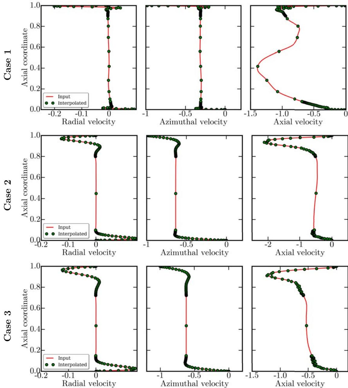
**Figure 3.25** – Axial profiles of the three velocity components (radial, azimuthal and axial resp. from left to right) for **Case 1**, **Case 2** and **Case 3** (resp. top to bottom). Extraction made at  $r^* = 0.5$ . The distribution of collocation points used in AVLP is indicated by the markers.
