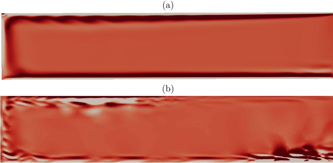
**Figure 3.21** – Isocontours of the fluctuations of azimuthal vorticity  $\eta$  in a meridional cut ( $r^*, \theta = 0, z^*$ ) from (a) the LES solution ( $\eta \in [-2.0, 2.0] \times 10^3$ ) and (b) only the first constituent DMD mode pulsing at  $2\pi F_1 - \Omega$  ( $\eta \in [-30, 30]$ ).
