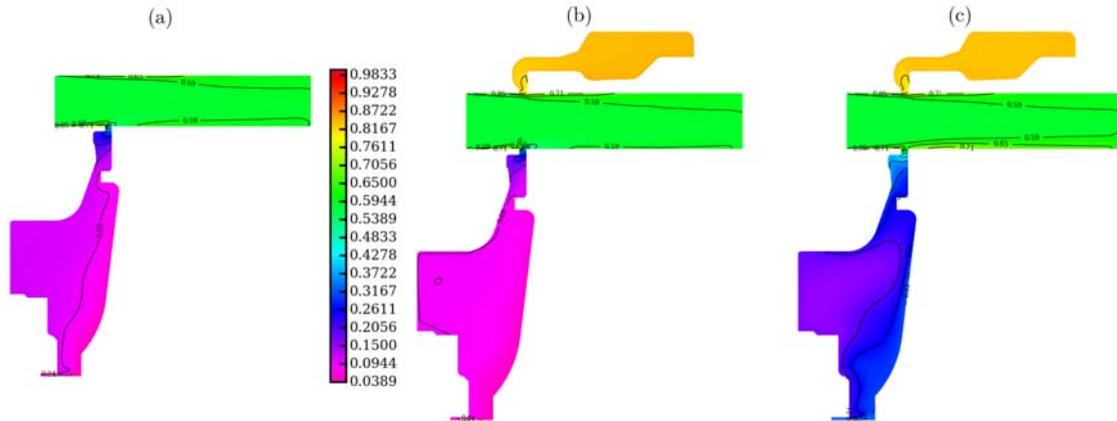
**Figure 4.16** – Contours of the averaged static temperature  $\bar{T}_s$  for (a) **Case 1**, (b) **Case 2** and (c) **Case 3**. The range indicated in (a) is valid in all three cases.
