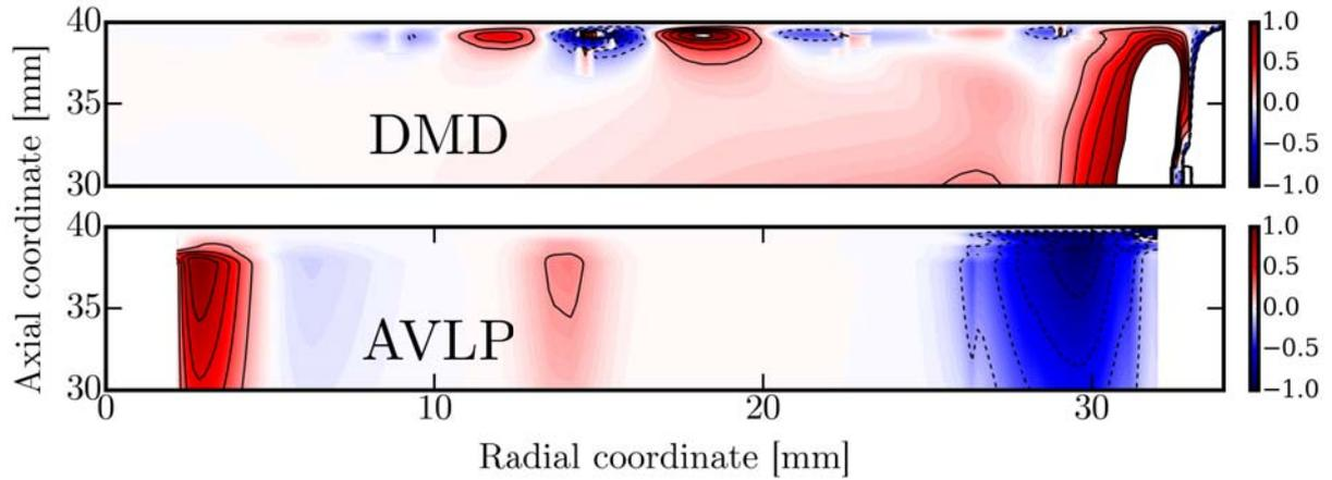
**Figure 3.46** – Fluctuating axial velocity of the global stator mode  $m = -3$  of **Case 1**. Comparison between (*top*) the mode obtained by DMD and (*bottom*) the present results with AVLP. Eigenfunctions are clocked at an arbitrary phase angle. The contour lines represent  $w/\max(w) = [-1.0, -0.8, -0.6, -0.4, -0.2, 0.2, 0.4, 0.6, 0.8, 1.0]$ .
