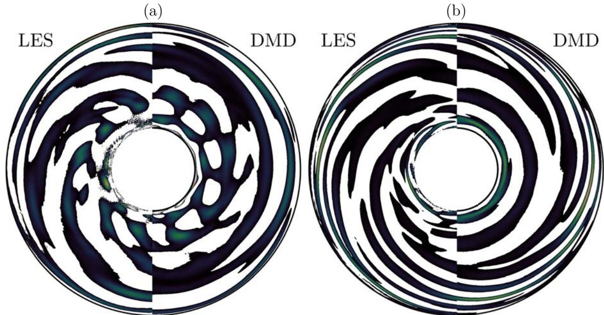
**Figure 3.17** – Isocontours of  $\tilde{u}_z \in [0, 0.05]$  for a composite made of the LES prediction for **Case 3** compared to the combination of the three DMD modes at (a)  $z^* = 0.5$  (mid-cavity) and (b)  $z^* = \delta/h$  (rotor). Values outside the colour range have been blanked out.
