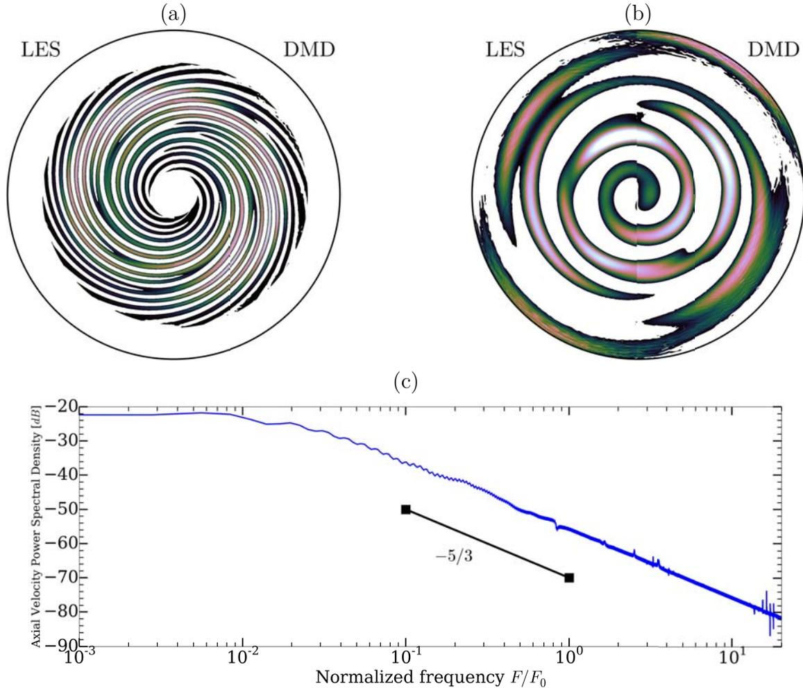
**Figure 3.22** – (a-b) Isocontours of  $\tilde{u}_z \in [0, 0.05]$  for a composite made of the LES prediction for **Case 2** compared to the combination of the DMD mode at (a)  $z^* = 1 - \delta/h$  (stator) and (b)  $z^* = 0.5$  (mid-cavity). Values outside the colour range have been blanked out. (c) Power Spectral Densities (PSD) of the fluctuations of axial velocity in the stationary disc boundary layer of **Case 2** registered by probes  $C_8P_0$ .
