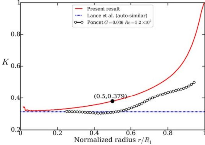
**FIGURE 7.** Radial evolution of the entrainment coefficient  $K$  for the confined flow. Comparison with the auto-similar solution from Lance *et al.* [36] (—) and the results obtained by Poncet [39] for a cavity with  $G = 0.036$  and  $Re_R \simeq 5 \times 10^5$  (○).
