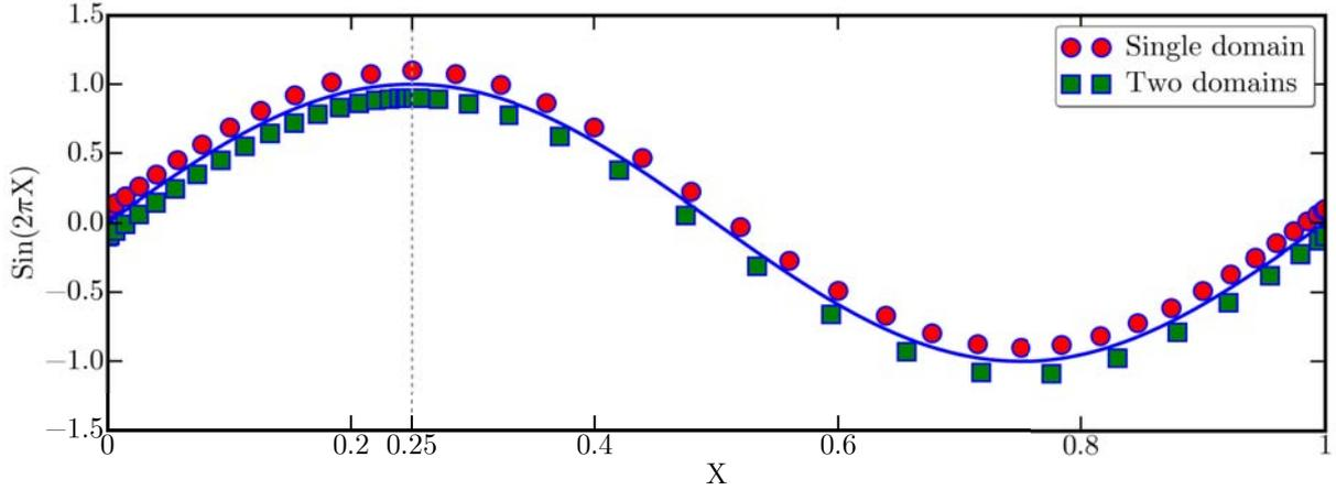
**Figure 2.13** – Influence of the number of sub-domains on the distribution of the mesh points: (red dots) single domain with  $N_{GL} = 40$ , (green squares) two domains with  $z_c = 0.25$  and  $N_{GL,0} = N_{GL,1} = 20$ . In both case, a linear mapping  $f_{in}$  has been used.
