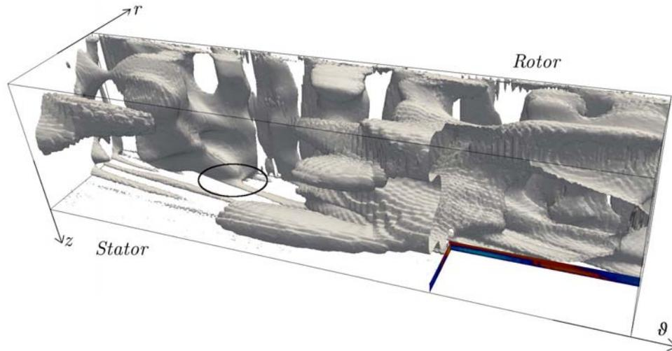
**Figure 3.12** – Isosurface of axial velocity fluctuation  $\tilde{u}_z = 0.02$  in the core of the cavity for **Case 1**. A Cartesian projection has been chosen that spans over the whole radial extent ( $0 \leq r^* \leq 1$ ), the whole axial extent ( $0 \leq z^* \leq 1$ ) and the whole azimuthal extent ( $0 \leq \theta \leq 2\pi$ ) of the cavity.
