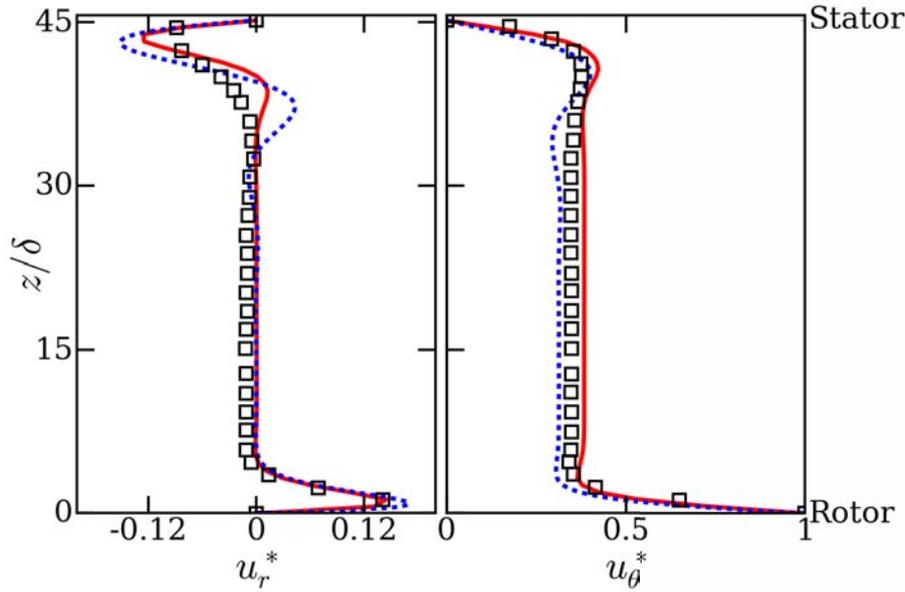
**Figure 3.4** – Axial profiles of the dimensionless mean radial  $u_r^*$  and azimuthal  $u_\theta^*$  velocity components at  $r^* = 0.5$ . Comparison between (–) the LES results, ( $\square$ ) the LDV data by [Séverac et al. \(2007\)](#) and (–) the auto-similar solution by [Rogers & Lance \(1962\)](#).
