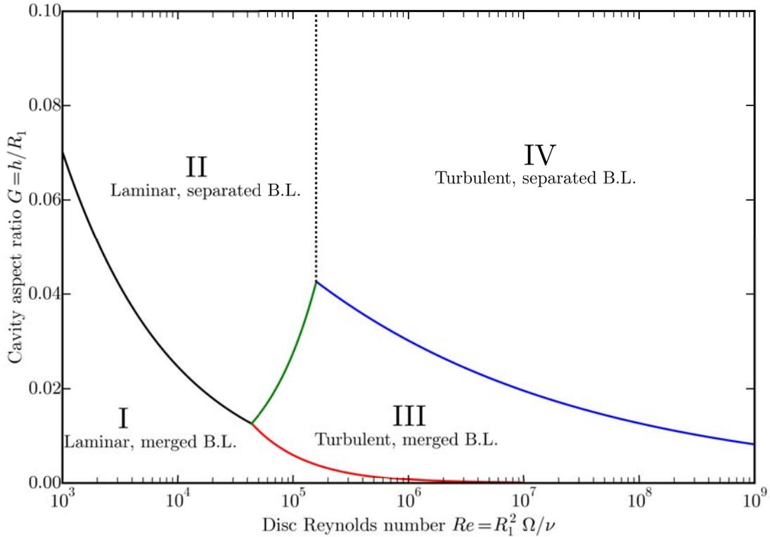
**Figure 2.7** – The four categories of flow encountered in an enclosed rotor/stator cavity, based on an original figure by [Owen & Rogers \(1989\)](#). Regime I is a laminar regime with merged boundary layers whereas regime III is the turbulent pendant. Regimes II and IV describe respectively the laminar and turbulent flows with separated boundary layers.
