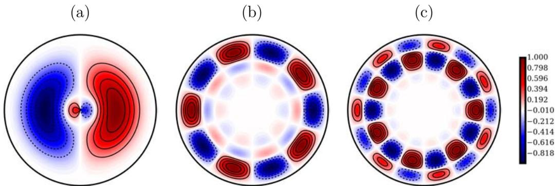
**Figure 2.14** – Fluctuations of radial velocity for the most temporally amplified mode at (a)  $Re = 200$ ,  $m = 1$ ,  $\alpha_r = 1$ , (b)  $Re = 1000$ ,  $m = 5$ ,  $\alpha_r = 1$  and (c)  $Re = 1000$ ,  $m = 7$ ,  $\alpha_r = 1$ .
