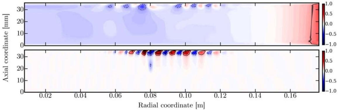
**Figure 3.42** – Fluctuating axial velocity of the global stator mode  $m = 16$  of **Case 2**. Comparison between (*top*) the only mode obtained by DMD (Sec. 3.6) and (*bottom*) the present results with AVLP. Eigenfunctions are clocked at an arbitrary phase angle. The contour lines represent  $w/\max(w) = [-1.0, -0.8, -0.6, -0.4, -0.2, 0.2, 0.4, 0.6, 0.8, 1.0]$ .
