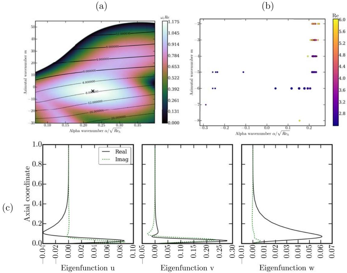
**Figure 3.29** – Results of the temporal stability analysis ( $\alpha_i = 0$ ) in **Case 3**, 'rotor branch'. (a) Amplification rate  $\omega_i Re$  map overlaid with frequency  $-\omega_r Re$  contours at  $Re = 4.48$ . (b) Progression of the most amplified point with the local Reynolds number (marker colour), characterized by the value of the amplification rate (marker size). (c) Example of eigenvector taken at the maximum of amplification.
