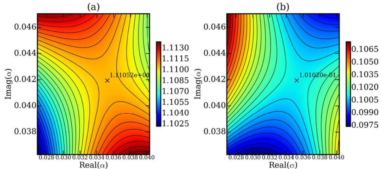
**Figure 3.44** – Isocontours of (a) amplification rate  $\omega_i Re$  and (b) temporal frequency  $-\omega_r Re$  in the  $(\alpha_r/\sqrt{Re_h}, \alpha_i/\sqrt{Re_h})$  plane for the rotor branch of **Case 1** at  $Re = 0.495$ . Zero-contours are represented by a thicker line.
