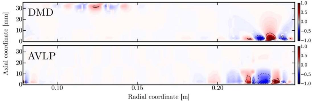
**Figure 3.35** – Fluctuating axial velocity of the global rotor mode  $m = 12$  of **Case 3**. Comparison between (*top*) the mode obtained by DMD and (*bottom*) the present results with AVLP. Eigenfunctions are clocked at an arbitrary phase angle. The contour lines represent  $w/\max(w) = [-1.0, -0.8, -0.6, -0.4, -0.2, 0.2, 0.4, 0.6, 0.8, 1.0]$ .
