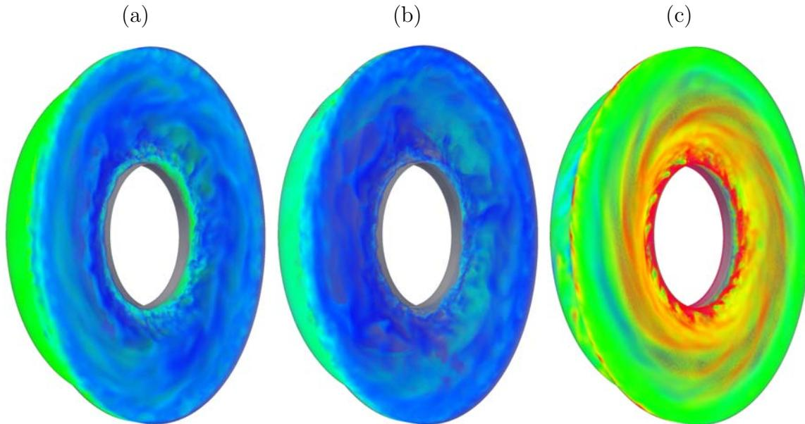
**Figure 4.20** – Isovolumes of  $\text{Species}_1$  mass fraction  $Y_{\text{Species}_1} \in [0.75, 1.0]$  coloured by the static temperature field  $T_s$  in (a) **Case 1**, (b) **Case 2** and (c) **Case 3**. View has been restricted to  $C_1$ . The closest wall (right hand side of each subplot) is the rotor wall.
