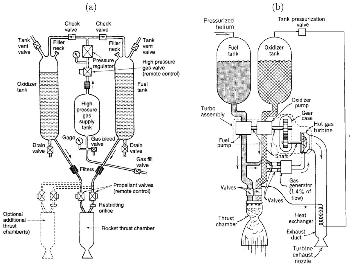
**Figure 1.2** – (a) Schematic flow diagram of a liquid propellant rocket engine with a gas pressure feed system. (b) Simplified schematic diagram of one type of liquid propellant rocket engine with a turbopump feed system and a separate gas generator generating "warm" gas for driving the turbine. Source : [Sutton & Biblarz \(2001\)](#)
