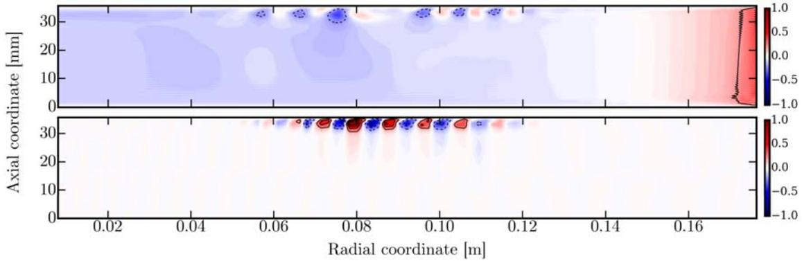
**Figure 3.43** – Fluctuating axial velocity of the global stator mode  $m = 18$  of **Case 2**. Comparison between (*top*) the only mode obtained by DMD (Sec. 3.6) and (*bottom*) the present results with AVLP. Eigenfunctions are clocked at an arbitrary phase angle. The contour lines represent  $w/\max(w) = [-1.0, -0.8, -0.6, -0.4, -0.2, 0.2, 0.4, 0.6, 0.8, 1.0]$ .
