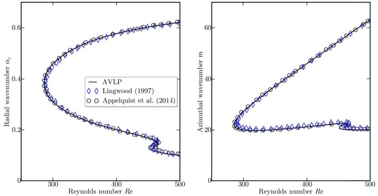
**Figure 2.18** – Neutral curves for stationary disturbance ( $\omega_r = 0$ ,  $\omega_i = 0$ ,  $\alpha_i = 0$ ). Comparison with the works by ( $\diamond$ , diamonds) Lingwood (1997) and ( $\circ$ , circles) Appelquist & Imayama (2014).  $Re$  stands for the local Reynolds number called  $Re_\delta$  in Eqs. (2.2.12)-(2.2.15).
