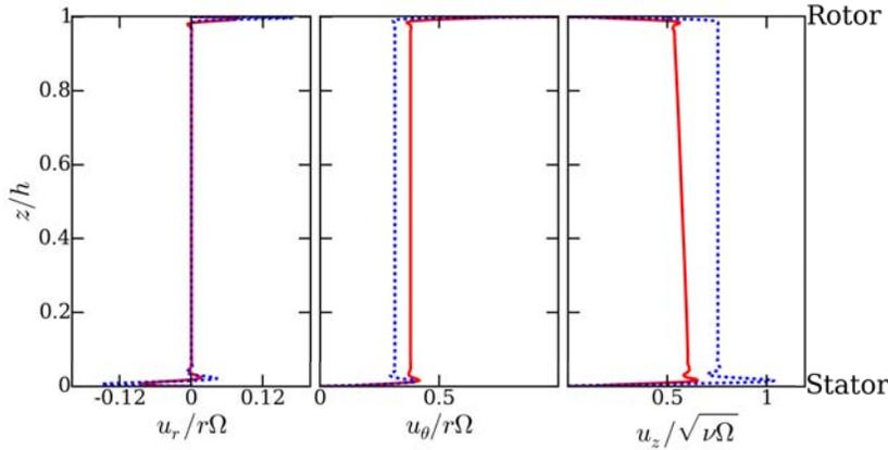
**FIGURE 5.** Axial profiles of the dimensionless time- and theta-averaged ( $N_\theta = 360$ ,  $N_t \Delta t = 100\Omega^{-1}$ ) radial, azimuthal and axial velocity components (from left to right) at mid-radius  $r = 0.5R_1$ . Comparison with the auto-similar solution by Lance *et al.* [36] (—).
