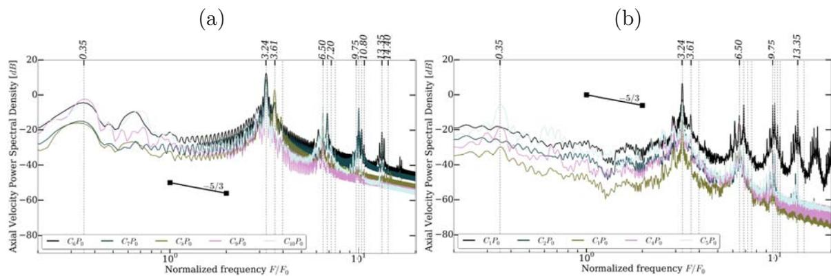
**Figure 3.20** – Power Spectral Densities (PSD) of the fluctuations of axial velocity (a) at mid-height in the cavity registered by probes  $C_{11}P_0$  to  $C_{16}P_0$  and (b) in the rotating disc boundary layer registered by probes  $C_1P_0$  to  $C_5P_0$ . In both cases, innermost probes have the darkest shade of grey, and outermost the lightest.
