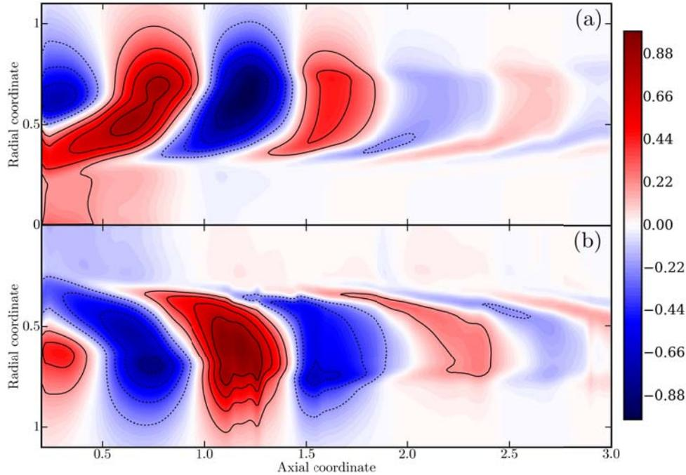
**Figure 2.25** – Fluctuating radial velocity of the mode  $m = 1$  pulsing at 48 Hz. Comparison between (a) the data obtained by Oberleithner (2011) and (b) the present results obtained with AVLP. Eigenfunctions are clocked at an arbitrary phase angle. The contour lines represent  $u/\max(u) = [-1.0, -0.8, -0.6, -0.4, -0.2, 0.2, 0.4, 0.6, 0.8, 1.0]$ .
