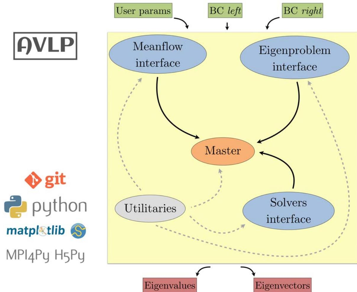
Figure 2.11 – Flowchart of the LNSE solver AVLP
