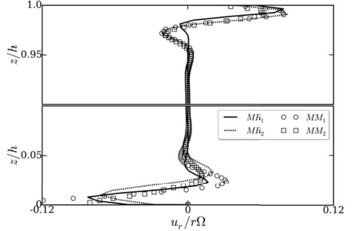
**FIGURE 11.** Axial profiles of the dimensionless time- and theta-averaged ( $N_\theta = 360$ ,  $N_t \Delta t = 100\Omega^{-1}$ ) radial velocity components at mid-radius  $r = 0.5R_1$ . Comparison between the four configurations of Tab. 1. Rotor layer at the top, stator layer at the bottom.
