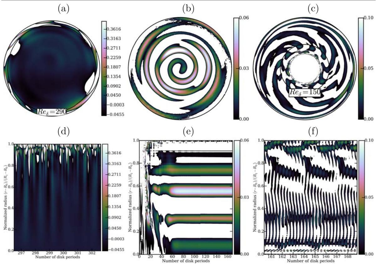
**Figure 3.11** – Snapshots (top) and space-time plots (bottom) of the axial velocity fluctuations  $\tilde{u}_z$  at  $z^* = 0.5$  for (a-d) **Case 1**, (b-e) **Case 2** and (c-f) **Case 3** respectively. Labels indicate radial positions of interest and/or the radial extent of the patterns. Bold circles without labels mark the limits of the computational domain.
