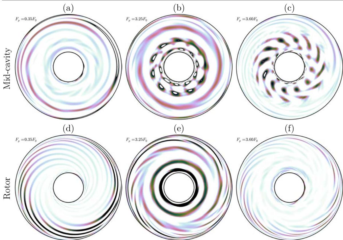
**Figure 3.16** – Isocontours of  $\tilde{u}_z \in [0, 0.05]$  at  $(a, b, c)$   $z^* = 0.5$  (mid-cavity) and  $(d, e, f)$   $z^* = \delta/h$  (rotor) for the three major DMD modes constituting **Case 3** sorted out by their respective frequencies. Values outside the colour range have been blanked out.
