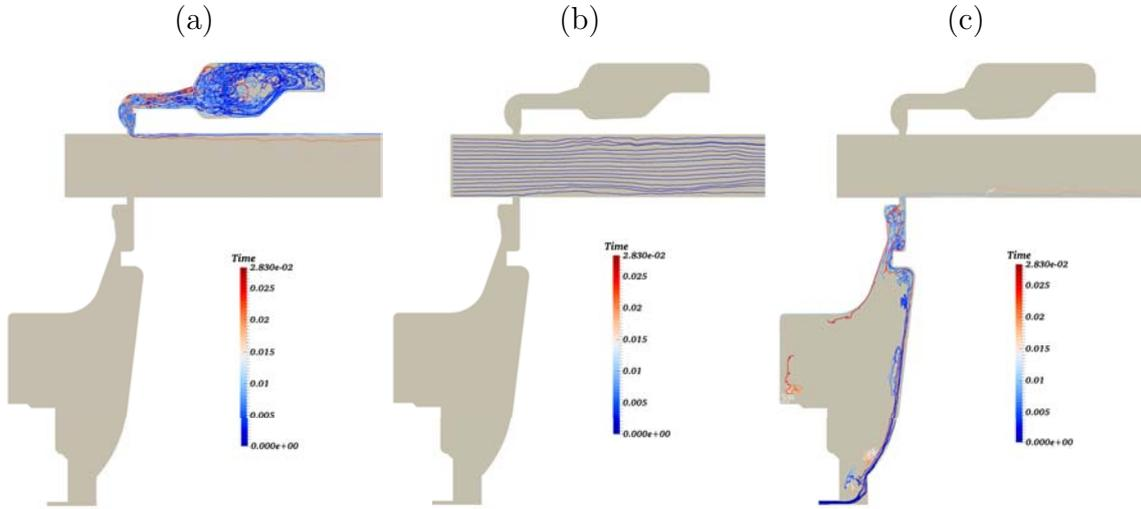
**Figure 4.19** – Projection upon an  $(r, z)$  plane of pathlines obtained with solutions from Case 3, seeded (a) in  $C_5$ , (b) close to the inlet  $I_2$  of the channel  $C_2$  and (c) close to the inlet  $I_1$  of the rotor/stator cavity  $C_1$ . Colormap is identical in all three subplots and represents the age of the fluid particles in seconds.
