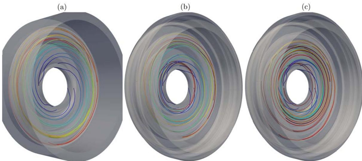
**Figure 4.11** – Streamlines seeded at  $r = 0.26$  and  $r = 0.30$  for (a) **Case 1**, (b) **Case 2** and (c) **Case 3**, integrated over 5 periods. The tubes are coloured by the age of the fluid particle.
