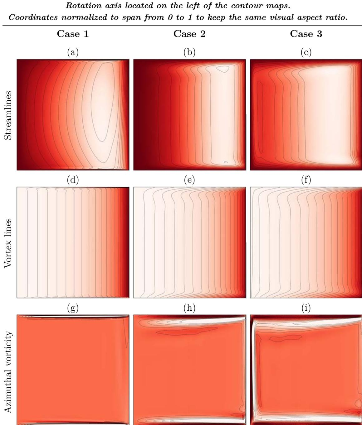
**Figure 3.6** – Contours of (top) streamlines, (middle) vortex lines and (bottom) azimuthal vorticity for (left) **Case 1**, (centre) **Case 2** and (right) **Case 3**. Streamlines are in the range  $\psi \in [-1.0 \times 10^{-5}, 0]$  for **Case 1** and  $\psi \in [-2.0 \times 10^{-3}, 0]$  for **Case 2** & **3**. For all cases, vortex lines span (quadratically)  $r^{*2}u_{\theta}^* \in [0, 1]$  and vorticity  $\eta_{\theta} \in [-1, 1]$ .
