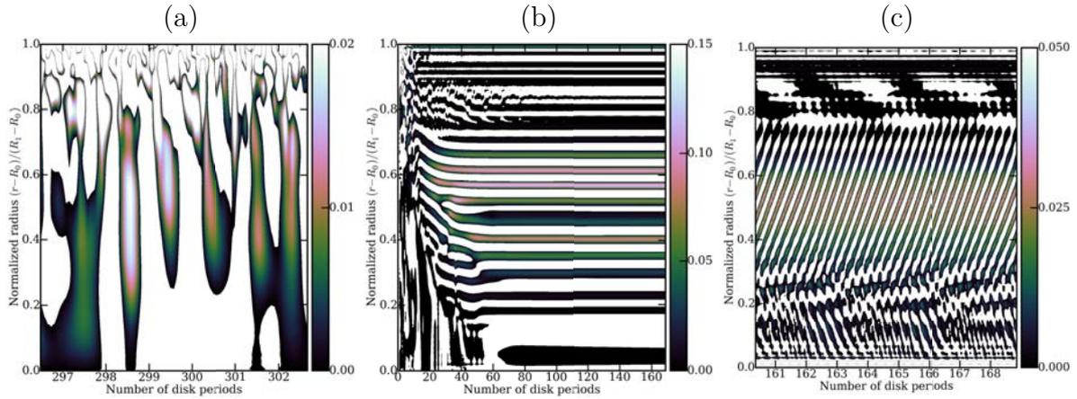
**Figure 3.9** – Space-time plots of  $\tilde{u}_z$  at  $z^* \simeq 1 - \delta/h$ ,  $\theta = 0$  with  $r^* \in [0, 1]$  for (a) **Case 1**, (b) **Case 2** and (c) **Case 3**. Time range has been zoomed as needed to capture the right precession frequency. Values outside of the colour range have been blanked out.
