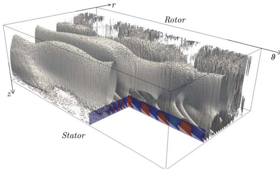
**Figure 3.13** – Isosurface of axial velocity fluctuation  $\tilde{u}_z = 8 \times 10^{-3}$  in the core of the cavity for **Case 2**. A Cartesian projection has been chosen that spans over the whole radial extent ( $0 \leq r^* \leq 1$ ), the whole axial extent ( $0 \leq z^* \leq 1$ ) and the whole azimuthal extent ( $0 \leq \theta \leq 2\pi$ ) of the cavity.
