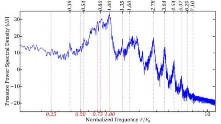
**FIGURE 4.** Temporal power spectral density of the pressure fluctuations (1) registered at the pointwise probe PB<sub>3</sub> (see Fig. 1(b)) plotted against the normalized frequency. Constituent frequencies from the experiments (dot-dashed lines) and from the LES (dashed lines) are also presented.
