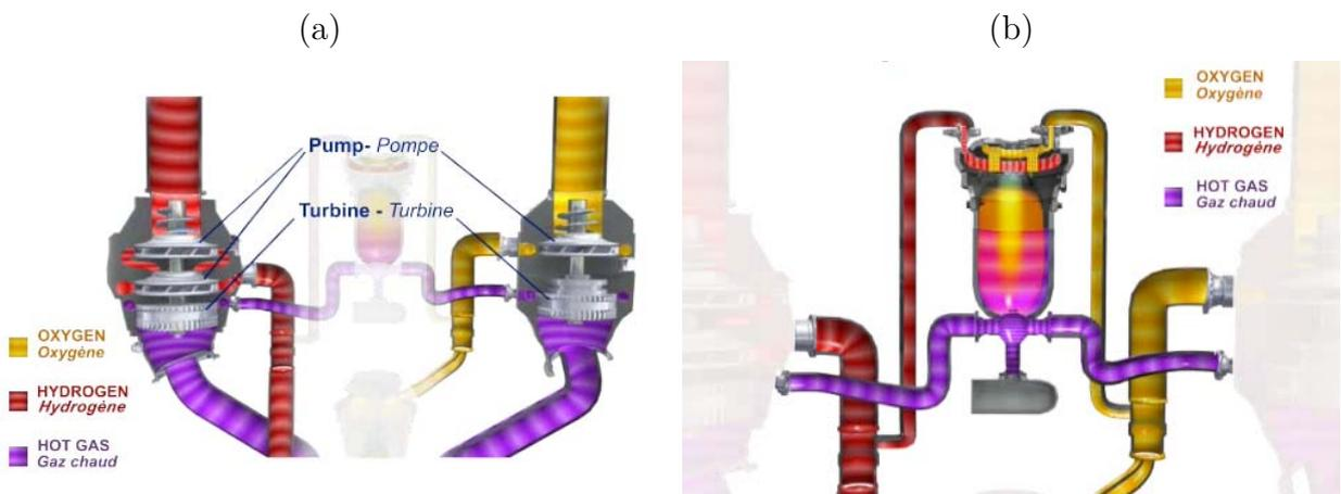
**Figure 1.3** – (a) Representation of the two turbopumps used in the Vulcain 2 engine and their gas generator. (b) Detail of the gas generator feeding both turbopumps of the Vulcain 2 engine. Source : [How Do Our Engines Work ?](#), Safran Snecma
