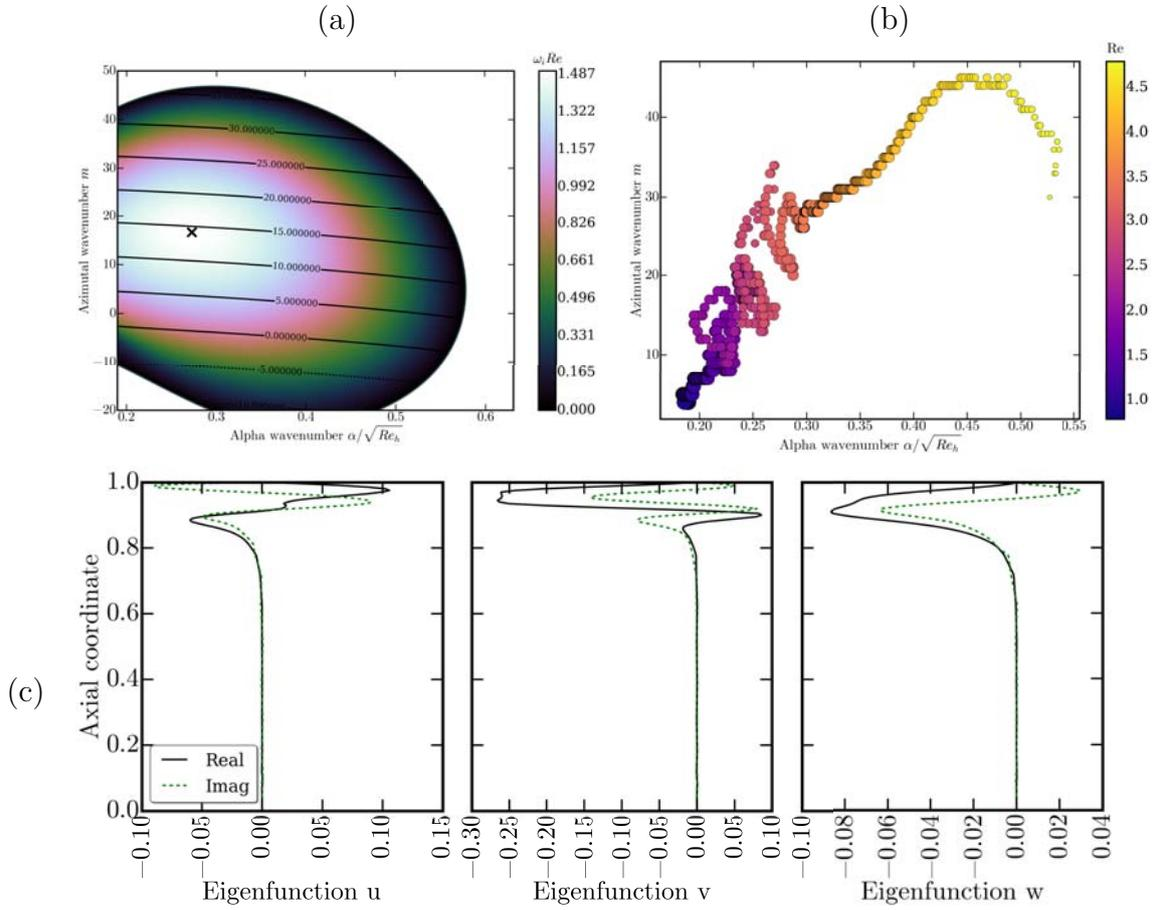
**Figure 3.27** – Results of the temporal stability analysis ( $\alpha_i = 0$ ) in **Case 2**, 'stator branch'. (a) Amplification rate  $\omega_i Re$  map overlaid with frequency  $-\omega_r Re$  contours at  $Re = 2.94$ . (b) Progression of the most amplified point with the local Reynolds number (marker colour), characterized by the value of the amplification rate (marker size). (c) Example of eigenvector taken at the maximum of amplification.
