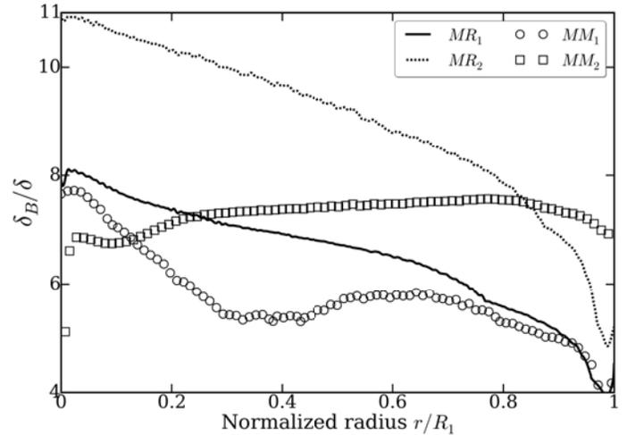
**FIGURE 12.** Radial distributions of the Bödewadt boundary layer thickness, non-dimensionalized by the factor  $\delta = \sqrt{\nu/\Omega}$ , plotted against the dimensionless radius  $r/R_1$ . Comparison between the four cases discussed in this document (see Tab. 1).
