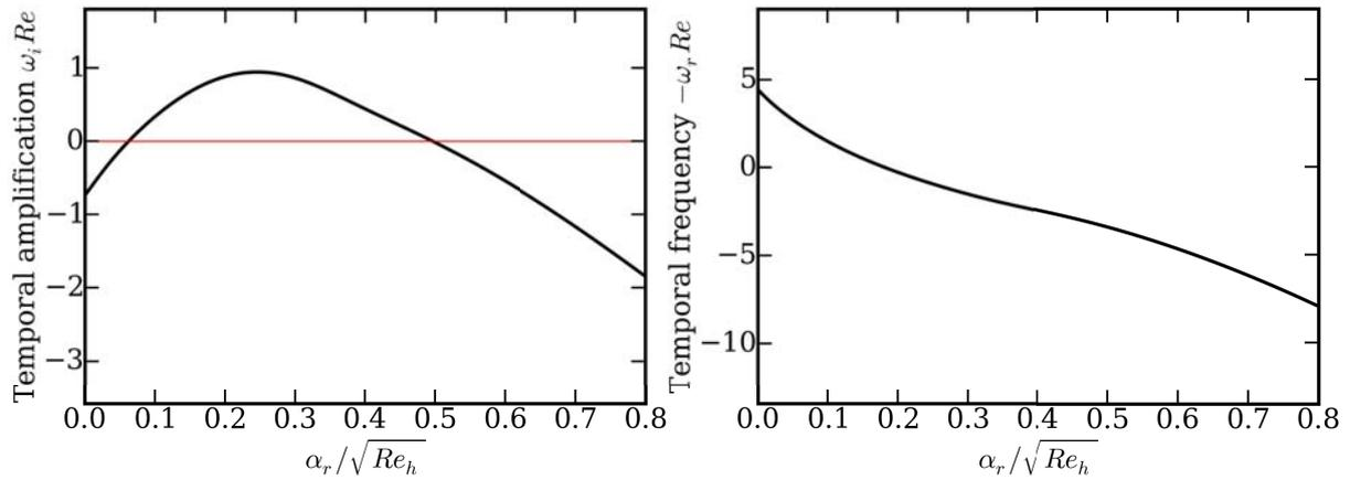
**Figure 3.31** – Evolution of (left) the temporal amplification rate  $\omega_i Re$  and (right) temporal frequency  $-\omega_r Re$  with the radial wavenumber  $\alpha_r/\sqrt{Re_h}$  at  $m = 12$  for the rotor branch of **Case 3** at  $Re = 4.48$ . Zero amplification is marked by an horizontal line.
