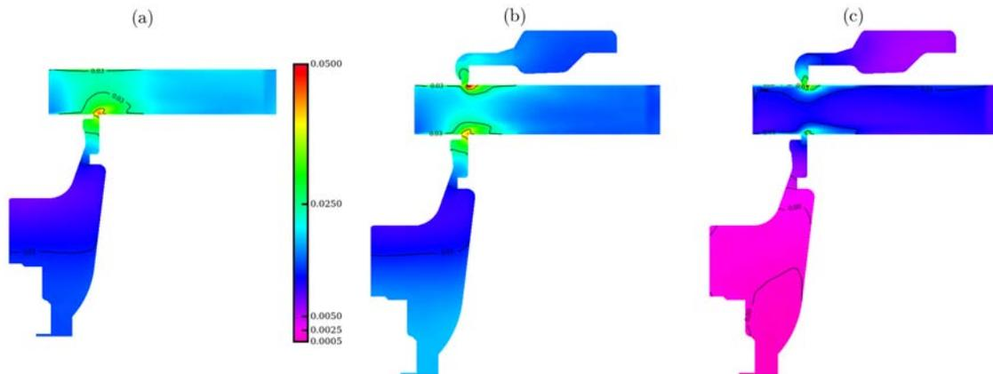
**Figure 4.17** – Contours of the static pressure RMS  $P_s^{\text{RMS}}$  for (a) **Case 1**, (b) **Case 2** and (c) **Case 3**. The range indicated in (a) is valid in all three cases.
