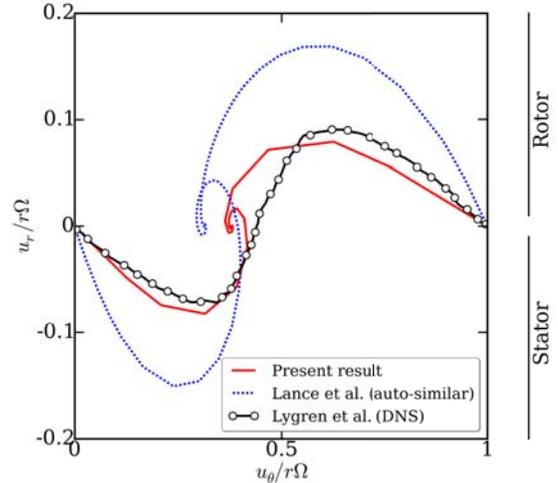
**FIGURE 6.** Polar plot of the dimensionless time- and theta-averaged ( $N_\theta = 360$ ,  $N_t \Delta t = 100\Omega^{-1}$ ) velocity distribution at mid-radius  $r = 0.5R_1$ . Comparison between (—) the LES results, (---) the auto-similar solution by Lance *et al.* [36] and (o-o) the DNS results of Lygren and Andersson [9].
