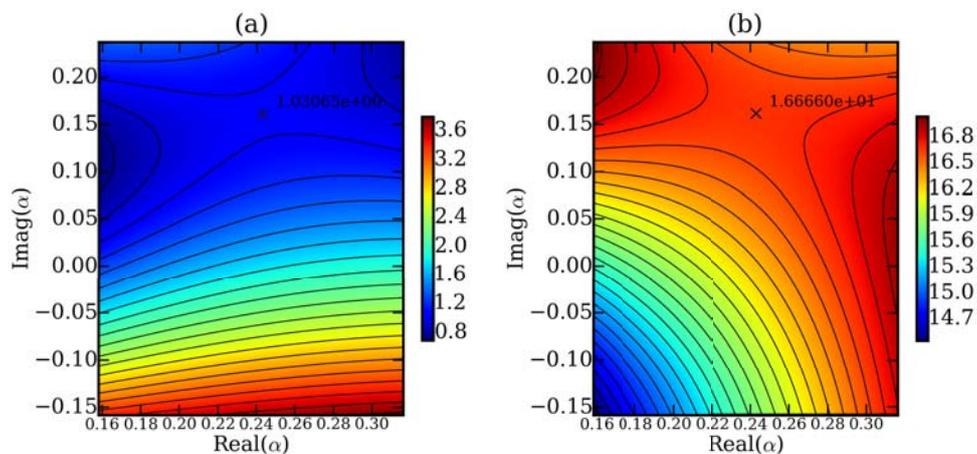
**Figure 3.40** – Isocontours of (a) amplification rate  $\omega_i Re$  and (b) temporal frequency  $-\omega_r Re$  in the  $(\alpha_r/\sqrt{Re_h}, \alpha_i/\sqrt{Re_h})$  plane for the rotor branch of **Case 2** at  $Re = 3.92$  and  $m = 18$ .
