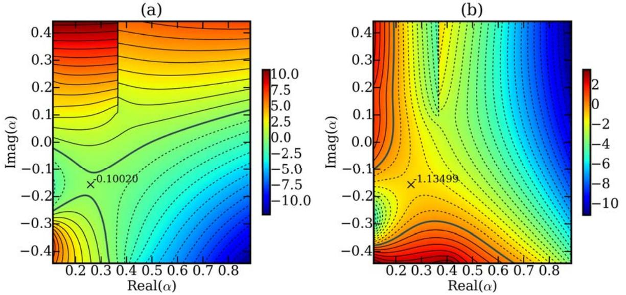
**Figure 3.32** – Isocontours of (a) amplification rate  $\omega_i Re$  and (b) temporal frequency  $-\omega_r Re$  in the  $(\alpha_r/\sqrt{Re_h}, \alpha_i/\sqrt{Re_h})$  plane for the rotor branch of **Case 3** at  $Re = 4.48$ . Zero-contours are represented by a thicker line.
