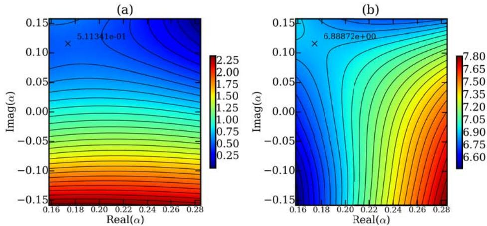
**Figure 3.38** – Isocontours of (a) amplification rate  $\omega_i Re$  and (b) temporal frequency  $-\omega_r Re$  in the  $(\alpha_r/\sqrt{Re_h}, \alpha_i/\sqrt{Re_h})$  plane for the rotor branch of **Case 2** at  $Re = 1.96$  and  $m = 7$ .
