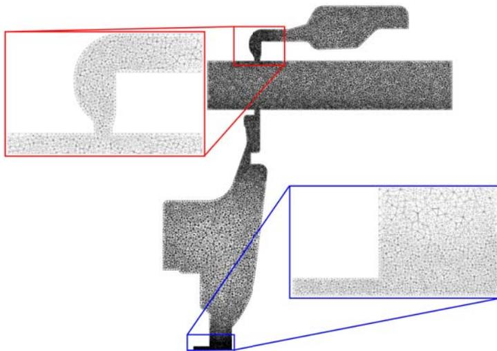
**Figure 4.2** –  $(r,z)$ -cut of the three-dimensional mesh used for **Case 1**, **Case 2** & **Case 3**, supplemented with insets showing the areas of refinement: (top, red)  $C_2$ - $C_5$  pass, (bottom, blue) inlet  $I_1$ .
