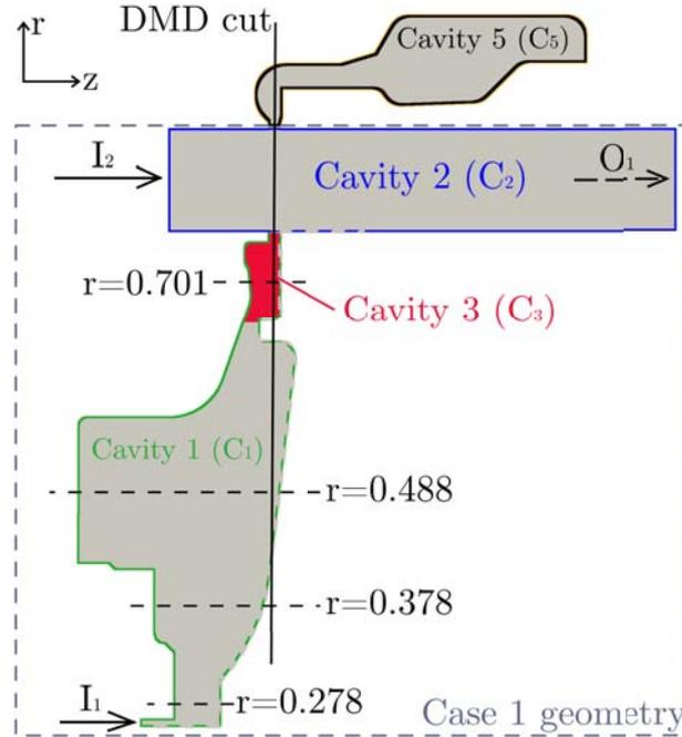
**Figure 4.1** –  $(r,z)$ -cut of the axisymmetric geometry used for **Case 1** (without  $C_5$ ) and **Case 2 & 3** marked with relevant notations pertaining to the names of the cavities, the inlets & outlets, the location of the rotor, four radial stations of special interest and the trace of the  $(r,\theta)$ -cut used for the DMD algorithm (see Sec. 4.4.2.b).
