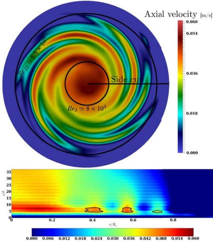
**FIGURE 9.** Top:  $(r/R_1, \theta, z/h = 0.025)$  slice (stator) colored by  $u_z$  with relevant notations. Bottom:  $(r/R_1, 0, 0.0 \leq z/h \leq 0.1)$  slice colored by axial velocity  $u_z$  and selected contours  $u_z = [0.02, 0.04]$ .
