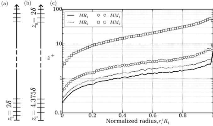
**FIGURE 10.** (a) Schematic structure of the mesh for MR<sub>2</sub> and MM<sub>1</sub>. (b) Schematic structure of the mesh for MM<sub>2</sub>. (c) Radial evolution of the wall normal coordinate  $z^+$  near the stator for all four cases (see Tab. 1).
