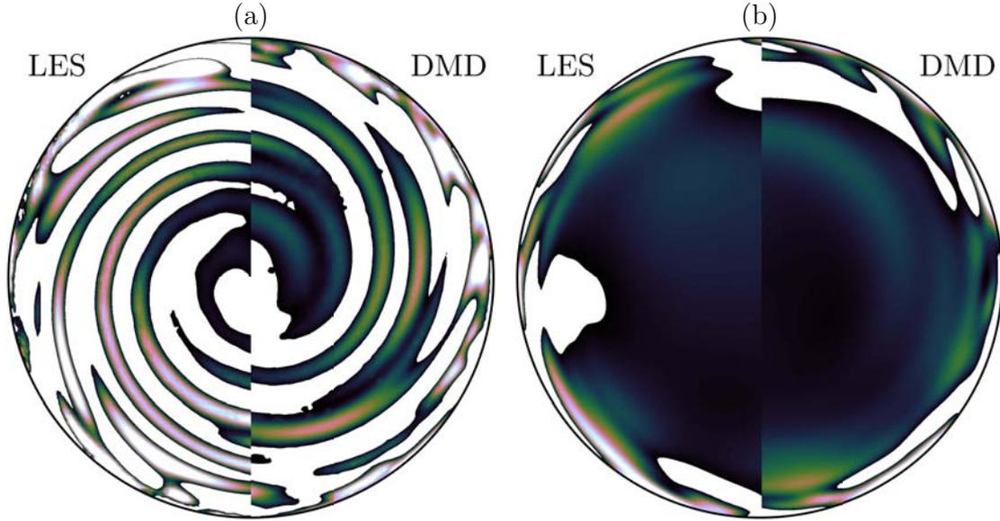
**Figure 3.23** – Isocontours of  $\tilde{u}_z \in [0, 0.05]$  for a composite made of the LES prediction for **Case 1** compared to the combination of the eleven DMD modes at (a)  $z^* = 1 - \delta/h$  (stator) and (b)  $z^* = 0.5$  (mid-cavity). Values outside the colour range have been blanked out.
