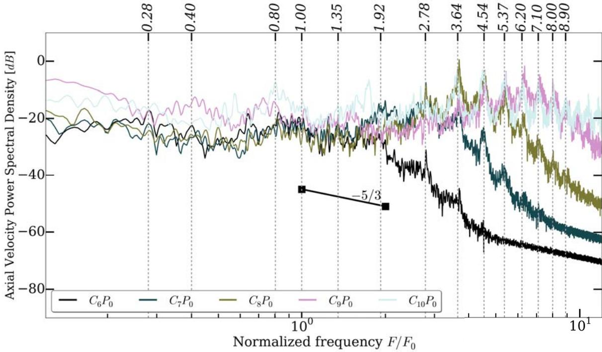
**Figure 3.24** – Power Spectral Densities (PSD) of the fluctuations of axial velocity in the stationary disc boundary layer of **Case 1** registered by probes  $C_6P_0$  to  $C_{10}P_0$  (darkest to lightest shade, respectively).
