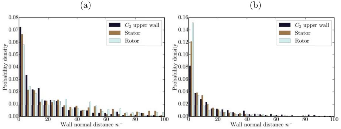
**Figure 4.4** – Density probability of normal wall coordinate  $n^+$  predicted by the LES of (a) **Case 2** and (b) **Case 3**. The repartition over  $C_2$  upper wall (left black), the stator wall (middle brown) and the rotor wall (right light blue) have been separated from each other.
