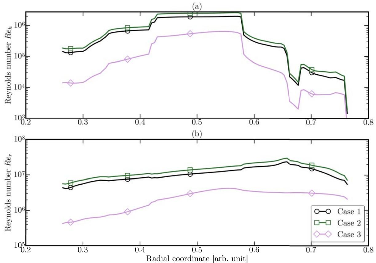
**Figure 4.8** – Evolution with the dimensionless radial coordinate of (a) the axial Reynolds number  $Re_h = h^2\Omega/\hat{\nu}$  and (b) the radial Reynolds number  $Re_r = r^2\Omega/\hat{\nu}$ . The four locations of extraction  $r_1$ ,  $r_2$ ,  $r_3$  and  $r_4$  are marked by symbols and the viscosity is defined by  $\hat{\nu}(r) = \int_{z_{\min}}^{z_{\max}} \nu(r, \xi) d\xi$
