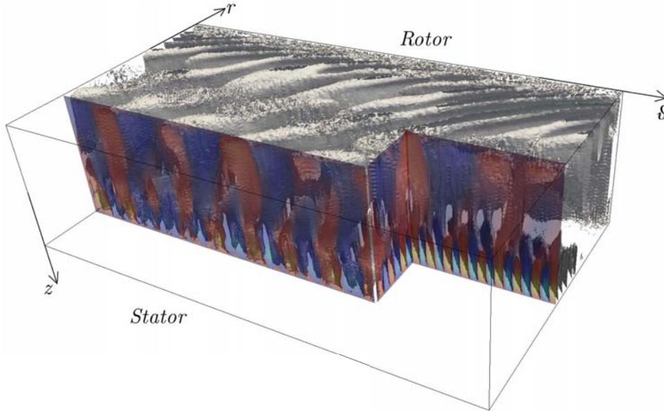
**Figure 3.14** – Isosurface of axial velocity fluctuation  $\tilde{u}_z = 0.01$  in the core of the cavity for **Case 3**. A Cartesian projection has been chosen that spans over the whole radial extent ( $0 \leq r^* \leq 1$ ), the whole axial extent ( $0 \leq z^* \leq 1$ ) and the whole azimuthal extent ( $0 \leq \theta \leq 2\pi$ ) of the cavity.
