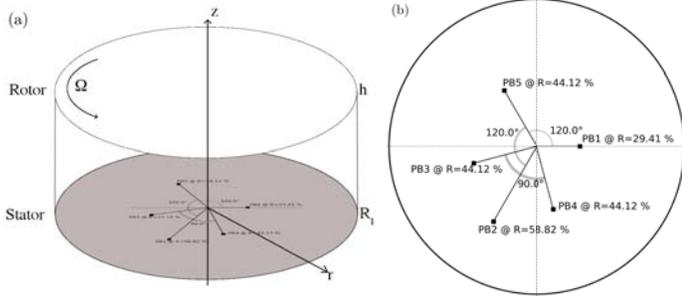
**FIGURE 1.** (a) Schematic representation of the rotating cavity with relevant notations: radius  $R_1$ , height  $h$  and rotation speed  $\Omega$ . (b) Detail of the five probes used in the experimental configuration.
