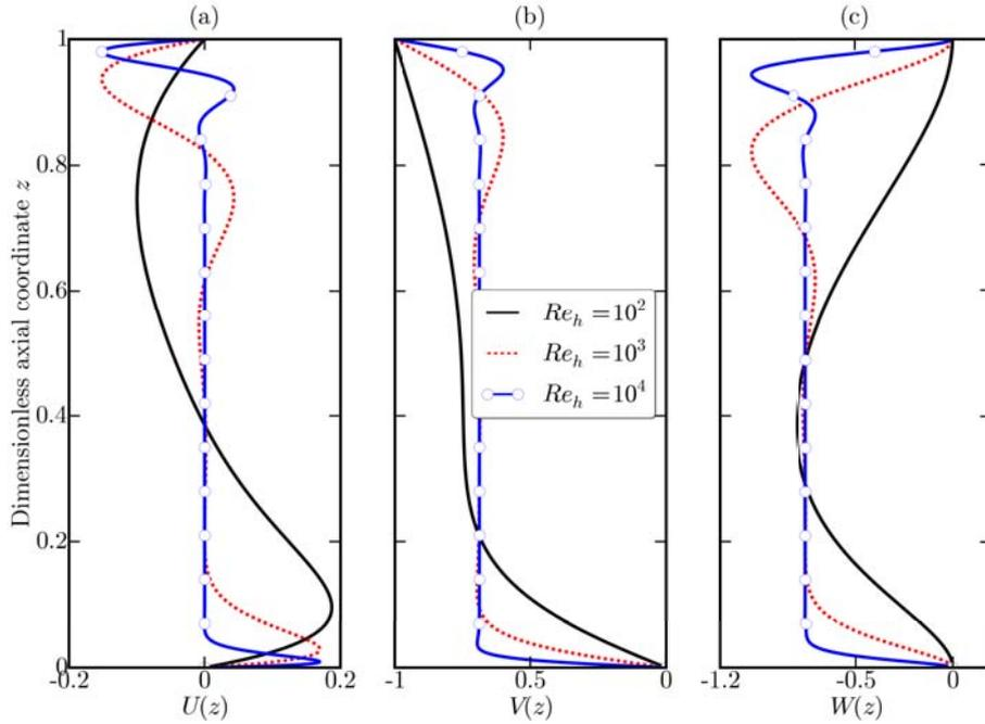
**Figure 2.6** – Auto-similar velocity profiles of the laminar flow between a rotor and a stator for different interdisc Reynolds numbers  $Re_h$ : (a) Radial velocity,  $U$ , (b) azimuthal velocity,  $V$  and (c) axial velocity,  $W$ , components.
