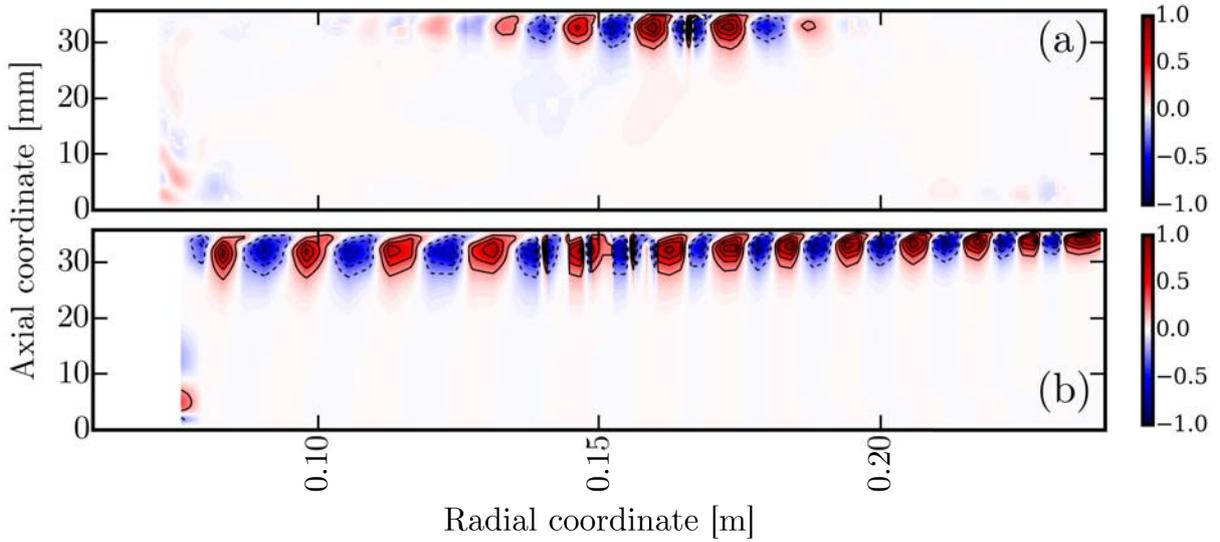
**Figure 3.30** – Fluctuations of axial velocity  $w$ , normalized by their  $\infty$ -norm, in **Case 3**. (a) Strongest DMD mode in the stator boundary layer organizing as a 29-armed spiral confined in  $r \in [0.110, 0.2]$  (see Sec. 3.6.1.a). (b) LSA stator mode reconstructed by selecting at each location the eigenvector and  $(\alpha_r, m)$  pair corresponding to the greatest temporal amplification rate (see Fig. 3.28).
