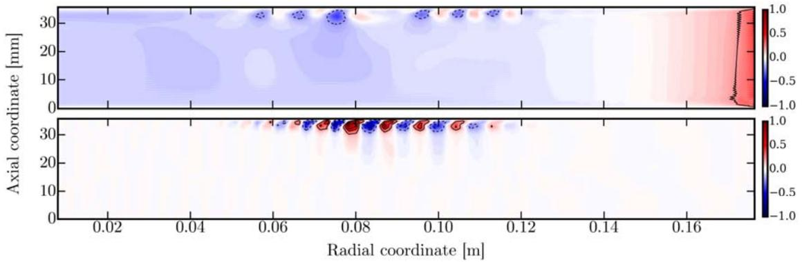
**Figure 3.41** – Fluctuating axial velocity of the global stator mode  $m = 7$  of **Case 2**. Comparison between (*top*) the only mode obtained by DMD (Sec. 3.6) and (*bottom*) the present results with AVLP. Eigenfunctions are clocked at an arbitrary phase angle. The contour lines represent  $w/\max(w) = [-1.0, -0.8, -0.6, -0.4, -0.2, 0.2, 0.4, 0.6, 0.8, 1.0]$ .
