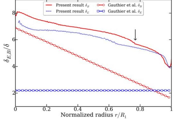
**FIGURE 8.** Radial distributions of the boundary layer thicknesses, non-dimensionalized by the factor  $\delta = \sqrt{\nu/\Omega}$ , plotted against the dimensionless radius  $r/R_1$ . Both the stationary disc  $\delta_B$  and the rotating disc  $\delta_E$  boundary layers are presented. Comparison with the experimental results of Gauthier *et al.* [34].
