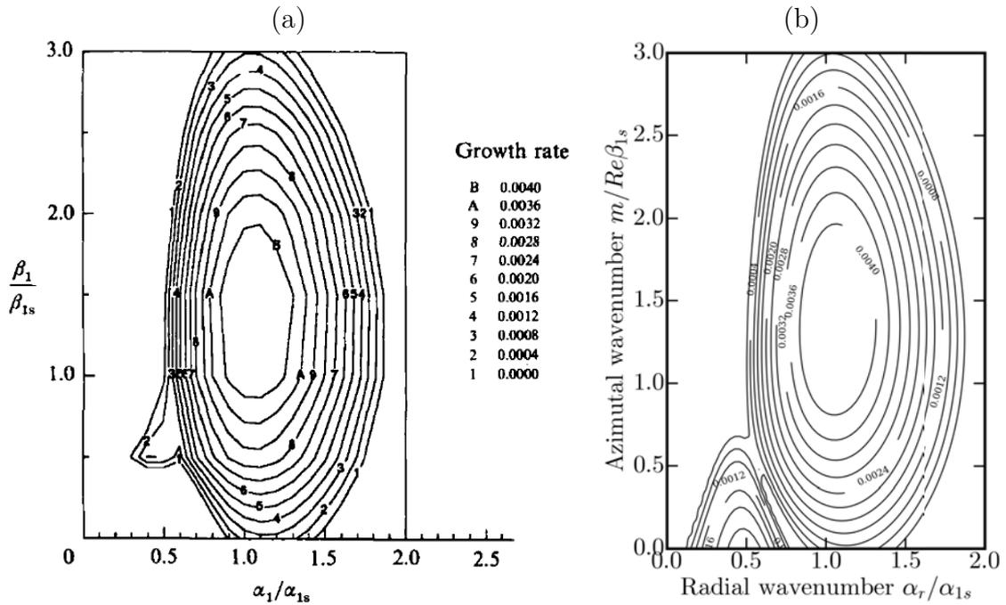
**Figure 2.16** – Contour plot of amplification rate in the wavenumber  $(\alpha_r, m)$ -plane for  $Re_\delta = 450$  - comparison between (a) Balachandar *et al.* (1992) results and (b) AVLP results. Here the radial and azimuthal wavenumbers are normalized by  $\alpha_{1s} = 0.328$  and  $Re_\delta \beta_{1s} = 31.455$ .
