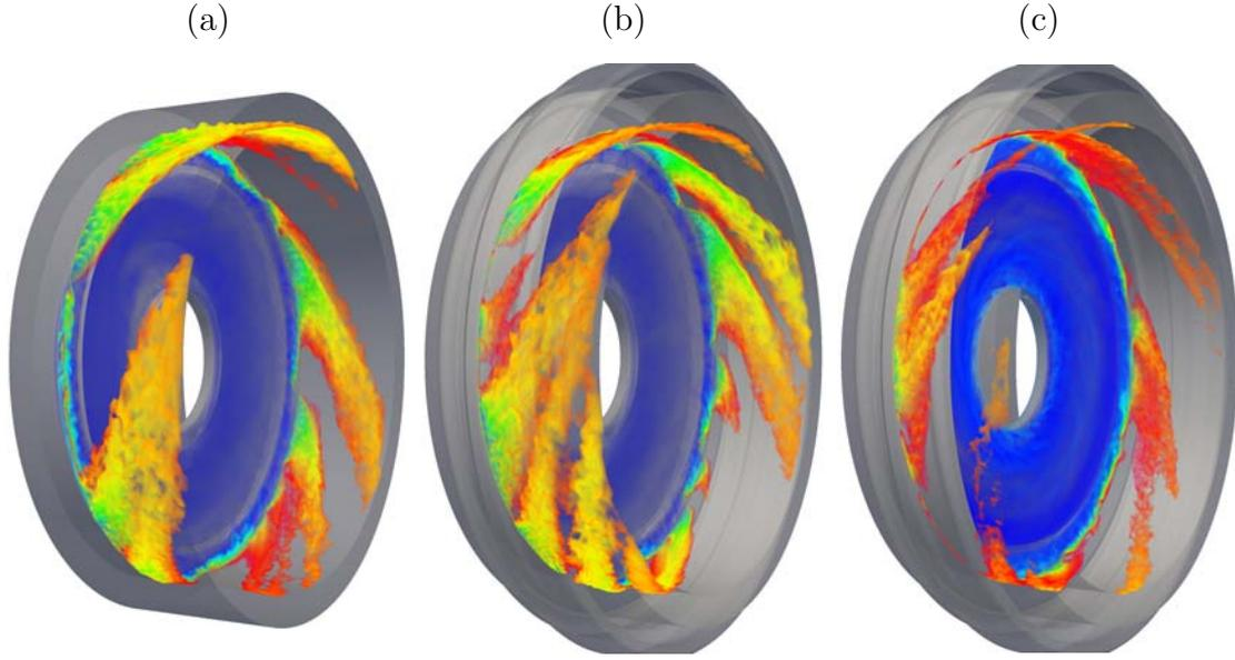
**Figure 4.21** – Isovolumes of Species<sub>1</sub> mass fraction  $Y_{\text{Species}_1}$  coloured by the static temperature field  $T_s$  in (a) **Case 1** for  $Y_{\text{Species}_1} \in [0.5, 1.0]$ , (b) **Case 2** for  $Y_{\text{Species}_1} \in [0.5, 1.0]$  and (c) **Case 3** for  $Y_{\text{Species}_1} \in [0.48, 1.0]$ . The whole geometry is shown, orientation is similar to that in Fig. 4.20.
