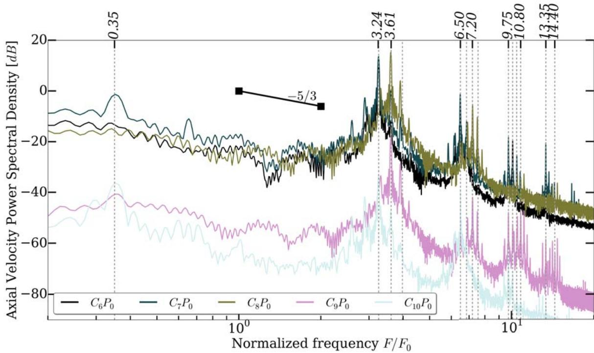
**Figure 3.19** – Power Spectral Densities (PSD) of the fluctuations of axial velocity in the stationary disc boundary layer of **Case 3** registered by probes  $C_6P_0$  to  $C_{10}P_0$  (darkest to lightest shade, respectively).
