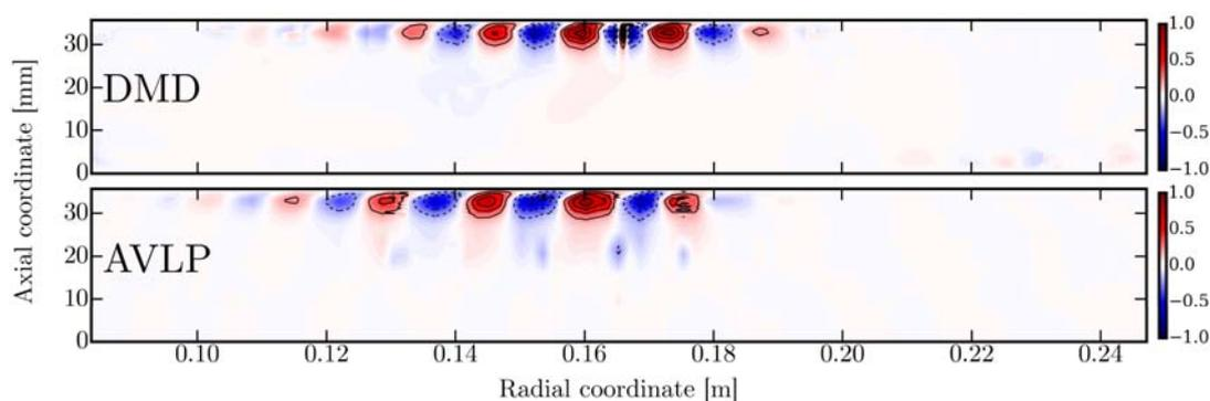
**Figure 3.37** – Fluctuating axial velocity of the global stator mode  $m = 29$  of **Case 3**. Comparison between (top) the mode obtained by DMD and (bottom) the present results with AVLP. Eigenfunctions are clocked at an arbitrary phase angle. The contour lines represent  $w/\max(w) = [-1.0, -0.8, -0.6, -0.4, -0.2, 0.2, 0.4, 0.6, 0.8, 1.0]$ .
