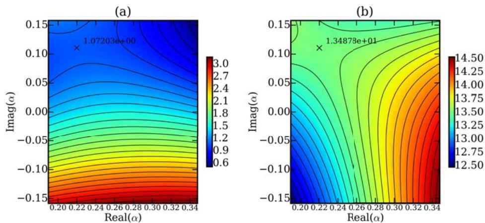
**Figure 3.39** – Isocontours of (a) amplification rate  $\omega_i Re$  and (b) temporal frequency  $-\omega_r Re$  in the  $(\alpha_r/\sqrt{Re_h}, \alpha_i/\sqrt{Re_h})$  plane for the rotor branch of **Case 2** at  $Re = 2.94$  and  $m = 16$ .
