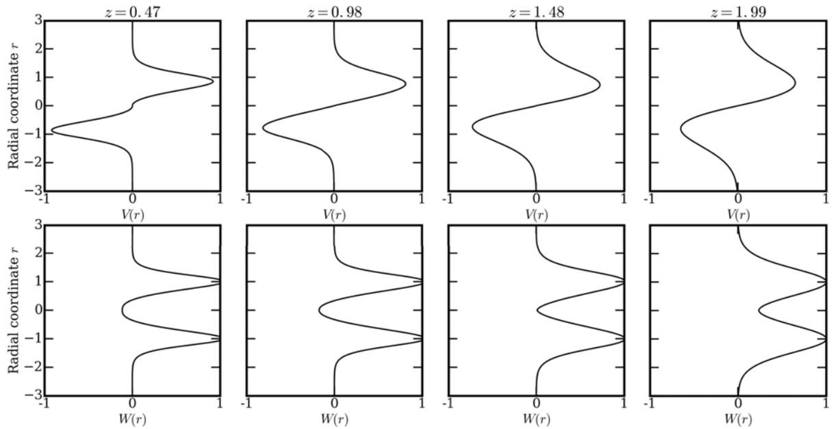
**Figure 2.22** – Azimuthal velocity (*top*) and axial velocity (*bottom*) profiles taken at four distinct dimensionless axial locations  $z = 0.47$ ,  $z = 0.98$ ,  $z = 1.48$  and  $z = 1.99$  as a function of the dimensional radial coordinate  $r$ . Profiles generated with the set of equations Eq. (2.2.51) and parameters from [Oberleithner \(2011\)](#).
