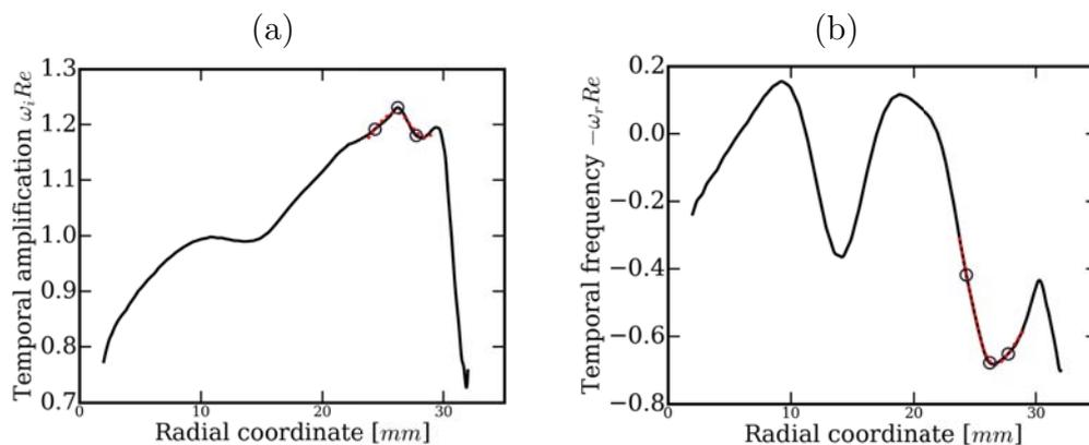
**Figure 3.45** – Radial evolution of (a) the growth rate and (b) the temporal frequency of the stator branch of **Case 1** with the fitted Padé polynomial in the region of interest (dashed line) and the position of the saddle points of  $\tilde{\omega}_0(r \in \mathbb{C})$ .
