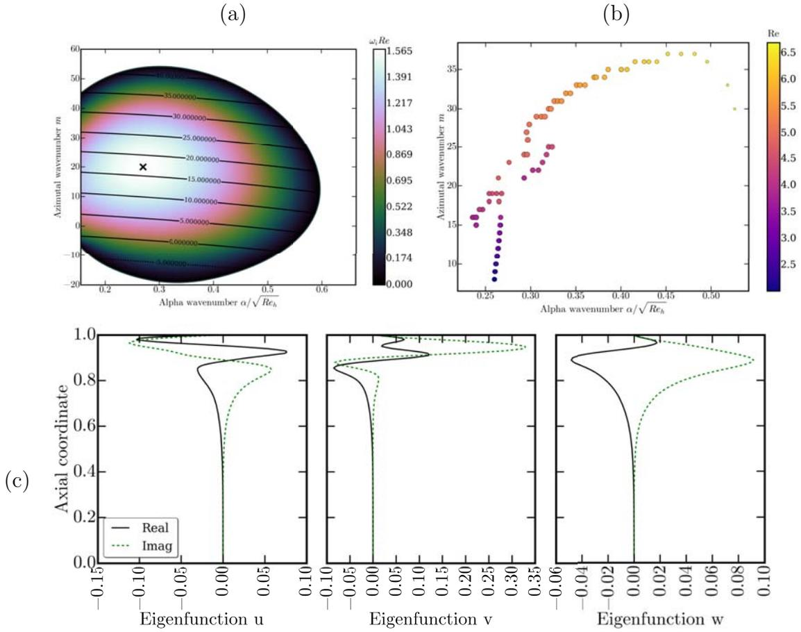
**Figure 3.28** – Results of the temporal stability analysis ( $\alpha_i = 0$ ) in **Case 3**, ‘stator branch’. (a) Amplification rate  $\omega_i Re$  map overlaid with frequency  $-\omega_r Re$  contours at  $Re = 4.48$ . (b) Progression of the most amplified point with the local Reynolds number (marker colour), characterized by the value of the amplification rate (marker size). (c) Example of eigenvector taken at the maximum of amplification.
