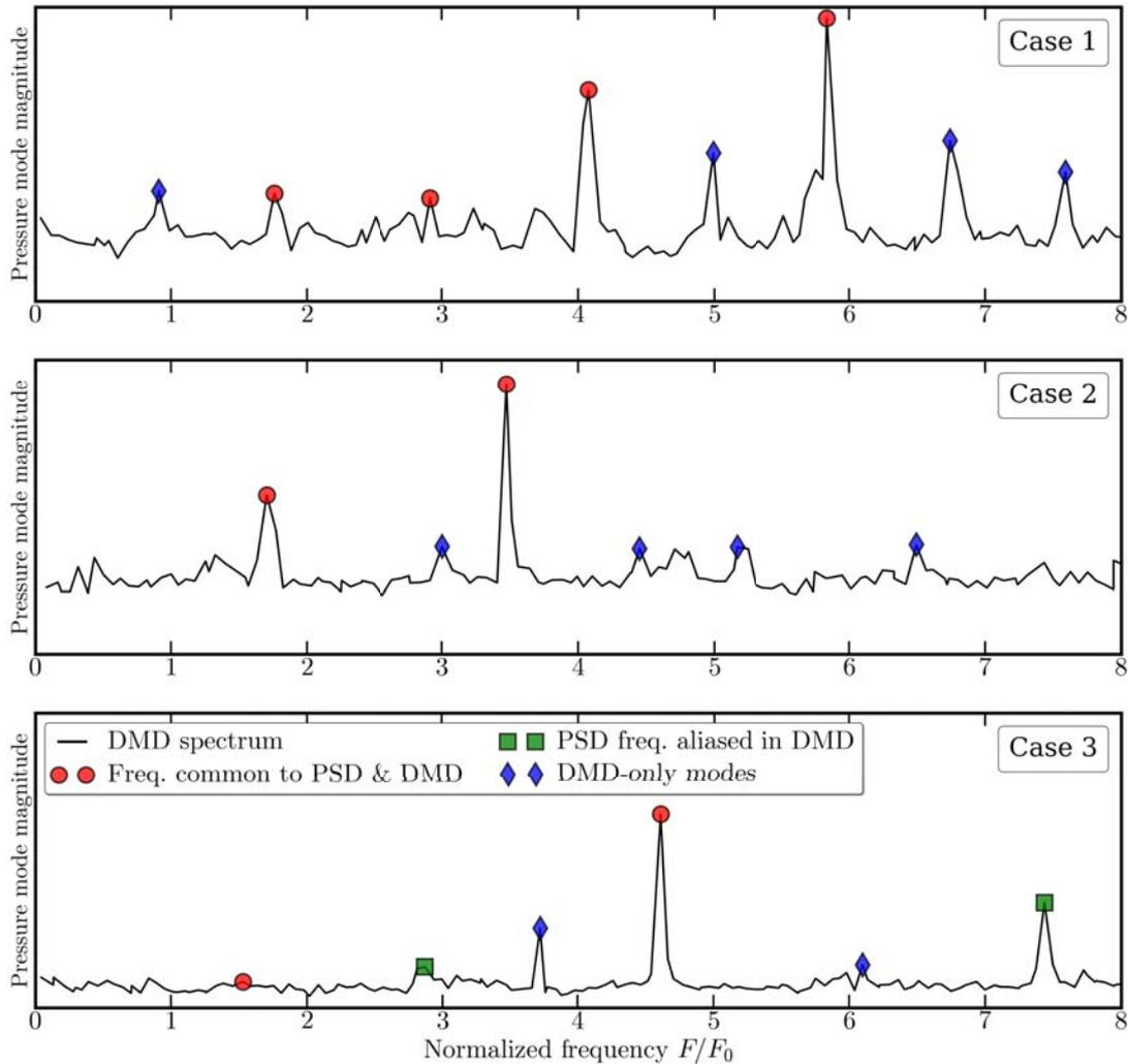
**Figure 4.27** – DMD spectrum for (top) **Case 1**, (middle) **Case 2** and (bottom) **Case 3**, obtained with instantaneous snapshots sampled at  $\Delta t_{\text{DMD}} = 0.06$  period for a time  $t_{\text{DMD}} = 17$  periods. PSD frequencies are indicated with dots. Aliased PSD frequencies are indicated with squares. Extra modes only given by the DMD are indicated with diamonds.
