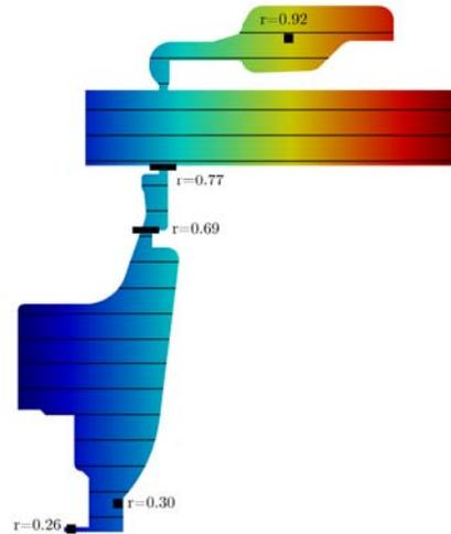
**Figure 4.10** – Locations of the seeds for the streamlines computations. (■) Single particle is tracked from that location. (■) 10 particles are seeded at the corresponding radial location. All seeding locations are duplicated at azimuths  $\theta = 0, \pi/2, \pi, 3\pi/2$ .
