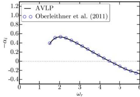
**Figure 2.24** – Spatial amplification rate of the mode  $m = 1$  versus dimensionless  $\omega_r$  at  $z = 0.5$ . Comparison between ( $\circ$ ) the data obtained by Oberleithner (2011) and (-) the present results with AVLP.
