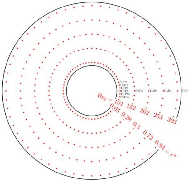
**Figure 3.18** – Locations of the numerical probes in the cavity associated with **Case 3**. The bottom disc, the homogeneous core and the top disc have been instrumented with 300 probes arranged on 5 circles of 60 probes. Numbering example matches that of the rotor layer.
