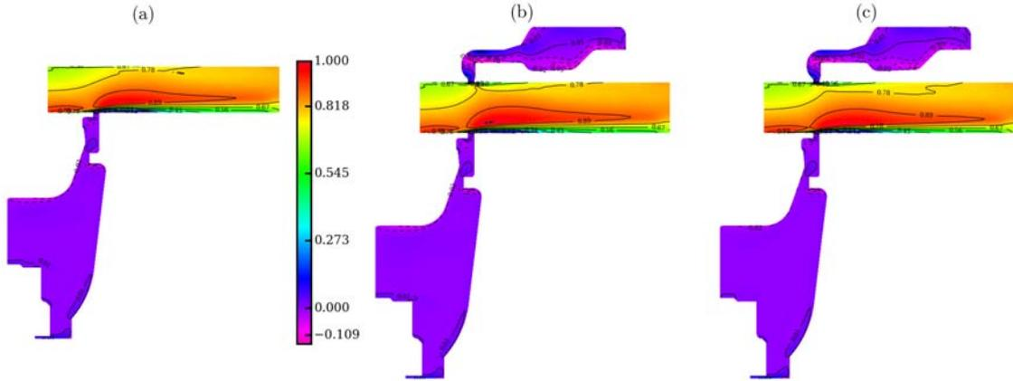
**Figure 4.18** – Contours of the averaged axial velocity  $\bar{u}$  for (a) **Case 1**, (b) **Case 2** and (c) **Case 3**. The velocity is expressed in m/s and the range indicated in (a) is valid in all three cases.
