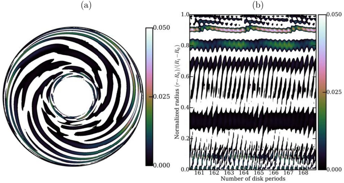
**Figure 3.10** – (a) Snapshot and (b) space-time plot of the axial velocity fluctuations  $\tilde{u}_z$  in the rotating disc boundary layer at  $z^* \simeq \delta/h$  for **Case 3**. Values outside the colour ranges have been blanked out.
