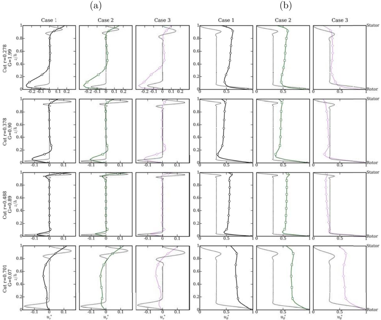
**Figure 4.9** – Axial profiles of the dimensionless mean (a) radial  $u_r^*$  and (b) azimuthal  $u_\theta^*$  velocity components extracted at the locations indicated on Fig. 4.8a. Comparison between (symbols) the LES results and (- -) the auto-similar laminar solution from Rogers & Lance (1962) at the ad-hoc axial Reynolds number (see Fig. 4.8b-top).
