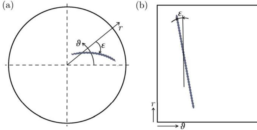
**Figure 3.7** – Definition of the angle  $\varepsilon$  between a spiral arm (bold grey dash-outlined streak) and the normal to the geostrophic flow in (a) polar view and (b) equivalent Cartesian coordinates.
