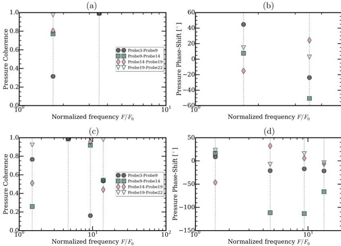
**Figure 4.26** – Coherence (a, c) and phase-shift (b, d) of the wavefronts at the constituent frequencies spotted in (a, b) **Case 2** and (c, d) **Case 3**. Four pairs of probes have been considered to characterize the modal organization throughout the geometry.
