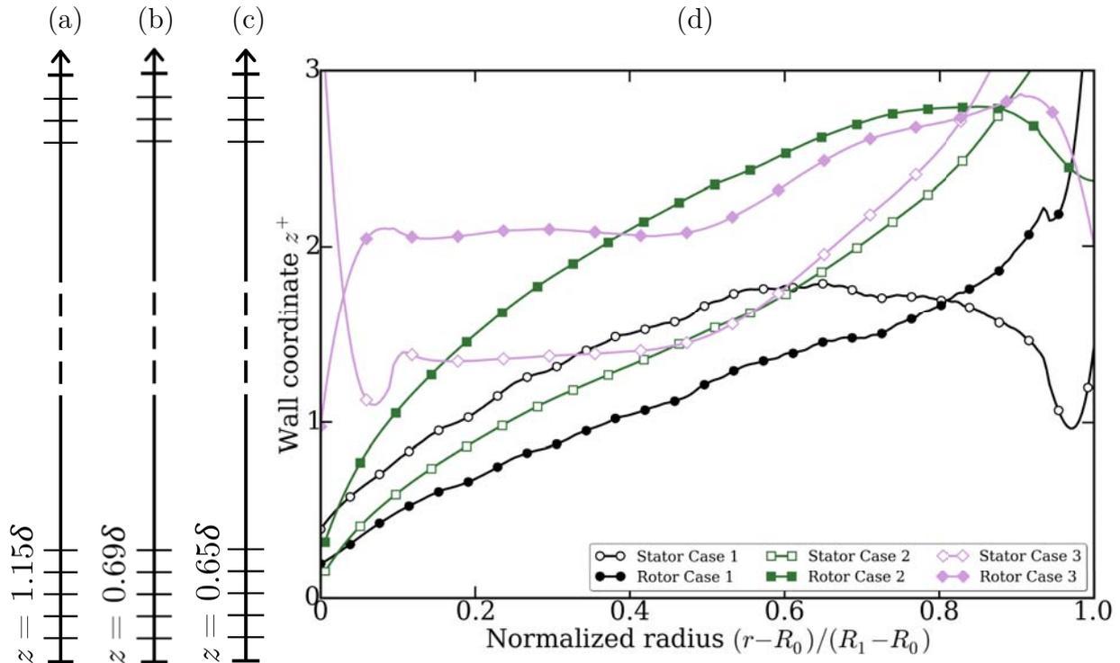
**Figure 3.3** – (a)-(b)-(c) Schematic structures of the wall-resolved LES meshes for **Case 1**, **Case 2** and **Case 3** respectively. (d) Radial evolution of the wall coordinate  $z^+$  near the rotors (filled symbols) and the stators (open symbols) for **Case 1** (circles), **Case 2** (squares) and **Case 3** (diamonds). Note that symbols do not indicate mesh nodes.
