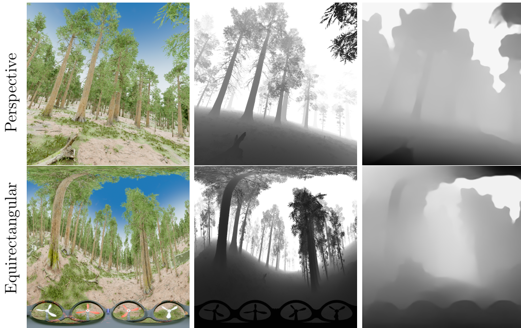
Figure 6.9: RДФOREST: (left to right: RGB, ground truth depth, and estimated depth with baseline MIDAS network [60]).
