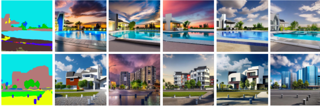
Figure 7.3: Controlling Stable Diffusion with ADE20K [58] segmentation map [159]. On the left is the control semantic segmentation control input used to create the different landscape images on the right.
