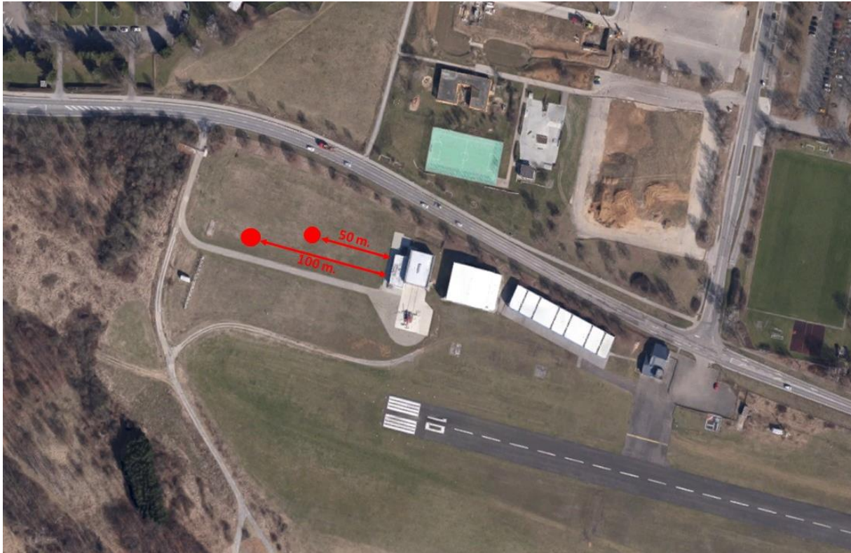
Figure 22 – Antenna positions for data collection at Pattonville airport
