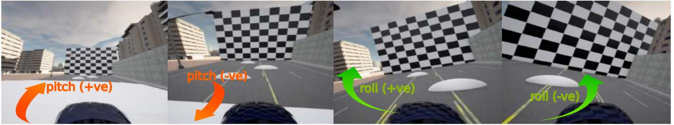
Figure 2.3: Excitation of the vehicle pitch and roll angles using bubble bumps for reliable calibration results using Kalibr.
