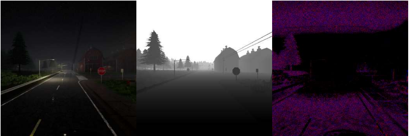
Figure 1.2: A simulated challenging driving scenario with high intensity fog, rain and darkness as seen from left to right by: RGB camera, Depth sensor, and Event camera (source: IBISCape [1]).
