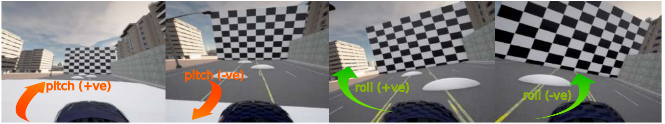
Figure 2.3: Excitation of the vehicle pitch and roll angles using bubble bumps for reliable calibration results using Kalibr.
