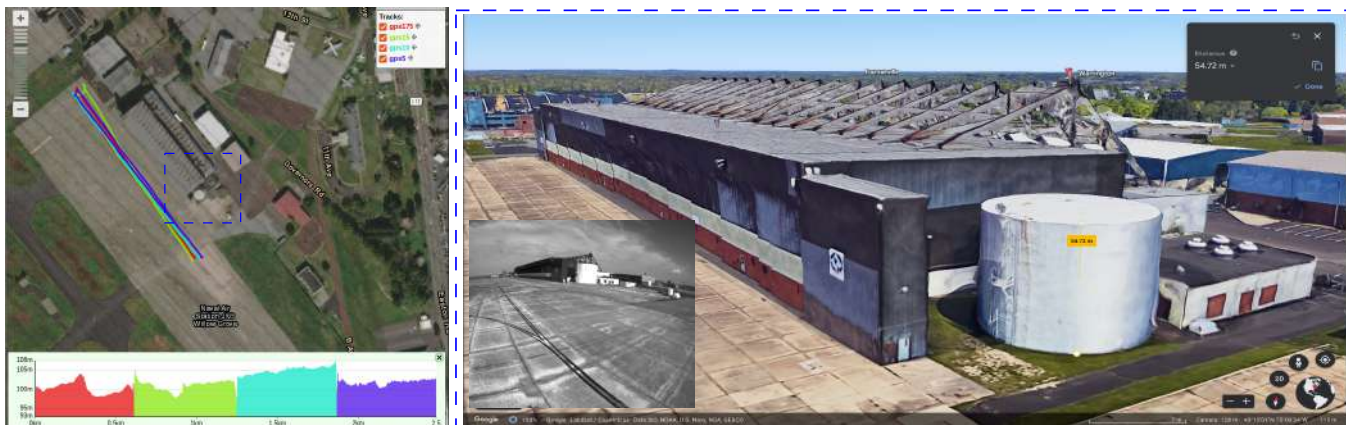
Figure 4.1: An example for the on-map GPS readings of the large-scale environment of the Fast Flight dataset [124] sequences: gps175 , gps15 , gps10 , and gps5 . The sequence number denotes the maximum flight velocity of each sequence: 17.5, 15, 10, and 5 [m/sec], respectively. The color bar (bottom) denotes the map scale in [km] on the x-axis and the altitude of each sequence in [m] on the y-axis. In the blue dotted box: Comparing the maximum MAV's altitude at instance before the descent stage to the height of an aircraft hangar. The estimated airport asset height is 54.72 [m], corresponding to the maximum MAV altitude. Images are courtesy of Google Earth.
