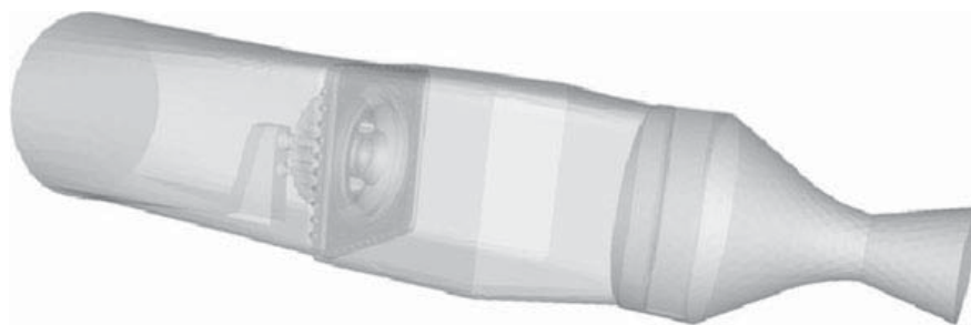
Fig. 9 Computational domain for the multipoint injection burner
