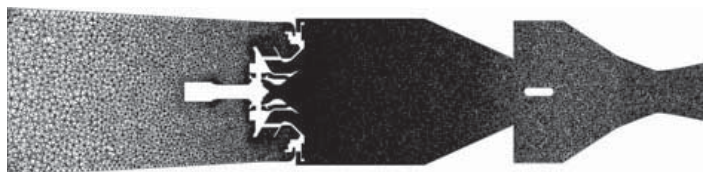
Fig. 11 Vertical mid-plane cut of the mesh used for the multipoint injection configuration
