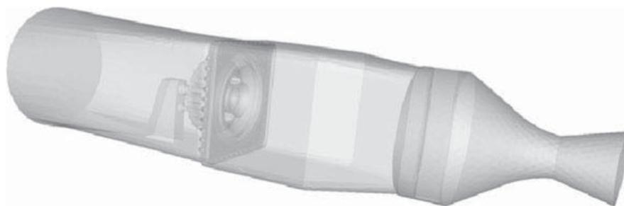
**Fig. 9** Computational domain for the multipoint injection burner
