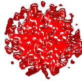
(a) Spotted texture of a pointed laser beam.
