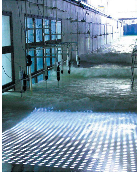
FIGURE 4.1 – Grid of light dot patterns projected onto the swash zone in the CIEM large-scale wave flume at the UPC (Barcelona).
