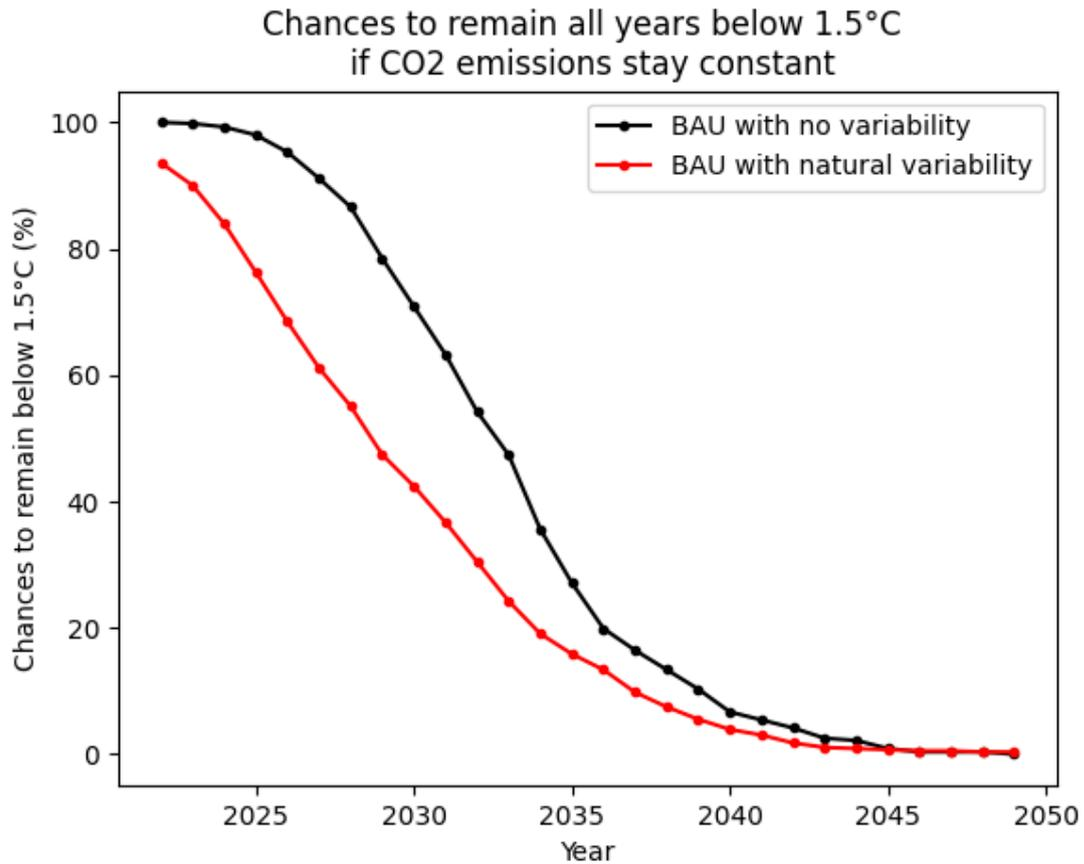
**Supplementary Figure 2** Chances of remaining below 1.5°C if CO<sub>2</sub> emissions remain at current 2022 levels and if non-CO<sub>2</sub> RF follows a scenario in the middle range of the C6-C7 ensemble<sup>16</sup> from AR6 (corresponding to a combination of current policies and moderate actions). Black line indicates the results obtained without considering natural variability. Red line shows those including natural variability.
