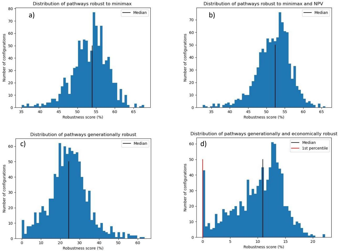
*Figure 5 Distribution of the robustness score for near-optimal pathways robust to minimax (panel a), minimax and NPV (panel b),  $NPV_{Diff}$  (panel c), and  $NPV_{Diff}$ , NPV and minimax (panel d). The black line gives the median value of these distributions. In panel d., the red line gives the 1<sup>st</sup> percentile of the configuration with the least economically and generationally robust pathways.*
