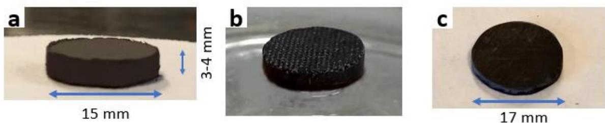
Figure-3.2.4: a - \text{Bi}_2\text{Te}_3 Buckypaper; b - \text{Bi}_2\text{Te}_3 /epoxy resin after curing (before polishing); c - CNT/epoxy resin composite after polishing
