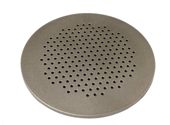
Figure 6.13: Photograph of the filter relative to the second prototype iodine tank.
