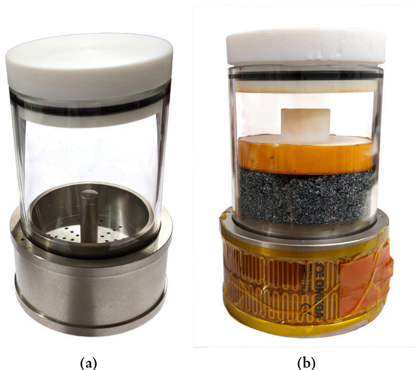
Figure 6.7: First prototype iodine tank (a) at first assembly and (b) after iodine loading.
