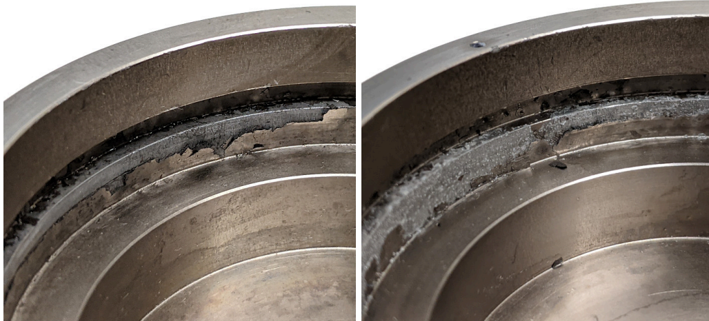
(a) Sublimation cup right after disassembly (b) Sublimation cup after a few days at room conditions.
