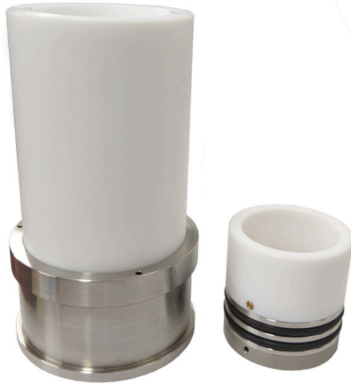
Figure 6.12: Photograph of the second prototype iodine tank, (left) main body and (right) upper piston.
