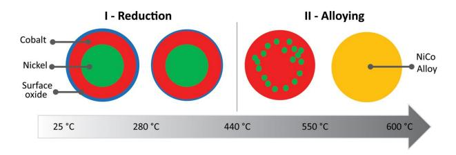
**Figure 2.** Evolution of the Ni-Co core-shell nanoparticles during heating under vacuum. Reproduced from <sup>44</sup>.
