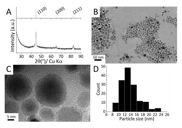
**Figure 1**. Crystalline bcc-Fe nanoparticles synthesized by adapting the method reported by L.-M. Lacroix *et al.*<sup>18</sup>. (A) Powder XRD pattern indexed along the bcc-Fe. (B) TEM and (C) HRTEM images showing spherical nanoparticles, with (D) the corresponding size distribution (D).
