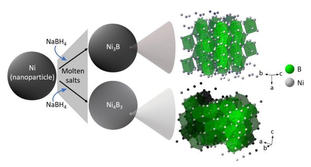
**Figure 1**. Schematic mechanisms of the syntheses of Ni<sub>3</sub>B and Ni<sub>4</sub>B<sub>3</sub> nanocrystals, with the corresponding crystal structures.
