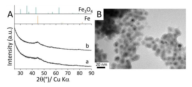
**Figure S6-III**. (A) Powder XRD patterns of the powders obtained from the reaction of Fe-Fe<sub>3</sub>O<sub>4</sub> nanoparticles with NaBH<sub>4</sub> in the molten eutectic mixture LiCl:KCl at 600 °C for 3 h with initial Fe:B atomic ratios (a) 1:1.3 and (b) 2:1.3. (B) TEM image of the sample obtained with Fe:B = 2:1.3.
