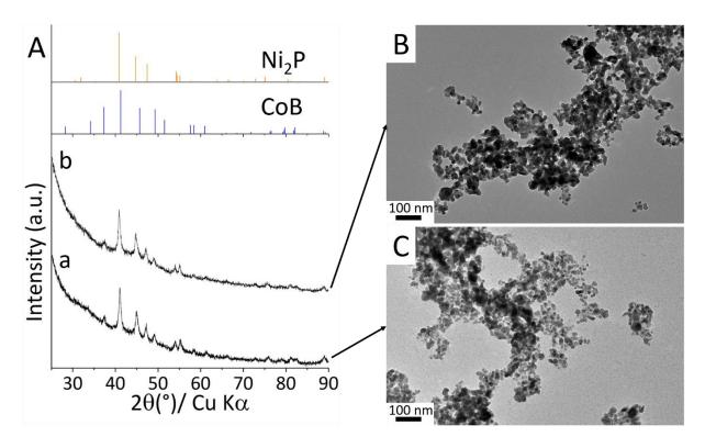
**Figure S5-I**. (A) Powder XRD patterns and (B, C) corresponding TEM images of nanoparticles obtained with the reagent ratio Metal:B = 1:1.3 at 600 °C for 3 h in molten (a) LiI:KI (58:42 mass.), (b) LiCl:KCl (44:56 mass.).
