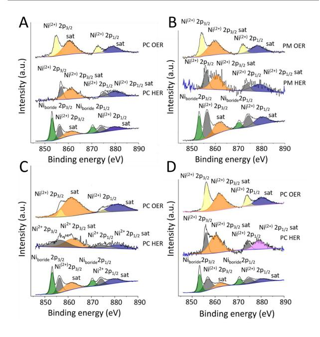
**Figure S3-V.** XPS spectra of electrodes and post-catalysis (PC) after chronopotentiometry at |10| mA.cm<sup>-2</sup> under HER and OER conditions for 8 h, compared to the pristine nanoparticles: (A) crystalline Ni<sub>3</sub>B, (B) crystalline Ni<sub>4</sub>B<sub>3</sub>, (C) amorphous Ni<sub>3</sub>B and (D) amorphous Ni<sub>4</sub>B<sub>3</sub>.
