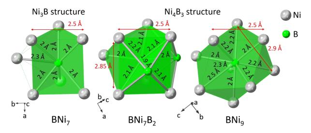
**Figure 4**. Single boron polyhedra constituting the Ni<sub>3</sub>B and Ni<sub>4</sub>B<sub>3</sub> crystal structures. The red marks indicate the distances between nickel atoms not directly engaged in a binding.
