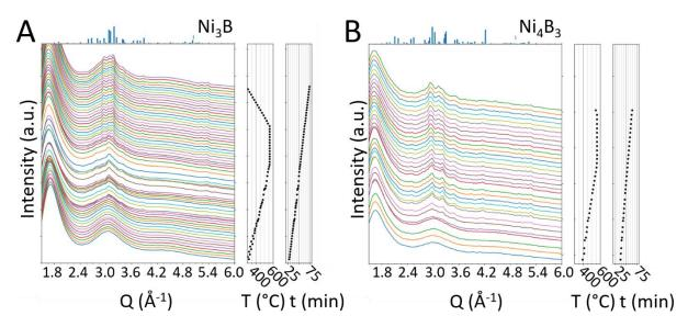
**Figure S2-IV.** *In situ* powder X-ray diagrams in total X-ray scattering configuration for (A) Ni<sub>3</sub>B and (B) Ni<sub>4</sub>B<sub>3</sub> mixtures.
