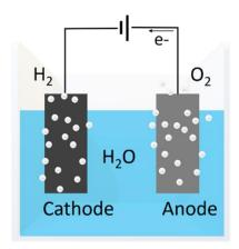
Figure 1: Scheme of an electrochemical water splitting cell.
