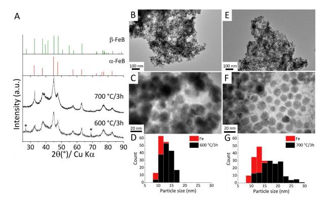
**Figure 2**. (A) Powder XRD patterns, (B, C, E, F) TEM images and (D, G) corresponding size distributions for the products obtained by reacting HDA-derived Fe nanoparticles with NaBH<sub>4</sub> (initial Fe:B atomic ratio 1:1.3) in the molten eutectic mixture LiCl:KCl. The products were obtained by reaction at (B-D) 600 and 700 °C (E-G). \*: unindexed peaks.
