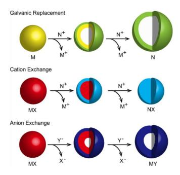
**Figure 1**. Schemes of exchange reactions in nanomaterials: galvanic replacement, cation exchange, anion exchange. The voids are represented by white areas. Adapted from <sup>20</sup>.
