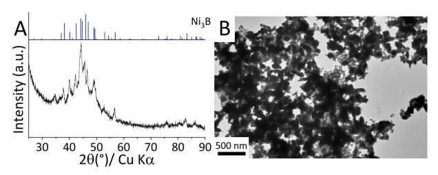
**Figure S2-XI**. (A) Powder XRD pattern (A) and (B) TEM image of Ni<sub>3</sub>B nanoparticles synthetized without impregnation using a hexane dispersion of nickel nanoparticles.
