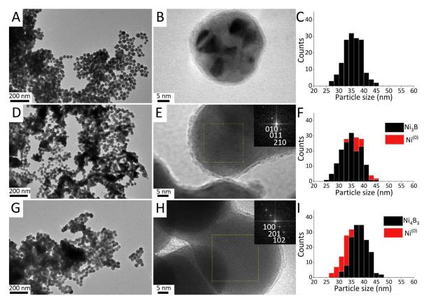
**Figure 2**. TEM study of (A-C) Ni<sup>(0)</sup> nanoparticles, (D-F) Ni<sub>3</sub>B nanocrystals and (G-I) Ni<sub>4</sub>B<sub>3</sub> nanoparticles: (A, D, G) TEM images; (B, E, H) HRTEM images with FFTs of the squared areas, indexed along the corresponding crystal structures of borides; (C, F, I) particle size
