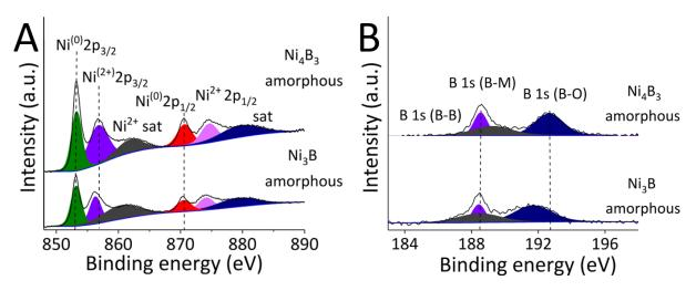
**Figure S2-VI.** XPS of amorphous Ni<sub>3</sub>B and Ni<sub>4</sub>B<sub>3</sub> nanoparticles: (A) Ni 2p region, (B) B 1s region.
