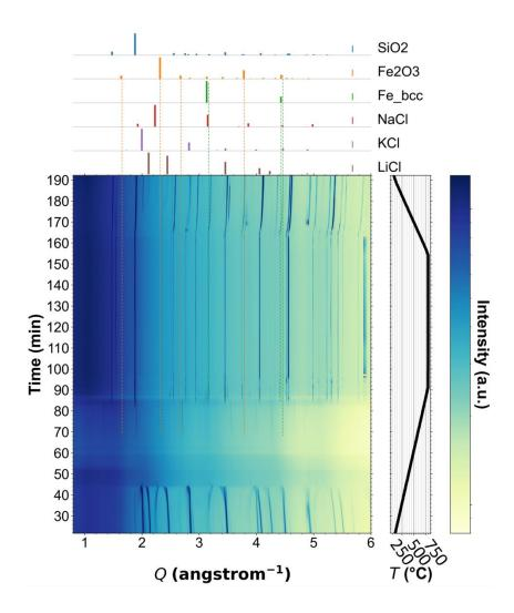
**Figure S6-IV**. Synchrotron radiation-based *in situ* XRD diagrams recorded during the reaction of bcc-Fe nanoparticles from the Peng et al. procedure  $^{13}$  with NaBH<sub>4</sub> (initial Fe:B = 1:1.3 at.) in the eutectic mixture LiCl:KCl. The heating ramp was recalibrated based on the heating point of the salt mixture.
