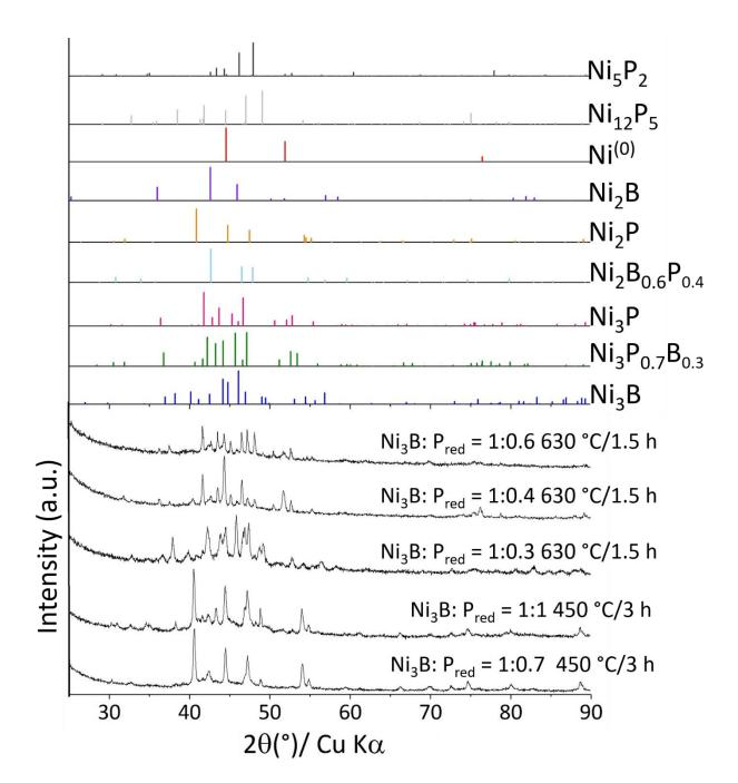
**Figure S4-IV**. Powder XRD patterns of the products obtained from the reaction of red phosphorus with Ni<sub>3</sub>B nanoparticles in the molten eutectic mixture LiI:KI. and (B) nanoparticles.
