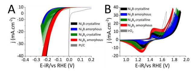
**Figure S3-I**. Cyclic voltammetry recorded with boride catalysts for 30 cycles until stabilization of the electrochemical response, under (A) HER conditions in Ar-saturated 0.5 M H<sub>2</sub>SO<sub>4</sub>, (B) OER in Fe purified O<sub>2</sub>-saturated 0.1 M KOH. For comparison, The Pt/C and IrO<sub>2</sub> benchmark curves corresponding to the first CV cycle are also plotted.
