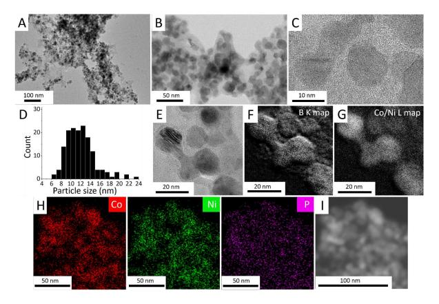
**Figure 8**. Transmission electron microscopy study of Ni-Co-B nanoparticles obtained by obtained by reacting Ni-Co nanoparticles with NaBH<sub>4</sub> (metal:B = 1:2.6 at.) at 600 °C for 1.5 h in molten LiI:KI. (A-C) TEM and HRTEM images and (D) corresponding size distribution. (E) TEM and corresponding EFTEM images at the (F) B-K and (G) Co-L edge. (H) STEM-EDS chemical maps of Co, Ni and P with (I) the corresponding TEM image.
