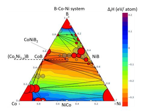
**Figure 4**. Predicted formation energy diagram of Ni-Co-B according to Matlearn<sup>49</sup>. White crosses indicate reported compositions in the training database. Red areas show the low formation energy zones. Red circles indicate predicted compositions on the convex hull, grey circles indicate compositions slightly above the convex hull, hence potentially metastable. The dotted line represents the targeted compositions.
