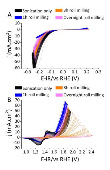
**Figure 4**. Cyclic voltammetry recorded under (A) HER in 0.5 M H<sub>2</sub>SO<sub>4</sub>, (B) OER in Fe purified 0.1 M KOH with roll milling under argon for 1h, 3h and overnight in comparison to the case of sonication only.
