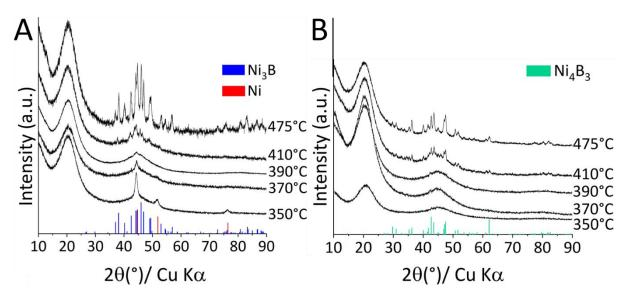
**Figure S2-V.** *Ex situ* powder XRD patterns of samples retrieved at different temperatures for 1.5 h plateaus from the (A) Ni<sub>3</sub>B and (B) Ni<sub>4</sub>B<sub>3</sub> reaction mixtures.
