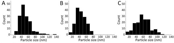
**Figure S-I**. Size distributions of nickel particles obtained by the reaction of NiCl<sub>2</sub> with NaH in molten LiI:KI (58:42 mass.) by induction heating at (A) 350 °C for 20 min, (B) 500 °C 30 s. and (C) 600 °C for 30 s.
