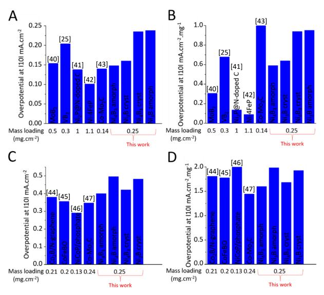
**Figure S3-III**. Overpotentials and mass normalized overpotentials measured at |10| mA cm<sup>-2</sup> in (A-B) HER and (C-D) OER conditions, for selected transition metal borides, phosphides and carbides from the literature and from the present work. Data reported for (A-B) HER and (C-D) OER correspond to 0.5 M H<sub>2</sub>SO<sub>4</sub> and 0.1 M KOH electrolytes, respectively.
