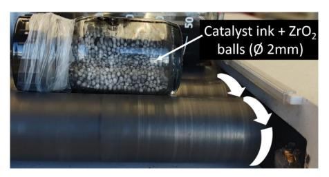
Figure 3. Experimental setup for ink dispersion studies by roll milling with zirconia balls.
