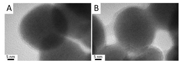
**Figure S2-VIII**. HRTEM images of Ni<sub>3</sub>B nanoparticles obtained by synthesis at 475 °C for 1.5 h: of (A) single amorphous nanoparticle, (B) coalesced amorphous nanoparticles.
