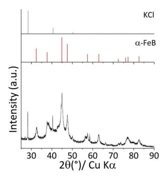
**Figure S6-VI**. Powder XRD pattern of the particles synthetized with Fe:B = 2:1.3 at. ratio at 700 °C for 3 h in molten LiCl:KCl.
