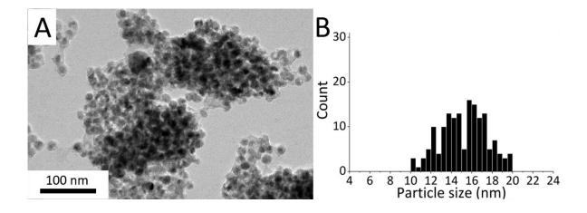
**Figure S5-III**. TEM image and the corresponding size distribution of the sample obtained by reacting Ni-Co nanoparticles with NaBH<sub>4</sub> (metal:B = 1:2.6 at.) at 600 °C for 1.5 h in LiI:KI.
