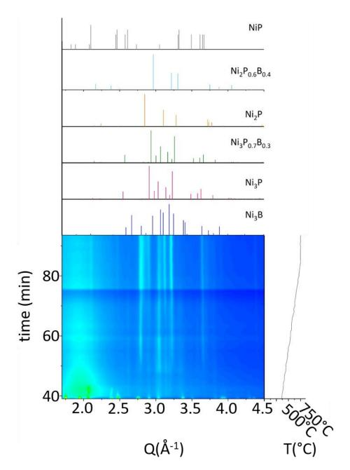
**Figure 4.** Synchrotron *in situ* XRD diagrams recorded during heating of a reaction mixture containing  $Ni_3B$  nanoparticles and red phosphorus in proportions  $Ni_3B:P_{red}=1:0.7$  at. in the molten eutectic mixture LiI:KI.
