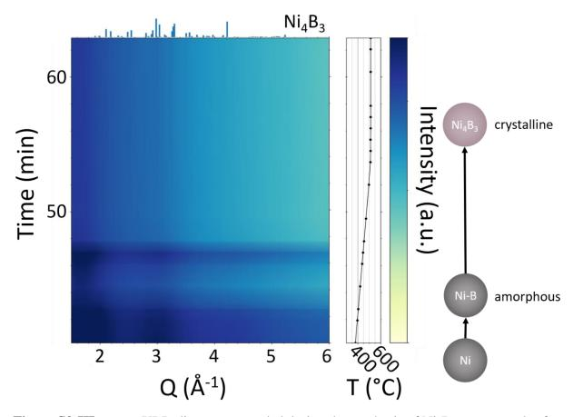
**Figure S2-III.** *In situ* XRD diagrams recorded during the synthesis of Ni<sub>4</sub>B<sub>3</sub> nanocrystals after melting of the eutectic salt mixture.
