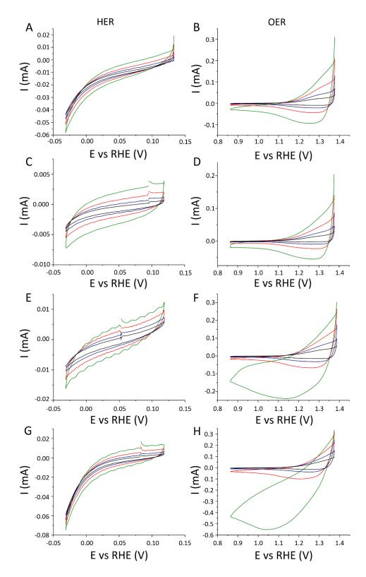
**Figure S3-IV**. Cyclic voltammetry curves recorded at scan rates of 2.5, 5, 10, 20 mV s<sup>-1</sup> in a low faradic region in HER and OER to estimate the double layer capacitance (C<sub>DL</sub>). (A, B) Ni<sub>3</sub>B crystalline, (C, D) Ni<sub>3</sub>B amorphous, (E, F) Ni<sub>4</sub>B<sub>3</sub> crystalline, (G, H) Ni<sub>4</sub>B<sub>3</sub> amorphous.
