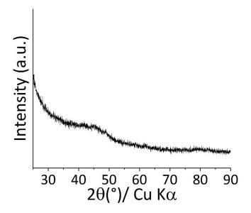
**Figure S5-IV**. XRD pattern of the powder obtained by reacting Ni-Co nanoparticles with NaBH<sub>4</sub> (metal:B = 1:2.6 at.) at 450  $^{\circ}$ C for 6 h in LiI/KI.
