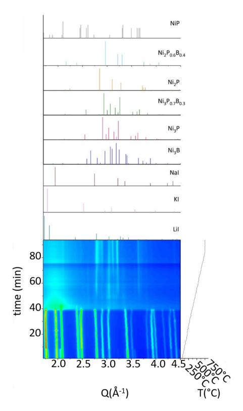
**Figure S4-III**. *In situ* XRD diagrams recorded during the reaction of  $Ni_3B$  with red phosphorus with the ratio  $Ni_3B$ : $P_{red} = 1:0.7$  at. in the eutectic mixture LiI:KI.
