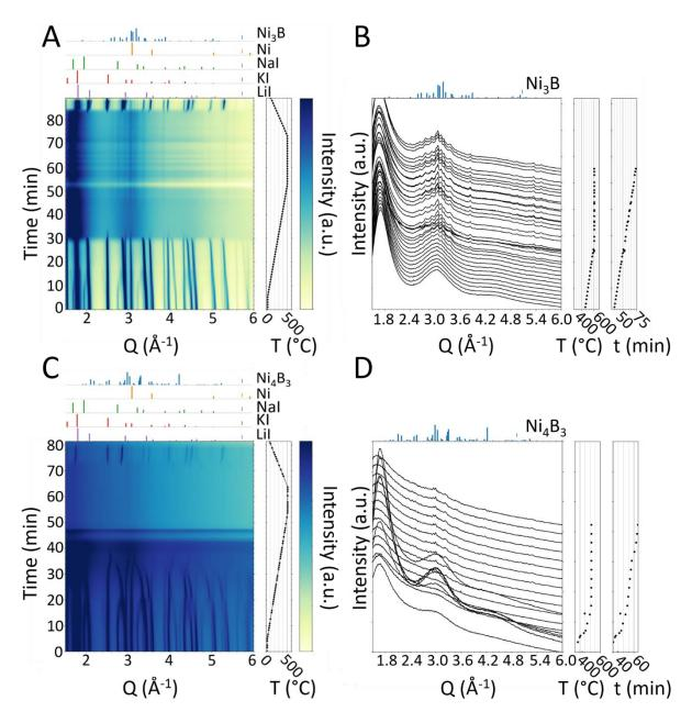
**Figure S2-II.** In situ XRD diagrams recorded during the synthesis of (A, B) Ni<sub>3</sub>B and (C, D) Ni<sub>4</sub>B<sub>3</sub> nanocrystals.
