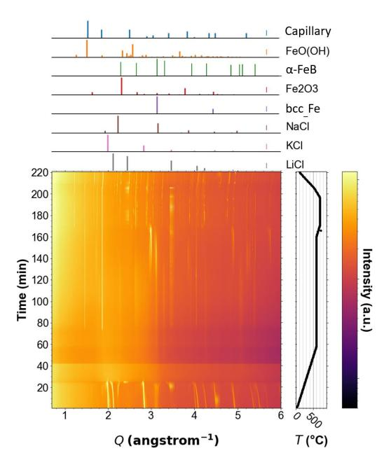
**Figure 3**. Synchrotron radiation-based *in situ* XRD diagrams recorded during the reaction of bcc-Fe nanoparticles with NaBH<sub>4</sub> (initial Fe:B = 1:1.3 at.) in the eutectic mixture LiCl:KCl.
