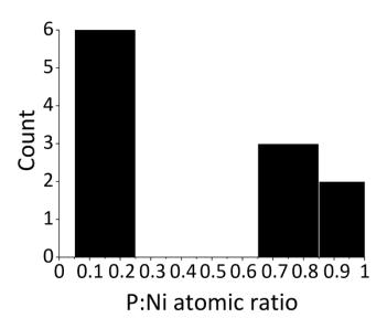
**Figure S4-VIII**. P:Ni atomic ratio distribution observed by STEM-EDX on 11 single particles from the sample obtained by the reaction of NiCl<sub>2</sub>, NaBH<sub>4</sub> and  $P_{red}$  (2:4:0.4 at. ratio) at 600 °C for 3h in the molten eutectic mixture LiCl:KCl.
