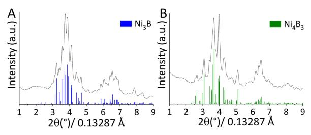
**Figure S2-I.** Powder XRD diagrams of (A)  $Ni_3B$  and (B)  $Ni_4B_3$  nanocrystals acquired in total X-ray scattering configuration by using synchrotron-based radiation, with wavelength 0.13287 Å.
