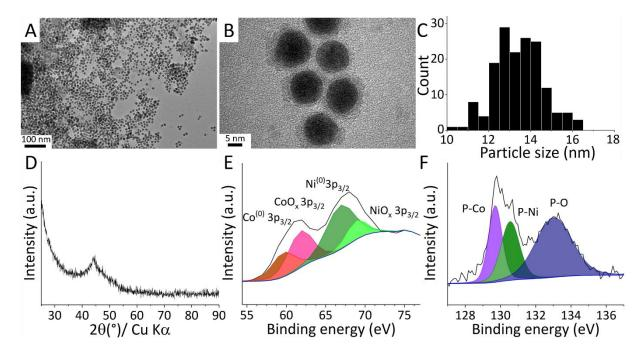
**Figure 3.** Ni-Co core-shell nanoparticles. (A) TEM image, (B) high magnification TEM image showing no local order and (C) size distribution of the particles, (D) powder XRD pattern, (E) XPS in the Co/Ni 3p<sub>3/2</sub> region, (F) XPS in the P 2p region.
