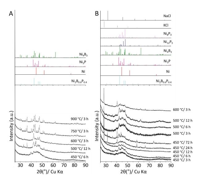
**Figure S4-VII**. Powder XRD patterns of the powders obtained from the reaction of NiCl<sub>2</sub>, NaBH<sub>4</sub> and P<sub>red</sub> in the molten eutectic mixture LiCl:KCl performed to target reported Ni-B-P ternary phases using Ni:B:P atomic ratio of (A) 3:6:0.7 and (B) 2:4:0.4. Some KCl and NaCl remains in some powder due to inefficient washing.
