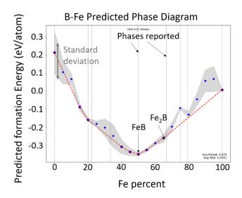
**Figure S6-II**. Predicted phase diagram at 0 K of Fe-B from the machine learning tool Matlearn<sup>15</sup>. The red dotted line corresponds to the convex hull. The blue point are phases predicted and the continuous vertical lines correspond to the phases reported.
