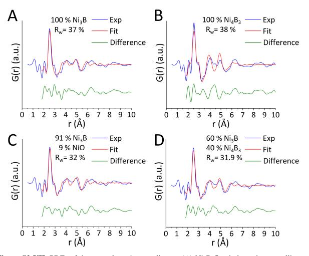
**Figure S2-VII.** PDFs of the amorphous intermediate to (A) Ni<sub>3</sub>B fitted along the crystalline structure of Ni<sub>3</sub>B, (B) Ni<sub>4</sub>B<sub>3</sub> fitted along the crystalline structure Ni<sub>4</sub>B<sub>3</sub>. PDF of the amorphous intermediate to Ni<sub>3</sub>B fitted along the crystalline structure of (C) Ni<sub>3</sub>B mixed with NiO, (D) Ni<sub>3</sub>B mixed with Ni<sub>4</sub>B<sub>3</sub>.
