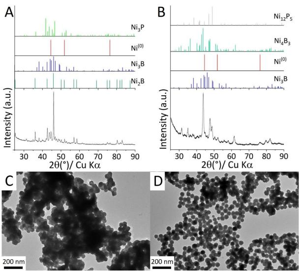
**Figure S2-IX**. Syntheses of borides nanoparticles without molten salts. XRD pattern and corresponding TEM images of (A, C) Ni<sub>3</sub>B mixture, (B, D) Ni<sub>4</sub>B<sub>3</sub> mixture.
