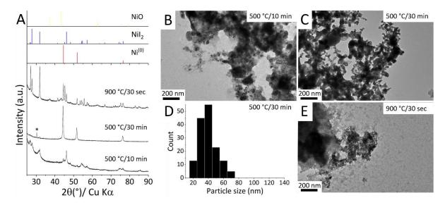
**Figure 3**. (A) XRD pattern and (B-E) TEM images of the powders obtained from mixtures NiI<sub>2</sub>:NaH (1:5 at.) reacted in the molten eutectic mixture LiI:KI heated by induction.
