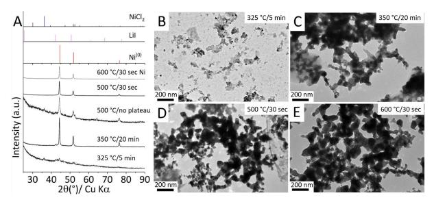
**Figure 2**. (A) XRD patterns and (B-E) TEM images of the powders obtained from mixtures NiCl<sub>2</sub>:NaH (1:5 at.) reacted in the molten eutectic mixture LiI:KI heated by induction.
