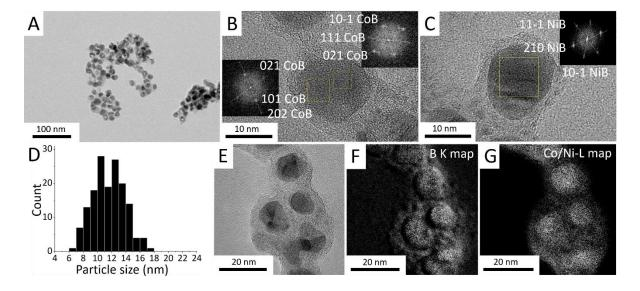
**Figure 6**. Morphology and composition study of bimetallic boride nanoparticles obtained by reacting Ni-Co nanoparticles with NaBH<sub>4</sub> (metal:B = 1:2.6 at.) at 600 °C for 0.5 h in molten LiI:KI. (A) TEM and (B, C) HRTEM images with corresponding FFTs. (D) Corresponding size distribution. (E) TEM and corresponding EFTEM images at the (F) B-K and (G) Co/Ni-L edges.
