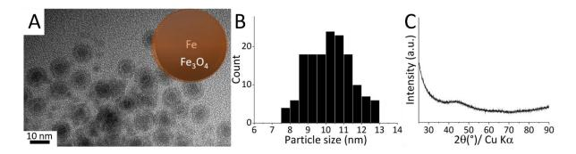
**Figure S6-I**. Fe nanoparticles synthesized by colloidal chemistry  $^{13}$  using Fe(CO)<sub>8</sub> as precursor. (A) TEM image and the corresponding scheme of the core-shell Fe-Fe<sub>3</sub>O<sub>4</sub> structure, corresponding (B) size distribution and (C) powder XRD pattern.
