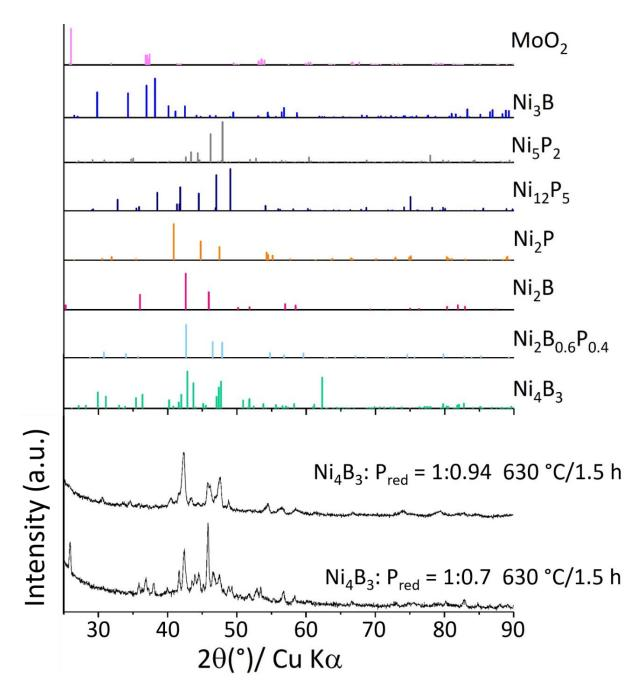
**Figure S4-V**. Powder XRD patterns of the products obtained from the reaction of red phosphorus with Ni<sub>4</sub>B<sub>3</sub> nanoparticles in the molten eutectic mixture LiI:KI.
