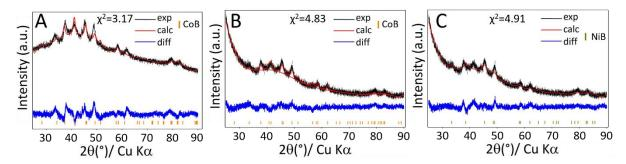
**Figure S5-II**. Powder XRD patterns and corresponding Rietveld refinements for the samples obtained by reacting Ni-Co nanoparticles with NaBH<sub>4</sub> (metal:B = 1:2.6 at.) at 600 °C for (A) 0.5 h by considering only CoB as constituent; for 1.5 h by considering (B) only CoB and (C) only NiB as references.
