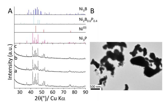
**Figure S4-IX**. (a-c) XRD diagrams of the powders obtained by reacting NiCl<sub>2</sub>, NaBH<sub>4</sub> and  $P_{red}$  with a large excess of NaH in the molten eutectic mixture LiCl:KCl. With initial reagents ratios Ni:B:P (a) 3:0.25:0.75, (b) 3:0.39:0.7, (c) 3:0.75:0.25 at 600 °C/3 h. (d) TEM image of powder obtained with the ratio 3:0.39:0.7
