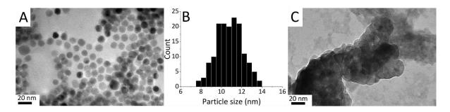
**Figure S4-II**. TEM image of (A) Ni<sub>2</sub>P nanoparticles with (B) corresponding size distribution. (C) TEM image of a Ni<sub>3</sub>P sample.
