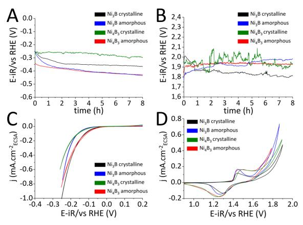
**Figure S3-II**. Chrono potentiometry (CP) for 8 h recorded at a current density of |10| mA.cm<sup>2</sup> on a 1 cm<sup>2</sup> carbon paper working electrode during (A) HER, (B) OER. Surface area normalized CV curves at the 30<sup>th</sup> cycle during (C) HER, (D) OER.
