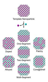
**Figure 2**. Examples of diverse structures reported by cation exchange reactions. Reproduced from <sup>37</sup>.
