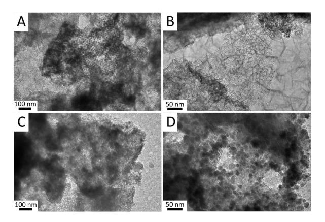
**Figure S6-V**. TEM images of  $\alpha$ -FeB nanoparticles synthetized at (A, B) 600 °C for 3 h, (C, D) 700 °C for 3 h by dispersion of the nanoparticles into methanol before deposition on a TEM carbon-coated copper grid and drying under air.
