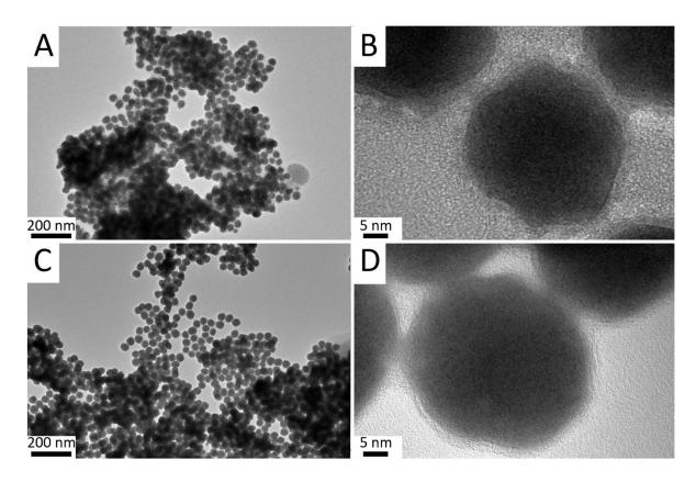
**Figure 6**. TEM pictures of the amorphous nanoparticles formed during the synthesis of (A, B) Ni<sub>3</sub>B and (C, D) Ni<sub>4</sub>B<sub>3</sub> nanocrystals. (A, C) Low and (B, D) high magnification images.
