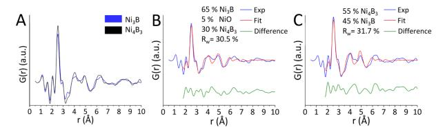
**Figure 7**. (A) *Ex situ* PDFs of the amorphous intermediates retrieved in the course of the syntheses of Ni<sub>3</sub>B and Ni<sub>4</sub>B<sub>3</sub>. (B) PDF of Ni<sub>3</sub>B refined as a mixture of Ni<sub>3</sub>B, Ni<sub>4</sub>B<sub>3</sub> and NiO crystal structures. (C) PDF of Ni<sub>4</sub>B<sub>3</sub> refined as a mixture of Ni<sub>4</sub>B<sub>3</sub> and Ni<sub>3</sub>B.
