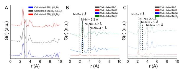
**Figure 8**. (A) Calculated PDF of the isolated polyhedra consisting of Ni<sub>3</sub>B (BNi<sub>7</sub>) and Ni<sub>4</sub>B<sub>3</sub> (BNi<sub>7</sub>B<sub>2</sub>, BNi<sub>9</sub>). The rectangle highlights the 2.9 Å peak unobserved in the BNi<sub>7</sub> coordination of Ni<sub>3</sub>B. Calculated PDF of the (B) Ni<sub>3</sub>B and (C) Ni<sub>4</sub>B<sub>3</sub> structures in a range of 9 Å and assignment of the contributions of B-B, Ni-B and Ni-Ni distances.
