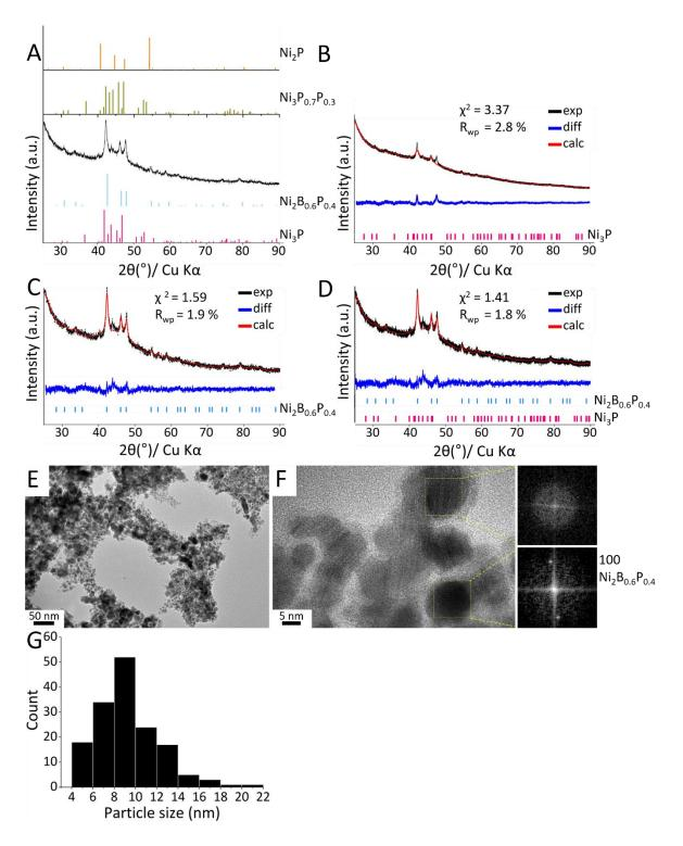
**Figure 5.** (A) Powder XRD pattern and corresponding Rietveld refinements performed by implementation of (B) Ni<sub>3</sub>P, (C) Ni<sub>2</sub>B<sub>0.6</sub>P<sub>0.4</sub>, (D) both Ni<sub>3</sub>P and Ni<sub>2</sub>B<sub>0.6</sub>P<sub>0.4</sub>. (E, F) TEM pictures including Fast Fourier Transform on selected particles, (G) Diagram of size distribution.
