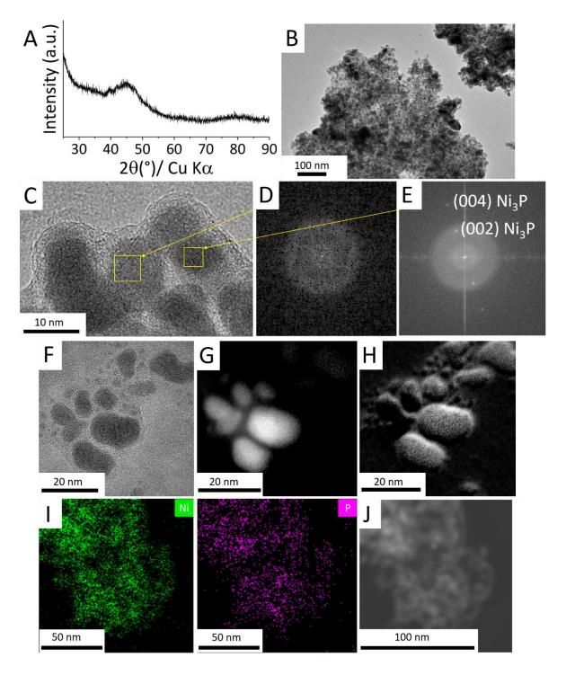
**Figure 7.** Nickel borophosphide obtained by reacting NiCl<sub>2</sub>, NaBH<sub>4</sub> and P<sub>red</sub> (2:4:0.4 at. ratio) at 450 °C/3 h in the molten eutectic mixture LiCl:KCl. (A) Powder XRD pattern, (B) TEM and (C) HRTEM images with (D-E) corresponding FFTs. (F) TEM and corresponding EFTEM images at the (G) Ni-L and (H) B-K edges. (I) STEM-EDX chemical maps of Ni and P with (J) the corresponding TEM image.
