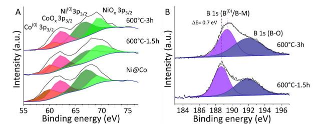
**Figure 9**. XPS spectra of Ni-Co nanoparticles and the products of their reaction with NaBH<sub>4</sub> in molten LiI:KI for a metal:B ratio of 1:2.6 at. at 600 °C for 1.5 and 3 h: (A) Ni, Co 3p region and (B) B 1s region.
