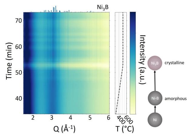
**Figure 5**. *In situ* XRD diagrams recorded during the synthesis of Ni<sub>3</sub>B nanocrystals after melting of the eutectic salt mixture.
