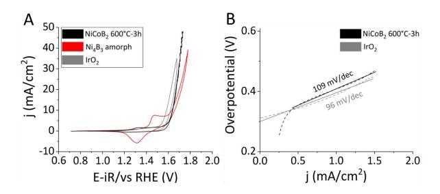
**Figure 11**. Electrochemical properties of nanocrystals obtained with metal:B ratio = 1:2.6 at. after 600 °C for 3 h. OER study in aqueous O<sub>2</sub>-saturated 0.1 M KOH Fe-free electrolyte: (A) CV curves at the 1<sup>st</sup> cycle compared to Ni<sub>4</sub>B<sub>3</sub> amorphous nanoparticles and IrO<sub>2</sub>, (B) Tafel slope compared to IrO<sub>2</sub>.
