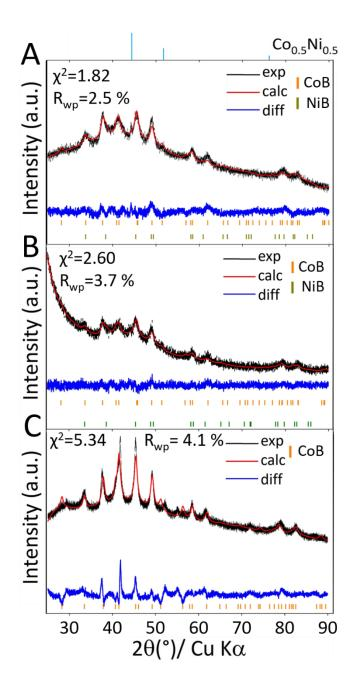
**Figure 5**. Rietveld refinements of the XRD pattern of powders obtained by reacting Ni-Co nanoparticles with NaBH<sub>4</sub> for metal:B = 1:2.6 at. in LiI:KI at 600 °C for (A) 0.5, (B) 1.5, and (C) 3 h. The phase indexed  $Co_{0.5}Ni_{0.5}$  in (A) was not accounted for in the refinement, as adding this third phase led to misinterpretation due to a large number of variables involved in the fit.
