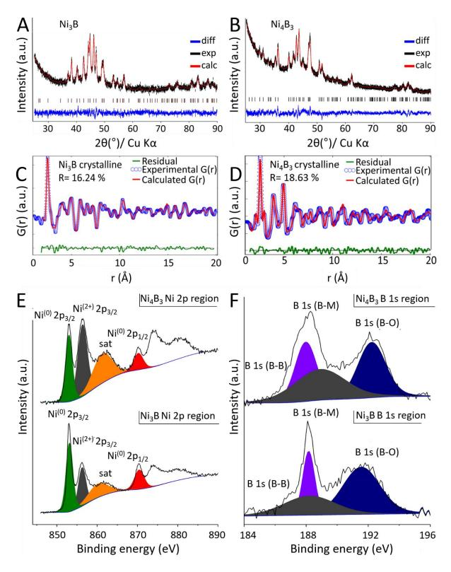
**Figure 3**. XRD patterns with corresponding Rietveld refinements of (A) Ni<sub>3</sub>B and (B) Ni<sub>4</sub>B<sub>3</sub> nanocrystals. Pair distribution functions of (C) Ni<sub>3</sub>B and (D) Ni<sub>4</sub>B<sub>3</sub> nanocrystals fitted along the corresponding crystal structures. XPS of Ni<sub>3</sub>B and Ni<sub>4</sub>B<sub>3</sub> in (E) Ni 2p (F) B 1s region.
