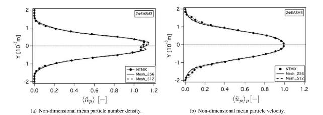
Figure 5.71: Comparison Lagrangian and Eulerian results. The Lagrangian computation has been performed in a 128<sup>3</sup> mesh grid. Mesh\_256 corresponds to the Eulerian simulation on a 256<sup>3</sup> mesh and Mesh\_512 to an Eulerian simulation on a 512<sup>3</sup> mesh.
