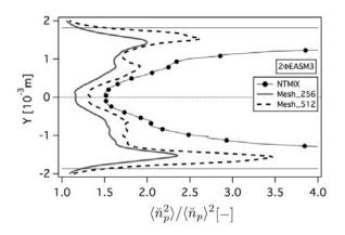
Figure 5.73: Comparison Lagrangian and Eulerian particle segregation. The Lagrangian computation has been performed in a 128<sup>3</sup> mesh grid. Mesh\_256 corresponds to the Eulerian simulation on a 256<sup>3</sup> mesh and Mesh\_512 to an Eulerian simulation on a 512<sup>3</sup> mesh.
