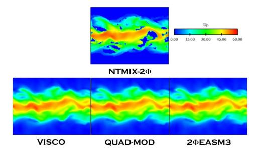
Figure 5.55: Comparison of Lagrangian (NTMIX-2 $\Phi$ ) and Eulerian particle velocity magnitude ( $U_p$ ) at 80 $t_{ref}$ . LR\_St033\_# case.
