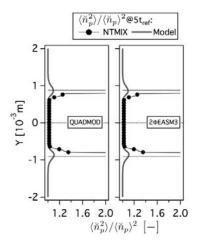
Figure F.3: Comparison of Eulerian and Lagrangian RMS particle segregation  $(\langle \breve{n}_p^2 \rangle / \langle \breve{n}_p \rangle^2)$  at  $5t_{ref}$ . HR\_St1\_# case.
