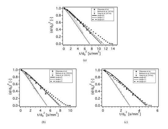
Figure 7.8: Temporal evolution of the non-dimensional droplet surface. n-heptane, P = 1bar: (a) T = 473K, (b) T = 548K, (c) T = 748K. Numerical simulations performed using the AS evaporation model. Experimental results of Chauveau et al. (2008) and Nomura et al. (1996); numerical results of case 1 in Yang & Wong (2001).
