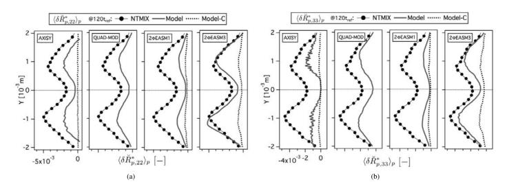
Figure 5.47: Comparison of Eulerian and Lagrangian (a) mean deviatoric RUM stress tensor YY component ( $\langle \delta \breve{R}_{p,22}^* \rangle_p$ ) and (b) mean deviatoric RUM stress tensor ZZ component ( $\langle \delta \breve{R}_{p,33}^* \rangle_p$ ) at 120t<sub>ref</sub>. Normalized by the square of the initial particle velocity in X-direction at the center of the slab. LR\_St3\_# case.
