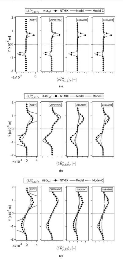
Figure 5.28: Comparison of Eulerian and Lagrangian mean deviatoric RUM stress tensor XY component ( $< \delta \breve{R}_{p,12}^* >_p$ ) at 5, 40 and 80t<sub>ref</sub>. Normalized by the square of the initial particle velocity in X-direction at the center of the slab. LR\_St1\_# case.
