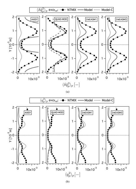
Figure D.4: Comparison of Eulerian and Lagrangian (a) mean Random Uncorrelated Energy ( $<\delta \check{q}_p >_p$ ) and (b) mean mesoscopic ( $\langle (\dot{q}_p^2 \rangle_p)$ ) and mesoscopic ( $\langle (\dot{q}_p^2 \rangle_p)$ ) particle energies at  $40t_{ref}$ . Normalized by the square of the initial particle velocity in X-direction at the center of the slab. LR\_St3\_# case.
