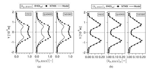
Figure E.9: Comparison of Eulerian and Lagrangian (a) RMS particle number density ( $\langle \breve{n}_{p,RMS} \rangle$ , normalized by the initial particle number density at the center of the slab) and (b) RMS particle velocity in X-direction ( $\langle \breve{u}_{p,RMS} \rangle_p$ , normalized by the initial particle number density at the center of the slab)at 40t<sub>ref</sub>. LR\_St033\_# case.
