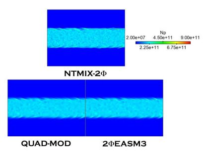
Figure F.15: Comparison of Lagrangian (NTMIX- $2\Phi$ ) and Eulerian particle number density ( $N_p$ ) at  $5t_{ref}$ . HR\_St1\_# case.
