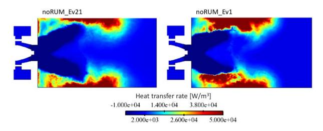
Figure 9.28: Evaporation heat transfer rate instantaneous fields. Cases noRUM\_Ev1 (right) and noRUM\_Ev21 (left).
