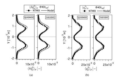
Figure F.11: Comparison of Eulerian and Lagrangian (a) mean Random Uncorrelated Energy ( $\langle \delta \breve{q}_p \rangle_p$ ) and (b) mean mesoscopic ( $\langle \breve{q}_p^2 \rangle_p$ ) particle energies at  $40t_{ref}$ . Normalized by the square of the initial particle velocity in X-direction at the center of the slab. HR\_St1\_# case.
