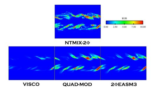
Figure E.20: Comparison of Lagrangian (NTMIX-2 $\Phi$ ) and Eulerian Random Uncorrelated Energy at 40 $t_{ref}$ . LR\_St033\_# case.
