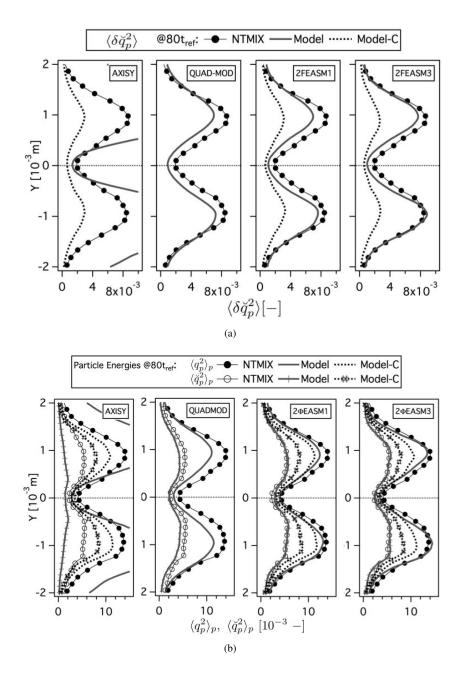
Figure D.12: Comparison of Eulerian and Lagrangian (a) mean Random Uncorrelated Energy ( $\langle \delta \check{q}_p \rangle_p$ ) and (b) mean total  $(\langle q_p^2 \rangle_p)$  and mesoscopic  $(\langle \check{q}_p^2 \rangle_p)$  particle energies at  $80t_{ref}$ . Normalized by the square of the initial particle velocity in X-direction at the center of the slab. LR\_St3\_# case.
