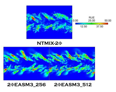
Figure 5.77: Comparison Lagrangian and Eulerian RUE instantaneous fields at  $40t_{ref}$ . The Lagrangian computation has been performed in a  $128^3$  mesh grid.  $2\Phi EASM3_256$  corresponds to the Eulerian simulation on a  $256^3$  mesh and  $2\Phi EASM3_512$  to an Eulerian simulation on a  $512^3$  mesh.
