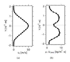
Figure 5.10: Comparison of AVBP (—) and NTMIX-2 $\Phi$  (-•-) carrier phase velocities in X-direction. HR\_St1\_# case. (a) Mean velocity ( $U_f$ ) and (b) RMS velocity times the fluid density ( $\rho_f U_{f,RMS}$ ) at 70 $t_{ref}$ .
