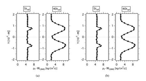
Figure B.3: Comparison of Eulerian and Lagrangian carrier phase velocities in Z-direction. HR\_St1\_# case. (a) Mean velocity ( $W_f$ ) and (b) RMS velocity times the fluid density ( $\rho_f W_{f,RMS}$ ) at 5 and  $40t_{ref}$ . Simulations performed with AVBP (—) and NTMIX-2 $\Phi$  (- $\bullet$ -).
