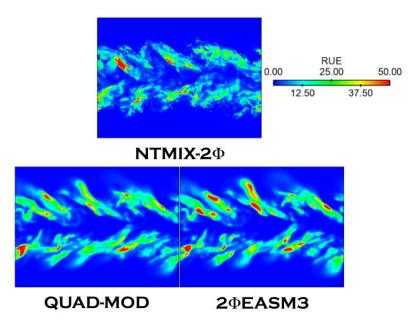
Figure F.20: Comparison of Lagrangian (NTMIX-2 $\Phi$ ) and Eulerian Random Uncorrelated Energy at 40 $t_{ref}$ . HR\_St1\_# case.
