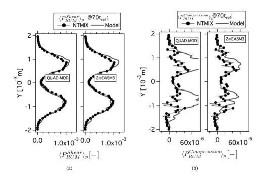
Figure 5.67: Comparison of Eulerian and Lagrangian (a) mean production of RUM energy by shear ( $\langle P_{RUM}^{Shear} \rangle_p$ ) and (b) mean productions of RUM energy by compression ( $\langle P_{RUM}^{Compression} \rangle_p$ ) at 70t<sub>ref</sub>. Normalized by the square of the initial particle velocity in X-direction at the center of the slab and the reference time (t<sub>ref</sub>). HR\_St1\_# case.
