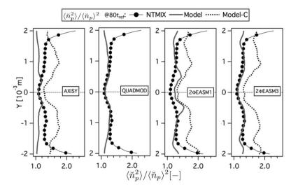
Figure D.11: Comparison of Eulerian and Lagrangian RMS particle segregation  $(\langle \breve{n}_p^2 \rangle / \langle \breve{n}_p \rangle^2)$  at 80t<sub>ref</sub>. LR\_St3\_# case.
