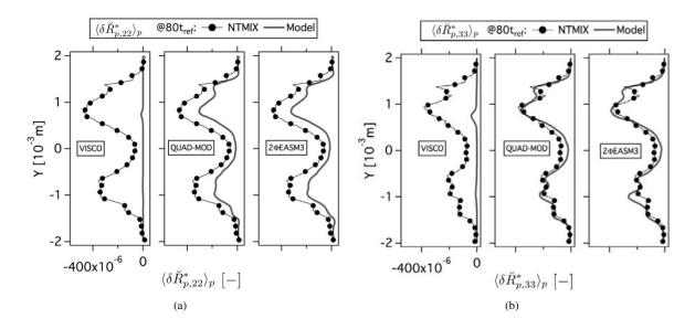
Figure 5.59: Comparison of Eulerian and Lagrangian (a) mean deviatoric RUM stress tensor YY component ( $<\delta \breve{R}_{p,22}^* >_p$ ) and (b) mean deviatoric RUM stress tensor ZZ component ( $<\delta \breve{R}_{p,33}^* >_p$ ) at 80t<sub>ref</sub>. Normalized by the square of the initial particle velocity in X-direction at the center of the slab. LR\_St033\_# case.
