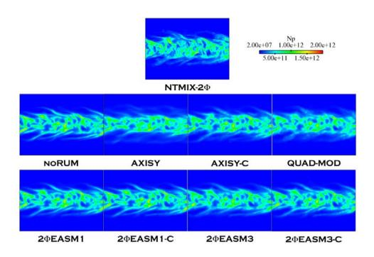
Figure C.2: Comparison of Lagrangian (NTMIX-2 $\Phi$ ) and Eulerian particle number density ( $N_p$ ) at 40t<sub>ref</sub>. LR\_St1\_# case.
