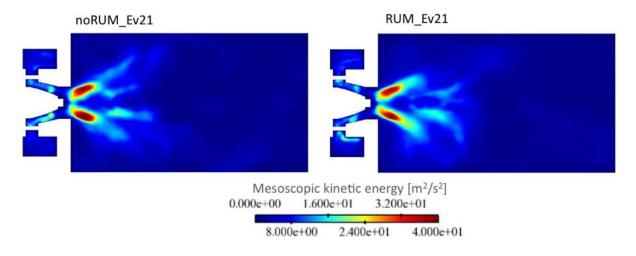
Figure 9.42: Mesoscopic kinetic energy averaged fields. Cases noRUM\_Ev21 (left) and RUM\_Ev21 (right).
