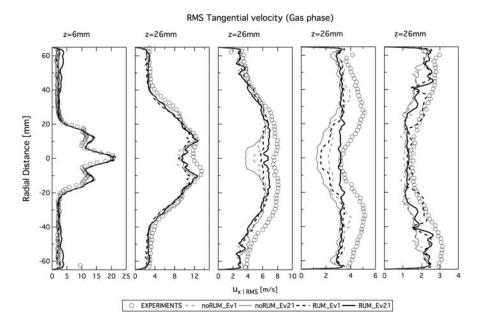
Figure 9.12: RMS tangential velocity profiles. Gaseous phase.
