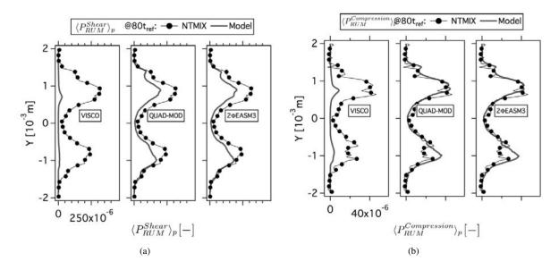
Figure 5.57: Comparison of Eulerian and Lagrangian (a) mean production of RUM energy by shear ( $\langle P_{RUM}^{Shear} \rangle_p$ ) and (b) mean productions of RUM energy by compression ( $\langle P_{RUM}^{Compression} \rangle_p$ ) at 80t<sub>ref</sub>. Normalized by the square of the initial particle velocity in X-direction at the center of the slab and the reference time (t<sub>ref</sub>). LR\_St033\_# case.
