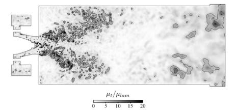
Figure 9.13: Ratio of turbulent to laminar viscosity corresponding to an instantaneous solution of Case RUM\_Ev21.
