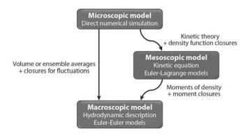
Figure 2.1: Classification of modeling approaches for DNS of two-phase flows. Extracted from Fox (2012).
