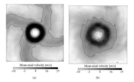
Figure 9.3: Mean gaseous axial velocity in transverse cuts at (a) z = 20 mm and (b) z = 40 mm. Isolines of axial velocity in the range -10 m/s and 25 m/s. Case RUM\_Ev21.
