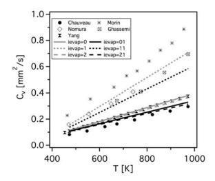
Figure 7.9: Comparison of the vaporization rate of n-heptane isolated droplets, versus temperature. Experimental results of Chauveau et al. (2008), Nomura et al. (1996), Yang & Wong (2001), Morin et al. (2000) and Ghassemi et al. (2006)
