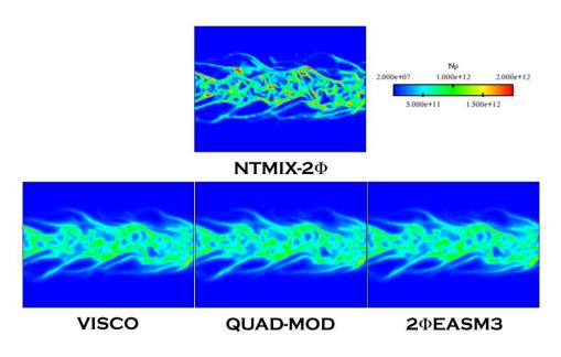
Figure E.16: Comparison of Lagrangian (NTMIX-2 $\Phi$ ) and Eulerian particle number density ( $N_p$ ) at 40t<sub>ref</sub>. LR\_St033\_# case.
