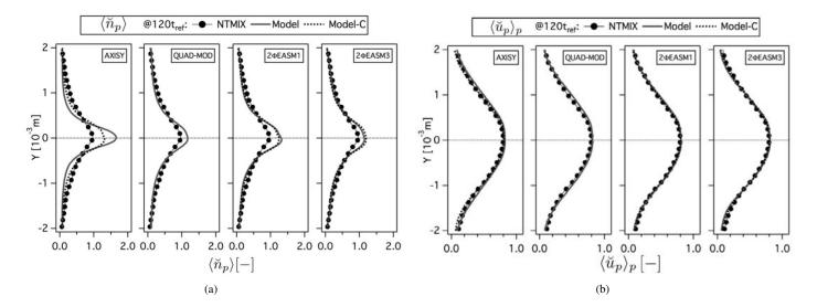
Figure 5.39: Comparison of Eulerian and Lagrangian (a) mean particle number density ( $\langle \breve{n}_p \rangle$ , normalized by the initial particle number density at the center of the slab) and (b) mean particle velocity in X-direction ( $\langle \breve{u}_p \rangle_p$ , normalized by the initial particle velocity in X-direction at the center of the slab) at  $120t_{ref}$ . LR\_St3\_# case.
