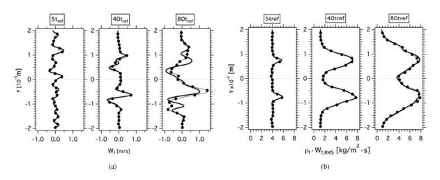
Figure 5.6: Comparison of AVBP (--) and NTMIX-2 $\Phi$  (-•-) carrier phase velocities in Z-direction. LR\_St1\_# case. (a) Mean velocity ( $W_f$ ) and (b) RMS velocity times the fluid density ( $\rho_f W_{f,RMS}$ ).
