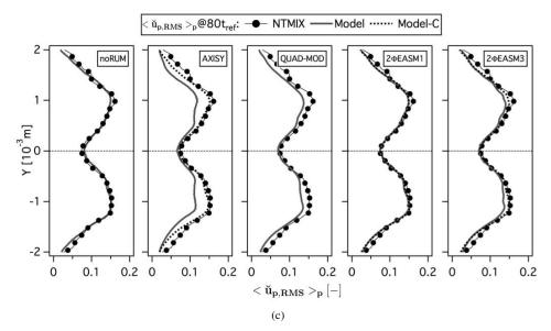
Figure 5.17: Comparison of Eulerian and Lagrangian RMS particle velocity in X-direction ( $\langle \tilde{u}_{p,RMS} \rangle_p$ ) at 5, 40 and 80t<sub>ref</sub>. Normalized by the initial particle velocity in X-direction at the center of the slab. LR\_St1\_# case.
