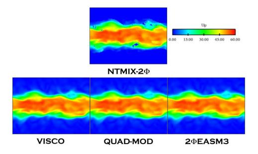
Figure E.18: Comparison of Lagrangian (NTMIX-2 $\Phi$ ) and Eulerian particle velocity magnitude ( $U_p$ ) at 40 $t_{ref}$ . LR\_St033\_# case.
