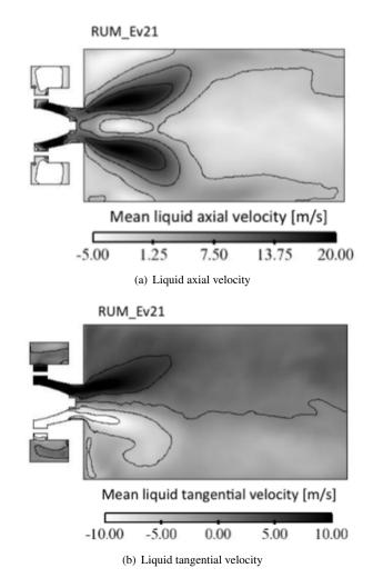
Figure 9.15: Average fields of liquid phase axial (a) and tangential (b) velocities. Case RUM\_Ev21.
