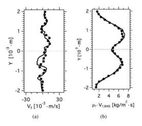
Figure 5.11: Comparison of AVBP (—) and NTMIX-2 $\Phi$  (-•-) carrier phase velocities in Y-direction. HR\_St1\_# case. (a) Mean velocity ( $U_f$ ) and (b) RMS velocity times the fluid density ( $\rho_f U_{f,RMS}$ ) at 70 $t_{ref}$ .
