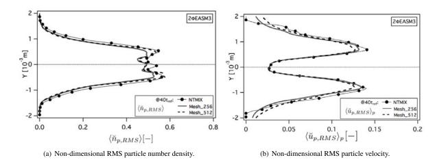
Figure 5.33: Comparison between Lagrangian and Eulerian results. The Lagrangian computation has been performed on a 128<sup>3</sup> mesh grid. Mesh\_256 corresponds to the Eulerian simulation on a 256<sup>3</sup> mesh and Mesh\_512 to the Eulerian simulation on a 512<sup>3</sup> mesh.
