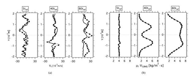
Figure 5.5: Comparison of AVBP (—) and NTMIX-2 $\Phi$  (–•–) carrier phase velocities in Y-direction. LR\_St1\_# case. (a) Mean velocity ( $V_f$ ) and (b) RMS velocity times the fluid density ( $\rho_f V_{f,RMS}$ ).
