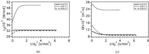
Figure 7.2: Temporal evolution of the main transport properties: (a) gaseous mixture viscosity, (b) thermal conductivity, (c) diffusion coefficient. n-heptane,  $T_g = 623K$ ,  $P_g = 1bar$ . Numerical simulations performed using the AS evaporation model.
