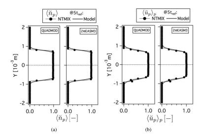
Figure F.1: Comparison of Eulerian and Lagrangian (a) mean particle number density ( $\langle \breve{n}_p \rangle$ , normalized by the initial particle number density at the center of the slab) and (b) mean particle velocity in X-direction ( $\langle \breve{u}_p \rangle_p$ , normalized by the initial particle velocity in X-direction at the center of the slab) at  $5t_{ref}$ . HR\_St1\_# case.
