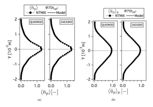
Figure 5.61: Comparison of Eulerian and Lagrangian (a) mean particle number density ( $\langle \breve{n}_p \rangle$ , normalized by the initial particle number density at the center of the slab) and (b) mean particle velocity in X-direction ( $\langle \breve{u}_p \rangle_p$ , normalized by the initial particle velocity in X-direction at the center of the slab) at 70t<sub>ref</sub>. HR\_St1\_# case.
