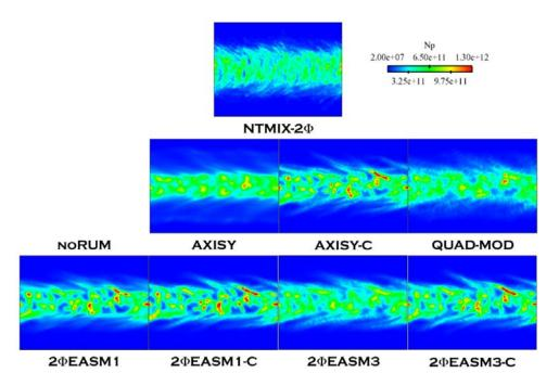
Figure D.17: Comparison of Lagrangian (NTMIX-2 $\Phi$ ) and Eulerian particle number density ( $N_p$ ) at 40 $t_{ref}$ . LR\_St3\_# case.
