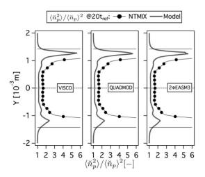
Figure E.3: Comparison of Eulerian and Lagrangian RMS particle segregation  $(\langle \breve{n}_p^2 \rangle / \langle \breve{n}_p \rangle^2)$  at  $20t_{ref}$ . LR\_St033\_# case.
