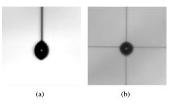
Figure 6.1: Droplet suspending technique: classical fiber (a), cross-fiber (b). Extracted from Chauveau et al. (2008).
