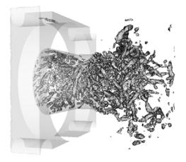
Figure 9.1: Instantaneous isosurface of Q-criterion ( $Q = 2 \cdot 10^8$ ) at the entrance of the chamber. Case RUM\_Ev21.
