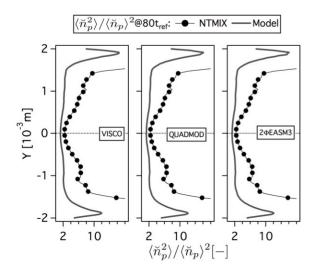
Figure 5.53: Comparison of Eulerian and Lagrangian RMS particle segregation  $(\langle \breve{n}_p^2 \rangle / \langle \breve{n}_p \rangle^2)$  at 80t<sub>ref</sub>. LR\_St033\_# case.
