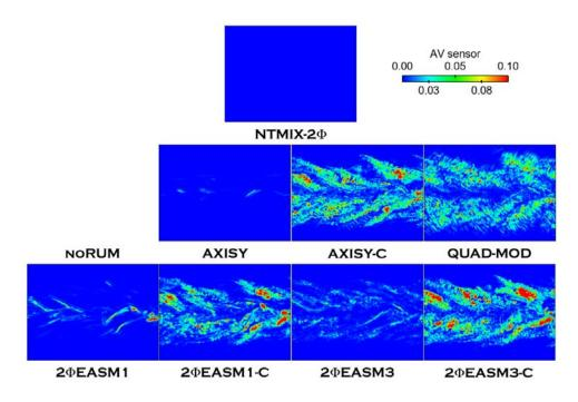
Figure D.24: Comparison of AV sensor levels at  $80t_{ref}$ . LR\_St3\_# case.
