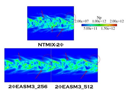
Figure 5.36: Comparison betwenn Lagrangian and Eulerian particle number density instantaneous fields at  $40t_{ref}$ . The Lagrangian computation has been performed in a  $128^3$  grid.  $2\Phi EASM3_256$  corresponds to the Eulerian simulation on a  $256^3$  mesh and  $2\Phi EASM3_512$  to an Eulerian simulation on a  $512^3$  mesh.
