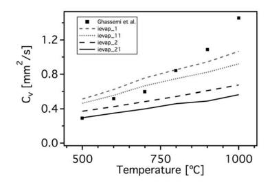
Figure 7.13: Evaporation rates of kerosene as a function of the gaseous temperature. Comparison with experimental results of Ghassemi et al. (2006)
