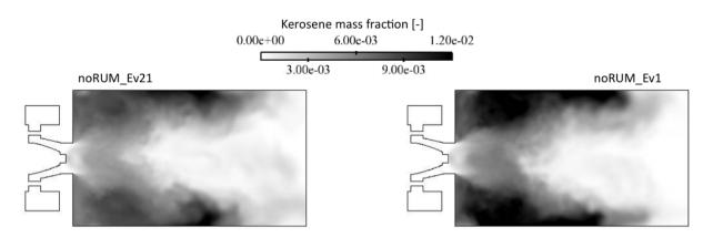
Figure 9.29: Gaseous kerosene mass fraction averaged fields. Cases noRUM\_Ev1 (right) and noRUM\_Ev21 (left).
