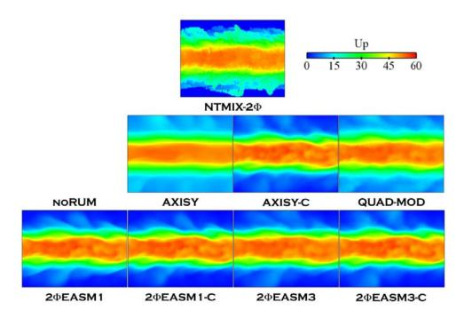
Figure D.19: Comparison of Lagrangian (NTMIX-2 $\Phi$ ) and Eulerian particle velocity magnitude ( $U_p$ ) at 40 $t_{ref}$ . LR\_St3\_# case.
