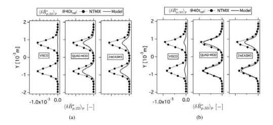
Figure E.14: Comparison of Eulerian and Lagrangian (a) mean deviatoric RUM stress tensor YY component ( $\langle \delta \breve{R}_{p,22}^* \rangle_p$ ) and (b) mean deviatoric RUM stress tensor ZZ component ( $\langle \delta \breve{R}_{p,33}^* \rangle_p$ ) at 40t<sub>ref</sub>. Normalized by the square of the initial particle velocity in X-direction at the center of the slab. LR\_St033\_# case.
