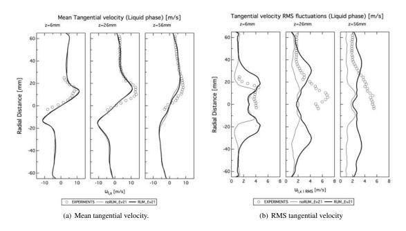
Figure 9.32: Mean and RMS tangential velocity profiles. Liquid phase. Cases noRUM\_Ev21 and RUM\_Ev21. Comparison with the experiments.
