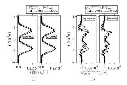
Figure F.12: Comparison of Eulerian and Lagrangian (a) mean production of RUM energy by shear components  $(< P_{RUM}^{Shear} >_p)$  and (b) mean productions of RUM energy by compression  $(< P_{RUM}^{Compression} >_p)$  at  $40t_{ref}$ . Normalized by the square of the initial particle velocity in X-direction at the center of the slab and the reference time  $(t_{ref})$ . HR\_St1\_# case.
