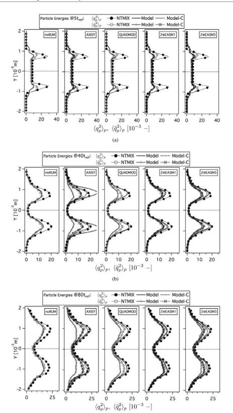
Figure 5.22: Comparison of Eulerian and Lagrangian mean total energy  $(\langle q_p^2 \rangle_p)$  and mean mesoscopic energy  $(\langle \breve{q}_p^2 \rangle_p)$  at 5, 40 and 80 $t_{ref}$ . Normalized by the square of the initial particle velocity in X-direction at the center of the slab. LR\_St1\_# case.
