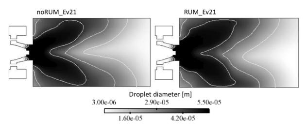
Figure 9.36: Droplet diameter averaged fields. Cases noRUM\_Ev21 (left) and RUM\_Ev21 (right).
