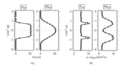
Figure B.1: Comparison of Eulerian and Lagrangian carrier phase velocities in X-direction. HR\_St1\_# case. (a) Mean velocity ( $U_f$ ) and (b) RMS velocity times the fluid density ( $\rho_f U_{f,RMS}$ ) at 5 and  $40t_{ref}$ . Simulations performed with AVBP (—) and NTMIX-2 $\Phi$  (–•–).
