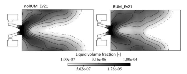
Figure 9.35: Liquid volume fraction averaged fields. Cases noRUM\_Ev21 (left) and RUM\_Ev21 (right).
