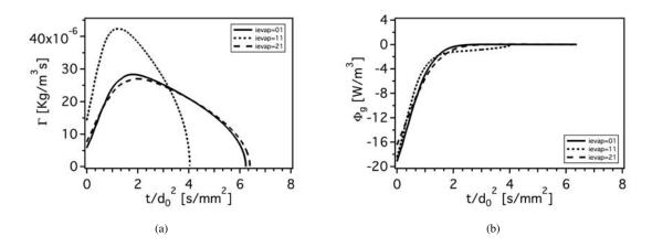
Figure 7.5: Evolution of the mass (a) and heat transfer rates (b). n-heptane,  $T_g = 623K$ ,  $P_g = 1bar$ . Numerical simulations performed using the AS evaporation model.
