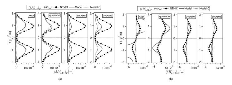
Figure D.6: Comparison of Eulerian and Lagrangian (a) mean deviatoric RUM stress tensor XX component ( $<\delta \breve{R}_{p,11}^* >_p$ ) and (b) mean deviatoric RUM stress tensor XY component ( $<\delta \breve{R}_{p,12}^* >_p$ ) at 40t<sub>ref</sub>. Normalized by the square of the initial particle velocity in X-direction at the center of the slab. LR\_St3\_# case.
