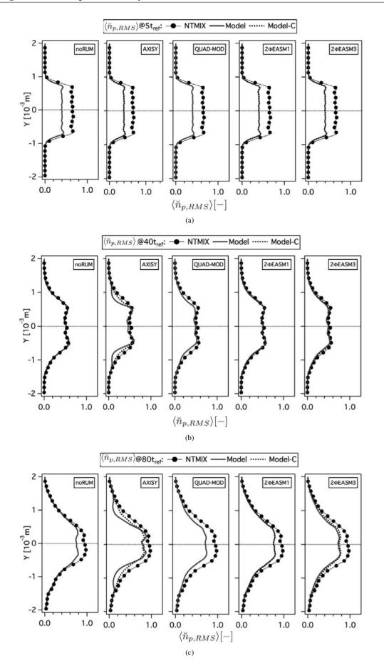
Figure 5.16: Comparison of Eulerian and Lagrangian RMS particle number density ( $\langle \breve{n}_{p,RMS} \rangle$ ) at 5, 40 and 80 $t_{ref}$ . Normalized by the initial particle number density at the center of the slab. LR\_St1\_# case.
