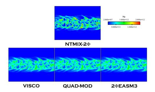
Figure E.15: Comparison of Lagrangian (NTMIX-2 $\Phi$ ) and Eulerian particle number density ( $N_p$ ) at 20t<sub>ref</sub>. LR\_St033\_# case.
