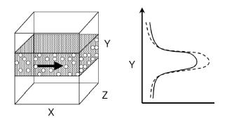
Figure 5.3: Simplified sketch of the particle-laden turbulent planar jet configuration. (Extracted from Vermorel (2003)).
