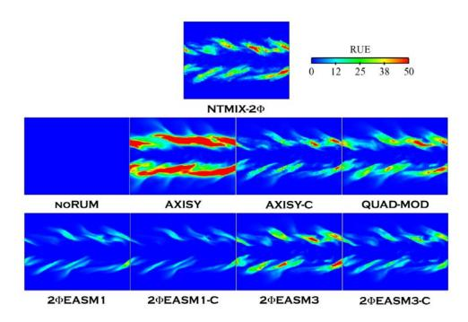
Figure C.6: Comparison of Lagrangian (NTMIX-2 $\Phi$ ) and Eulerian Random Uncorrelated Energy at 40 $t_{ref}$ . LR\_St1\_# case.
