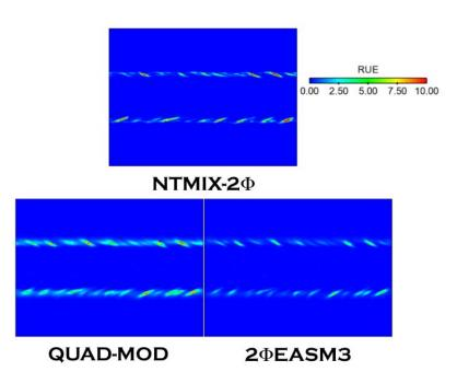
Figure F.19: Comparison of Lagrangian (NTMIX-2 $\Phi$ ) and Eulerian Random Uncorrelated Energy at 5t<sub>ref</sub>. HR\_St1\_# case.
