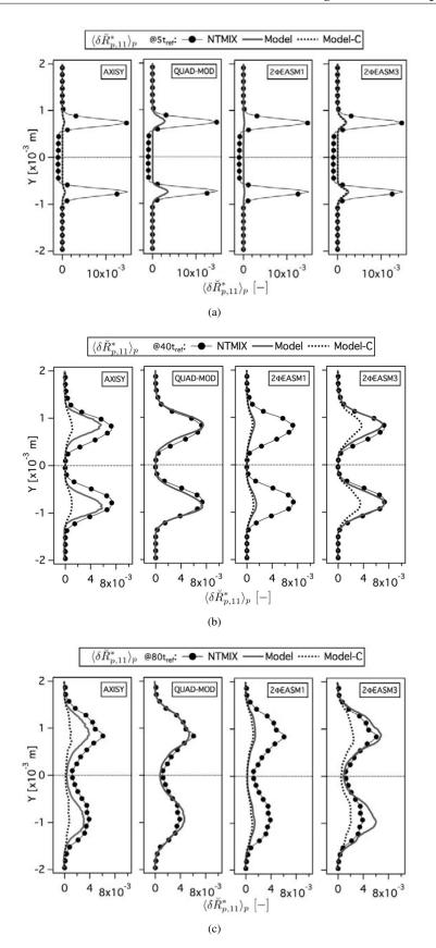
Figure 5.25: Comparison of Eulerian and Lagrangian mean deviatoric RUM stress tensor XX component ( $\langle \delta \breve{R}_{p,11}^* \rangle_p$ ) at 5, 40 and 80t<sub>ref</sub>. Normalized by the square of the initial particle velocity in X-direction at the center of the slab. LR\_St1\_# case.
