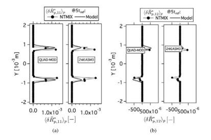
Figure F.6: Comparison of Eulerian and Lagrangian (a) mean deviatoric RUM stress tensor XX component ( $\langle \delta \vec{R}_{p,11}^* \rangle_p$ ) and (b) mean deviatoric RUM stress tensor XY component ( $\langle \delta \vec{R}_{p,12}^* \rangle_p$ ) at  $5t_{ref}$ . Normalized by the square of the initial particle velocity in X-direction at the center of the slab. HR\_St1\_# case.
