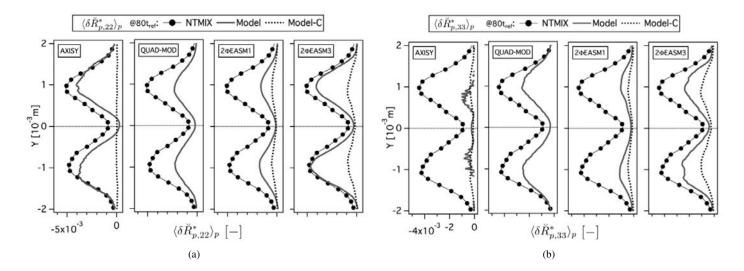
Figure D.15: Comparison of Eulerian and Lagrangian (a) mean deviatoric RUM stress tensor YY component ( $<\delta \breve{R}^*_{p,22} >_p$ ) and (b) mean deviatoric RUM stress tensor ZZ component ( $<\delta \breve{R}^*_{p,33} >_p$ ) at  $80t_{ref}$ . Normalized by the square of the initial particle velocity in X-direction at the center of the slab. LR\_St3\_# case.
