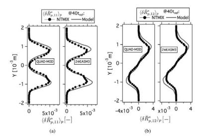
Figure F.13: Comparison of Eulerian and Lagrangian (a) mean deviatoric RUM stress tensor XX component ( $< \delta \tilde{R}_{p,11}^* >_p$ ) and (b) mean deviatoric RUM stress tensor XY component ( $< \delta \tilde{R}_{p,12}^* >_p$ ) at 40t<sub>ref</sub>. Normalized by the square of the initial particle velocity in X-direction at the center of the slab. HR\_St1\_# case.
