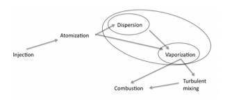
Figure 1.6: Sketch of the principal phenomena related to the dispersed phase in combustion chambers.
