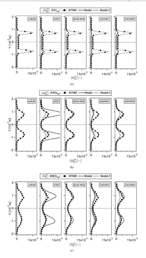
Figure 5.21: Comparison of Eulerian and Lagrangian mean Random Uncorrelated Energy  $(\langle \delta \check{\theta}_p \rangle_p)$  at 5, 40 and 80 $t_{ref}$ . Normalized by the square of the initial particle velocity in X-direction at the center of the slab. LR\_St1\_# case.
