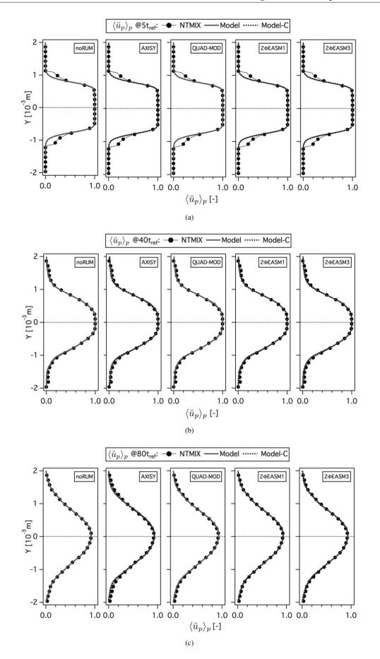
Figure 5.15: Comparison of Eulerian and Lagrangian mean particle velocity in X-direction ( $\langle \breve{u}_p \rangle_p$ ) at 5, 40 and 80 $t_{ref}$ . Normalized by the initial particle velocity in X-direction at the center of the slab. LR\_St1\_# case.
