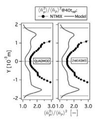
Figure F.10: Comparison of Eulerian and Lagrangian RMS particle segregation  $(\langle \breve{n}_p^2 \rangle / \langle \breve{n}_p \rangle^2)$  at  $40t_{ref}$ . HR\_St1\_# case.
