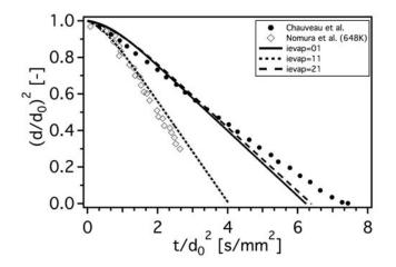
Figure 7.3: Temporal evolution of the non-dimensional droplet surface. n-heptane,  $T_g = 623K$ ,  $P_g = 1bar$ . Numerical simulations performed using the AS evaporation model. Experimental results of Chauveau et al. (2008) and Nomura et al. (1996).
