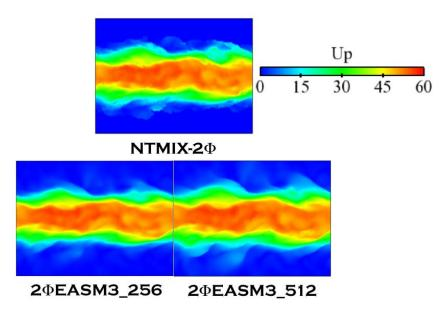
Figure 5.37: Comparison between Lagrangian and Eulerian particle velocity instantaneous fields at  $40t_{ref}$ . The Lagrangian computation has been performed in a  $128^3$  grid.  $2\Phi EASM3_256$  corresponds to the Eulerian simulation on a  $256^3$  mesh and  $2\Phi EASM3_512$  to an Eulerian simulation on a  $512^3$  mesh.
