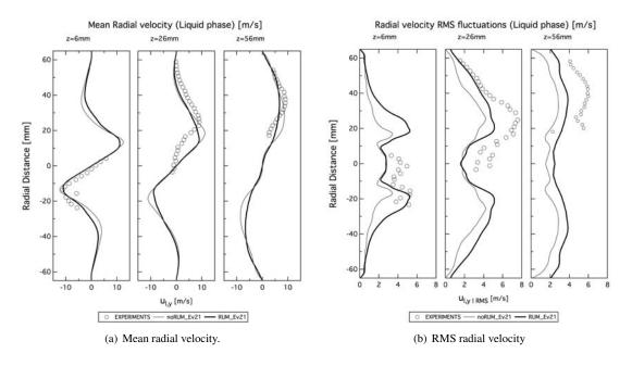
Figure 9.31: Mean and RMS radial velocity profiles. Liquid phase. Cases noRUM\_Ev21 and RUM\_Ev21. Comparison with the experiments.
