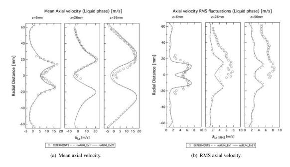
Figure 9.19: Mean and RMS axial velocity profiles. Liquid phase. Cases noRUM\_Ev1 and noRUM\_Ev21. Comparison with the experiments.
