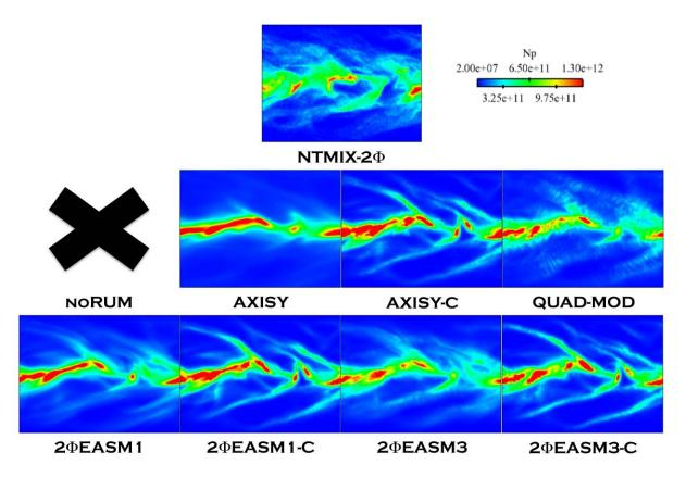
Figure 5.42: Comparison of Lagrangian (NTMIX-2 $\Phi$ ) and Eulerian particle number density fields ( $N_p$ ) at 120 $t_{ref}$ . LR\_St3\_# case.
