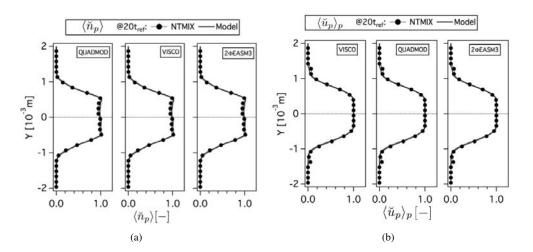
Figure E.1: Comparison of Eulerian and Lagrangian (a) mean particle number density ( $\langle \breve{n}_p \rangle$ , normalized by the initial particle number density at the center of the slab) and (b) mean particle velocity in X-direction ( $\langle \breve{u}_p \rangle_p$ , normalized by the initial particle velocity in X-direction at the center of the slab) at 20t<sub>ref</sub>. LR\_St033\_# case.
