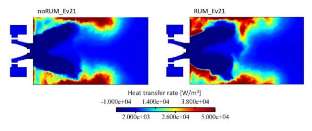
Figure 9.39: Evaporation heat transfer rate instantaneous fields. Cases noRUM\_Ev21 (left) and RUM\_Ev21 (right).
