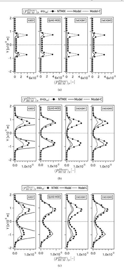
Figure 5.23: Comparison of Eulerian and Lagrangian mean productions of RUM energy by shear ( $\langle P_{RUM}^{Shear} \rangle_p$ ) at 5, 40 and 80t<sub>ref</sub>. Normalized by the square of the initial particle velocity in X-direction at the center of the slab and the reference time (t<sub>ref</sub>). LR\_St1\_# case.
