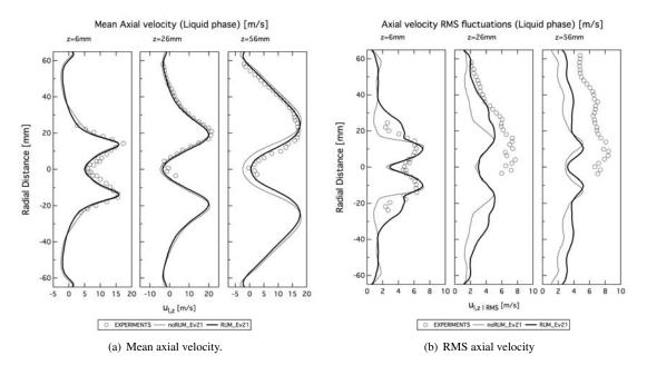
Figure 9.30: Mean and RMS axial velocity profiles. Liquid phase. Cases noRUM\_Ev21 and RUM\_Ev21. Comparison with the experiments.
