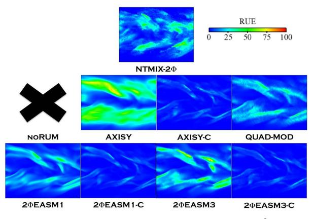
Figure 5.48: Comparison of Lagrangian (NTMIX-2 $\Phi$ ) and Eulerian Random Uncorrelated Energy ( $\delta q_p^2$ ) at 120 $t_{ref}$ . LR\_St3\_# case.
