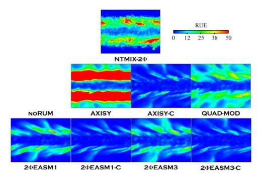
Figure D.21: Comparison of Lagrangian (NTMIX-2 $\Phi$ ) and Eulerian Random Uncorrelated Energy at 40t<sub>ref</sub>. LR\_St3\_# case.
