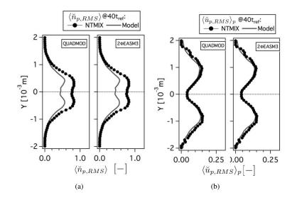
Figure F.9: Comparison of Eulerian and Lagrangian (a) RMS particle number density ( $\langle \breve{n}_{p,RMS} \rangle$ , normalized by the initial particle number density at the center of the slab) and (b) RMS particle velocity in X-direction ( $\langle \breve{u}_{p,RMS} \rangle_p$ , normalized by the initial particle number density at the center of the slab)at 40 $t_{ref}$ . HR\_St1\_# case.
