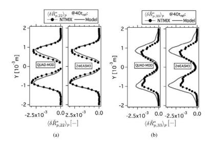
Figure F.14: Comparison of Eulerian and Lagrangian (a) mean deviatoric RUM stress tensor YY component ( $<\delta \breve{R}^*_{p,22} >_p$ ) and (b) mean deviatoric RUM stress tensor ZZ component ( $<\delta \breve{R}^*_{p,33} >_p$ ) at 40t<sub>ref</sub>. Normalized by the square of the initial particle velocity in X-direction at the center of the slab. HR\_St1\_# case.
