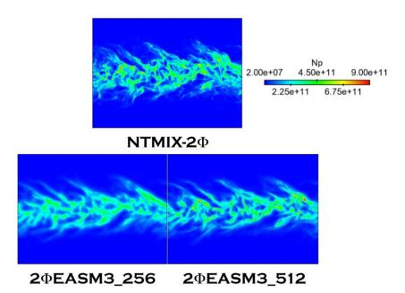
Figure 5.75: Comparison Lagrangian and Eulerian particle number density instantaneous fields at  $40t_{ref}$ . The Lagrangian computation has been performed in a  $128^3$  mesh grid.  $2\Phi EASM3_256$  corresponds to the Eulerian simulation on a  $256^3$  mesh and  $2\Phi EASM3_512$  to an Eulerian simulation on a  $512^3$  mesh.
