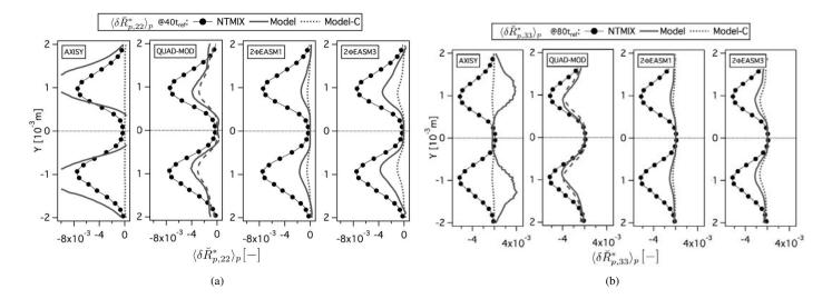
Figure D.7: Comparison of Eulerian and Lagrangian (a) mean deviatoric RUM stress tensor YY component ( $<\delta \breve{R}^*_{p,22} >_p$ ) and (b) mean deviatoric RUM stress tensor ZZ component ( $<\delta \breve{R}^*_{p,33} >_p$ ) at 40t<sub>ref</sub>. Normalized by the square of the initial particle velocity in X-direction at the center of the slab. LR\_St3\_# case.
