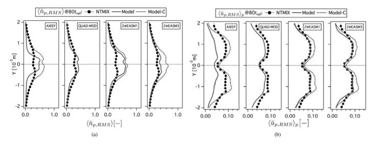
Figure D.10: Comparison of Eulerian and Lagrangian (a) RMS particle number density ( $\langle \breve{n}_{p,RMS} \rangle$ , normalized by the initial particle number density at the center of the slab) and (b) RMS particle velocity in X-direction ( $\langle \breve{u}_{p,RMS} \rangle_p$ , normalized by the initial particle number density at the center of the slab)at 80t<sub>ref</sub>. LR\_St3\_# case.
