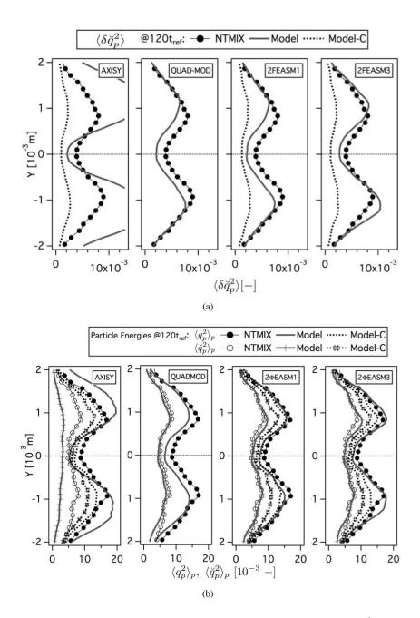
Figure 5.44: Comparison of Eulerian and Lagrangian (a) mean Random Uncorrelated Energy  $(\delta q_p^2)$  and (b) mean total  $(q_p^2)$ and mesoscopic  $(\breve{q}_p^2)$  particle energies at  $120t_{ref}$ . Normalized by the square of the initial particle velocity in X-direction at the center of the slab. LR\_St3\_# case.
