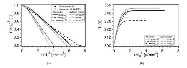
Figure 7.7: Comparison of the evolution of the non-dimensional droplet surface (a) and temperature (b) for the different evaporation models. n-heptane droplet,  $T_g = 623K$ ,  $P_g = 1bar$ . Simulations performed with the Spalding and the AS evaporation models. Experimental results of Chauveau et al. (2008) and Nomura et al. (1996).
