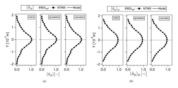
Figure 5.51: Comparison of Eulerian and Lagrangian (a) mean particle number density ( $\langle \check{n}_p \rangle$ , normalized by the initial particle number density at the center of the slab) and (b) mean particle velocity in X-direction ( $\langle \check{u}_p \rangle_p$ , normalized by the initial particle velocity in X-direction at the center of the slab) at 80t<sub>ref</sub>. LR\_St033\_# case.
