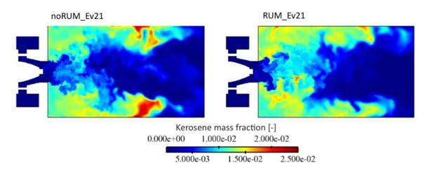
Figure 9.40: Gaseous kerosene mass fraction instantaneous fields. Cases noRUM\_Ev21 (left) and RUM\_Ev21 (right).
