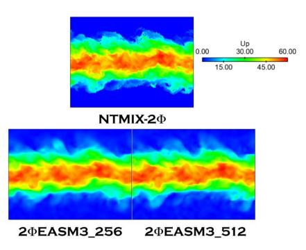
Figure 5.76: Comparison Lagrangian and Eulerian particle velocity instantaneous fields at  $40t_{ref}$ . The Lagrangian computation has been performed in a  $128^3$  mesh grid.  $2\Phi EASM3_256$  corresponds to the Eulerian simulation on a  $256^3$  mesh and  $2\Phi EASM3_512$  to an Eulerian simulation on a  $512^3$  mesh.
