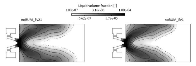
Figure 9.23: Liquid volume fraction time-averaged fields. Cases noRUM\_Ev1 (right) and noRUM\_Ev21 (left).
