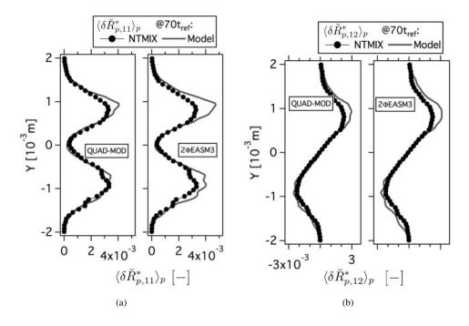
Figure 5.68: Comparison of Eulerian and Lagrangian (a) mean deviatoric RUM stress tensor XX component ( $<\delta \tilde{R}_{p,11}^* >_p$ ) and (b) mean deviatoric RUM stress tensor XY component ( $<\delta \tilde{R}_{p,12}^* >_p$ ) at 70 $t_{ref}$ . Normalized by the square of the initial particle velocity in X-direction at the center of the slab. HR\_St1\_# case.
