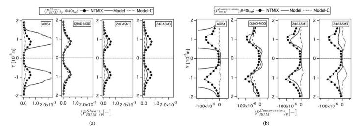
Figure D.5: Comparison of Eulerian and Lagrangian (a) mean production of RUM energy by shear components  $(\langle P_{RUM}^{Shear} \rangle_p)$  and (b) mean productions of RUM energy by compression  $(\langle P_{RUM}^{Compression} \rangle_p)$  at  $40t_{ref}$ . Normalized by the square of the initial particle velocity in X-direction at the center of the slab and the reference time  $(t_{ref})$ . LR\_St3\_# case.
