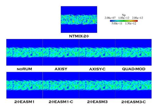
Figure C.1: Comparison of Lagrangian (NTMIX-2 $\Phi$ ) and Eulerian particle number density ( $N_p$ ) at 5t<sub>ref</sub>. LR\_St1\_# case.
