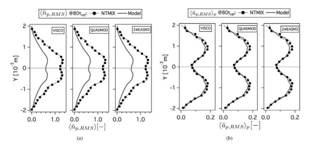
Figure 5.52: Comparison of Eulerian and Lagrangian (a) RMS particle number density ( $\langle \breve{n}_{p,RMS} \rangle$ , normalized by the initial particle number density at the center of the slab) and (b) RMS particle velocity in X-direction ( $\langle \breve{u}_{p,RMS} \rangle_p$ , normalized by the initial particle number density at the center of the slab) at 80t<sub>ref</sub>. LR\_St033\_# case.
