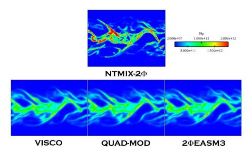
Figure 5.54: Comparison of Lagrangian (NTMIX-2 $\Phi$ ) and Eulerian particle number density ( $N_p$ ) at 80 $t_{ref}$ . LR\_St033\_# case.
