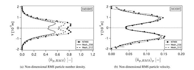
Figure 5.72: Comparison Lagrangian and Eulerian results. The Lagrangian computation has been performed in a 128<sup>3</sup> mesh grid. Mesh\_256 corresponds to the Eulerian simulation on a 256<sup>3</sup> mesh and Mesh\_512 to an Eulerian simulation on a 512<sup>3</sup> mesh.
