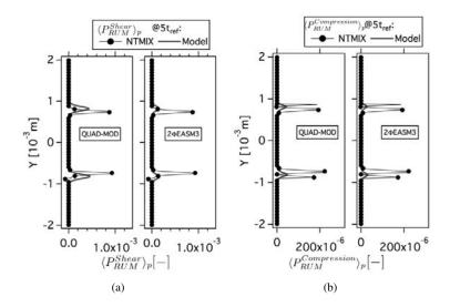
Figure F.5: Comparison of Eulerian and Lagrangian (a) mean production of RUM energy by shear components  $(< P_{RUM}^{Shear} >_p)$  and (b) mean productions of RUM energy by compression  $(< P_{RUM}^{Compression} >_p)$  at  $5t_{ref}$ . Normalized by the square of the initial particle velocity in X-direction at thecenter of the slab and t[h!]e reference time  $(t_{ref})$ . HR\_St1\_# case.
