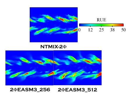
Figure 5.38: Comparison between Lagrangian and Eulerian RUE instantaneous fields at  $40t_{ref}$ . The Lagrangian computation has been performed in a  $128^3$  grid.  $2\Phi EASM3_256$  corresponds to the Eulerian simulation on a  $256^3$  mesh and  $2\Phi EASM3_512$  to an Eulerian simulation on a  $512^3$  mesh.
