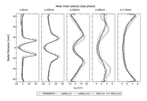
Figure 9.7: Mean axial velocity profiles. Gaseous phase.
