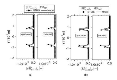
Figure F.7: Comparison of Eulerian and Lagrangian (a) mean deviatoric RUM stress tensor YY component ( $\langle \delta \breve{R}_{p,22}^* \rangle_p$ ) and (b) mean deviatoric RUM stress tensor ZZ component ( $\langle \delta \breve{R}_{p,33}^* \rangle_p$ ) at  $5t_{ref}$ . Normalized by the square of the initial particle velocity in X-direction at the center of the slab. HR\_St1\_# case.
