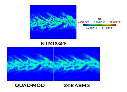
Figure F.16: Comparison of Lagrangian (NTMIX-2 $\Phi$ ) and Eulerian particle number density ( $N_p$ ) at 40 $t_{ref}$ . HR\_St1\_# case.
