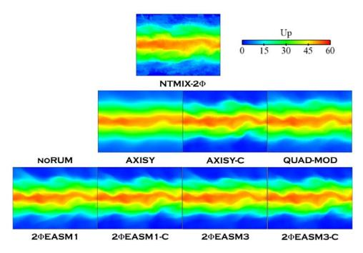
Figure D.20: Comparison of Lagrangian (NTMIX-2 $\Phi$ ) and Eulerian particle velocity magnitude ( $U_p$ ) at 80 $t_{ref}$ . LR\_St3\_# case.
