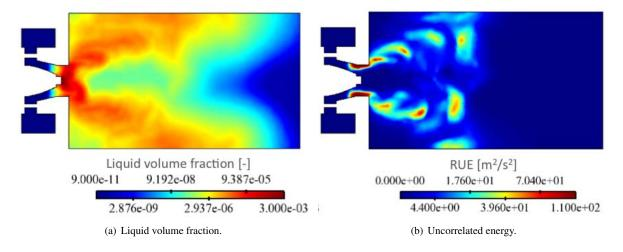
Figure 9.41: Instantaneous fields of (a) liquid volume fraction and (b) RUE at t = 48 ms. Case RUM\_Ev21.
