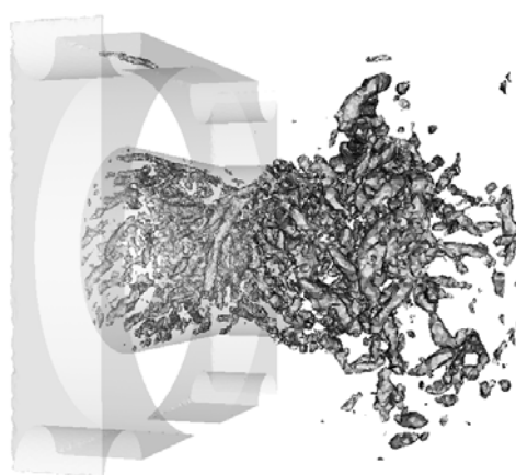
Figure 9.1: Instantaneous isosurface of Q -criterion ( Q = 2 \cdot 10^8 ) at the entrance of the chamber. Case RUM_Ev21.
