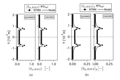
Figure F.2: Comparison of Eulerian and Lagrangian (a) RMS particle number density ( $\langle \check{n}_{p,RMS} \rangle$ , normalized by the initial particle number density at the center of the slab) and (b) RMS particle velocity in X-direction ( $\langle \check{u}_{p,RMS} \rangle_p$ , normalized by the initial particle number density at the center of the slab) at  $5t_{ref}$ . HR\_St1\_# case.
