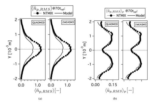
Figure 5.62: Comparison of Eulerian and Lagrangian (a) RMS particle number density ( $\langle \breve{n}_{p,RMS} \rangle$ , normalized by the initial particle number density at the center of the slab) and (b) RMS particle velocity in X-direction ( $\langle \breve{u}_{p,RMS} \rangle_p$ , normalized by the initial particle number density at the center of the slab)at 70t<sub>ref</sub>. HR\_St1\_# case.
