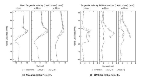
Figure 9.22: Mean and RMS tangential velocity profiles. Liquid phase. Cases noRUM\_Ev1 and noRUM\_Ev21. Comparison with the experiments.
