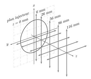
Figure 8.2: Sketch of the experimental measurement planes (Extracted from Sanjosé (2009)).
