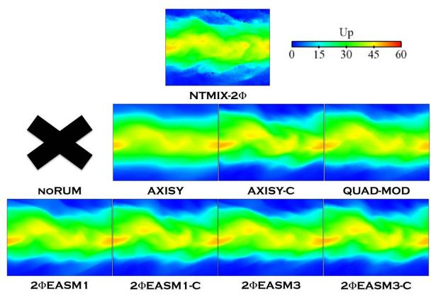
Figure 5.43: Comparison of Lagrangian (NTMIX-2 $\Phi$ ) and Eulerian particle velocity magnitude fields ( $U_p$ ) at 120 $t_{ref}$ . LR\_St3\_# case.
