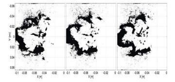
Figure 9.17: Tomographic visualization of the fuel spray. Binarized thresholded snapshots. Source Linassier et al. (2011).
