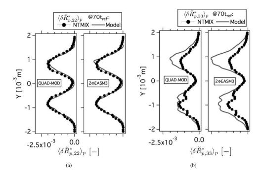
Figure 5.69: Comparison of Eulerian and Lagrangian (a) mean deviatoric RUM stress tensor YY component ( $< \delta \ddot{R}^*_{p,22} >_p$ ) and (b) mean deviatoric RUM stress tensor ZZ component ( $< \delta \ddot{R}^*_{p,33} >_p$ ) at 70t<sub>ref</sub>. Normalized by the square of the initial particle velocity in X-direction at the center of the slab. HR\_St1\_# case.
