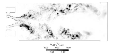
Figure 9.14: Ratio of artificial to laminar viscosity corresponding to an instantaneous solution of Case RUM\_Ev21.
