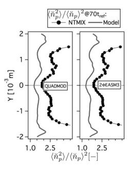
Figure 5.63: Comparison of Eulerian and Lagrangian RMS particle segregation  $(\langle \breve{n}_p^2 \rangle / \langle \breve{n}_p \rangle^2)$  at 70t<sub>ref</sub>. HR\_St1\_# case.
