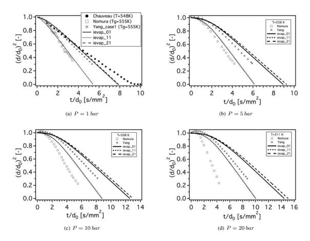
Figure 7.10: Temporal evolution of the non-dimensional droplet surface. Evaporation of n-heptane droplet. T = 548K. P = 1bar (a), P = 5bar (b), P = 10bar (c) and P = 20bar (d). Comparison of numerical results performed using AS evaporation model, case 1 in Yang & Wong (2001) and eperimental results of Nomura et al. (1996).
