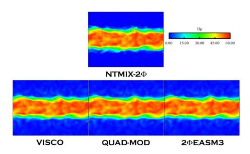
Figure E.17: Comparison of Lagrangian (NTMIX-2 $\Phi$ ) and Eulerian particle velocity magnitude ( $U_p$ ) at 20 $t_{ref}$ . LR\_St033\_# case.
