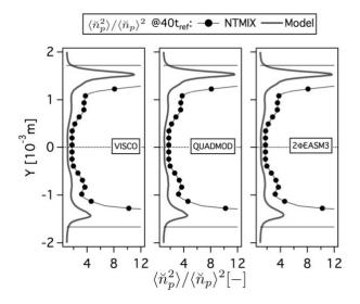
Figure E.10: Comparison of Eulerian and Lagrangian RMS particle segregation  $(\langle \breve{n}_p^2 \rangle / \langle \breve{n}_p \rangle^2)$  at 40t<sub>ref</sub>. LR\_St033\_# case.
