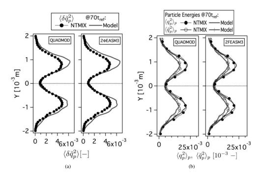
Figure 5.66: Comparison of Eulerian and Lagrangian (a) mean Random Uncorrelated Energy  $(\delta q_p^2)$  and (b) mean total  $(q_p^2)$ and mesoscopic  $(\langle \breve{q}_p^2 \rangle_p)$  particle energies at 70 $t_{ref}$ . Normalized by the square of the initial particle velocity in X-direction at the center of the slab. HR\_St1\_# case.
