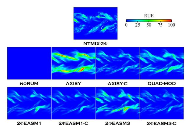
Figure 5.29: Comparison of Lagrangian (NTMIX-2 $\Phi$ ) and Eulerian Random Uncorrelated Energy at 80 $t_{ref}$ . LR\_St1\_# case.
