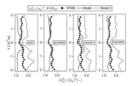
Figure 5.41: Comparison of Eulerian and Lagrangian RMS particle segregation  $(\langle \tilde{n}_p^2 \rangle / \langle \tilde{n}_p \rangle^2)$  at 120 $t_{ref}$ . LR\_St3\_# case.
