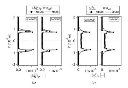
Figure F.4: Comparison of Eulerian and Lagrangian (a) mean Random Uncorrelated Energy ( $\langle \delta \breve{q}_p \rangle_p$ ) and (b) mean mesoscopic ( $\langle \breve{q}_p^2 \rangle_p$ ) particle energies at 5t<sub>ref</sub>. Normalized by the square of the initial particle velocity in X-direction at the center of the slab. HR\_St1\_# case.
