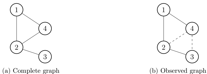
Figure 1.10: Illustration of the link prediction task. In the left panel, we have the true complete graph which is not observed. The right panel describes our observation: the true edges (1, 2) , (1, 4) , (2, 3) are observed, along with the non-existent edge (1, 3) , but the information concerning the pairs (2, 4) and (3, 4) is missing. We aim to decide for (2, 4) and (3, 4) whether there is a true edge or not.
