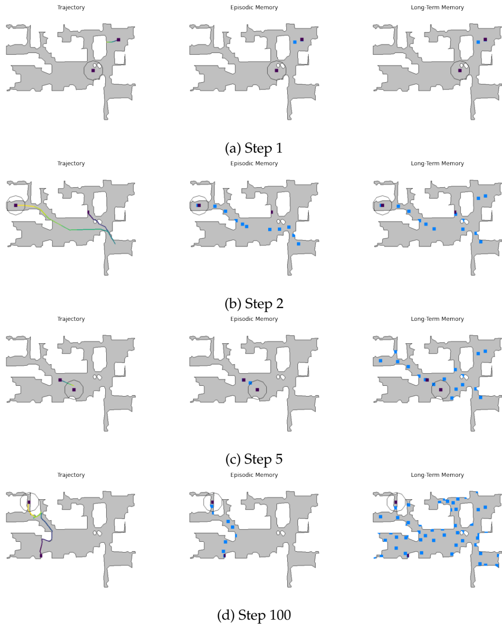
FIGURE 3.9: Visualization of the agent's trajectory, episodic and long-term memories for first, second, fifth and 100th episode in the Eastville environment. The start and goal locations are shown in black, goal location being circled by a line showing the success area. The blue points represent the location of the episodic and long-term memory vectors. The episodic memory is reset after each episode, while the long-term memory remains for 100 episodes in the same scene.
