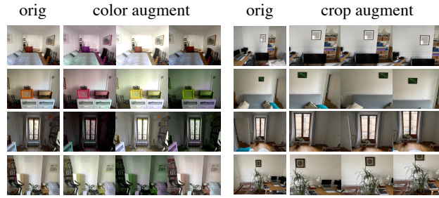
FIGURE 3.3: Illustration of data augmentation that we use to train our model. We consider both color jittering (left) and random crops (right). For a panoramic observation with v views, the parameters of the augmentation are sampled independently.
