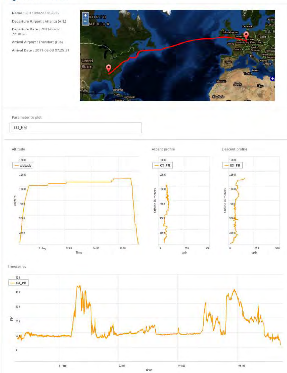
Figure 3.4: Example of IAGOS O 3 data measured during a single flight from Atlanta to Frankfurt. Top panel: the trajectory of the aircraft. Middle panel: the evolution of the aircraft altitude (left); O 3 measurements (in ppb) during the ascent (middle) and descent (right) phase. Bottom: O 3 measurements (in ppb) during the cruise phase. Source: https://www.iagos.org/
