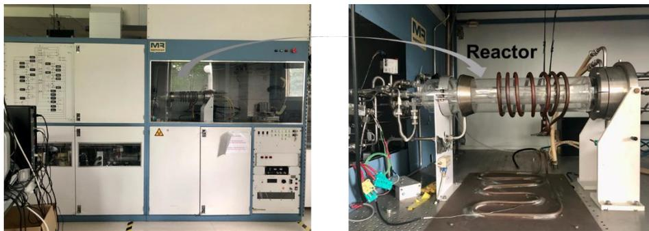
Figure 2-1. MOCVD machine and reactor in GEMaC.
