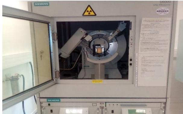
Figure 2-2. Photograph of X-ray diffractometer Bruker-Siemens D5000, in Bragg-Brentano configuration, in GEMaC.
