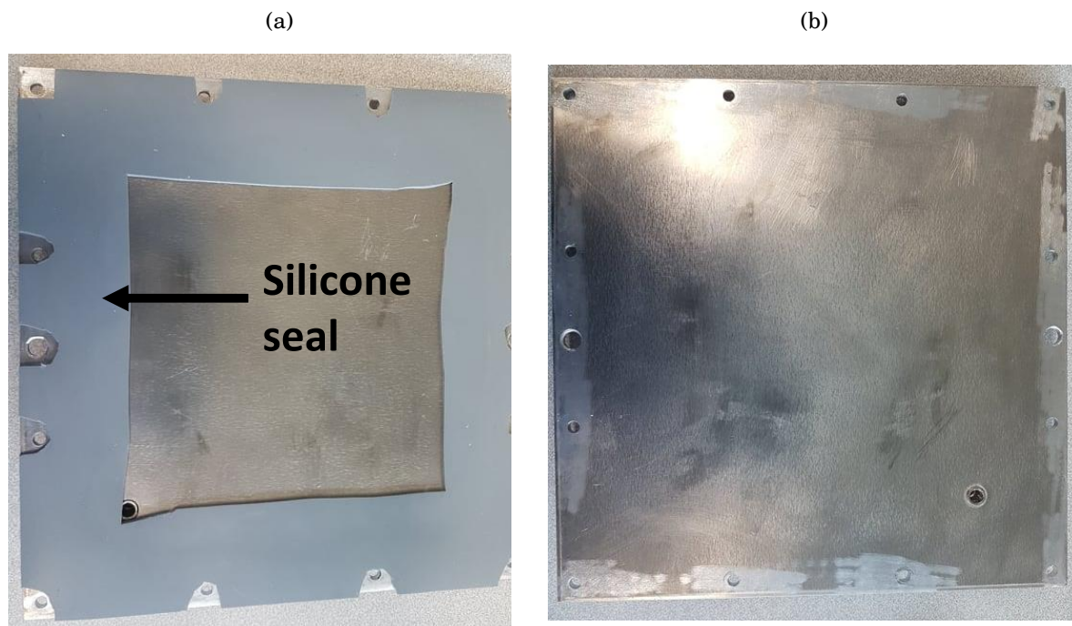
Figure 4.5: Mold preparation for VIC process
