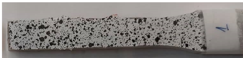
Figure 4.21: Example of a speckle pattern
