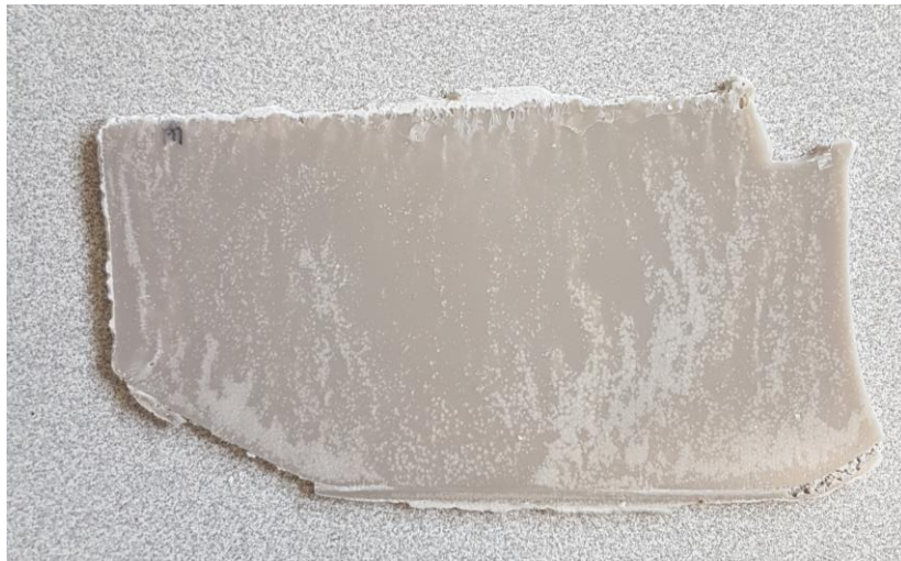
Figure 4.3: Composite manufactured by the CSM process
