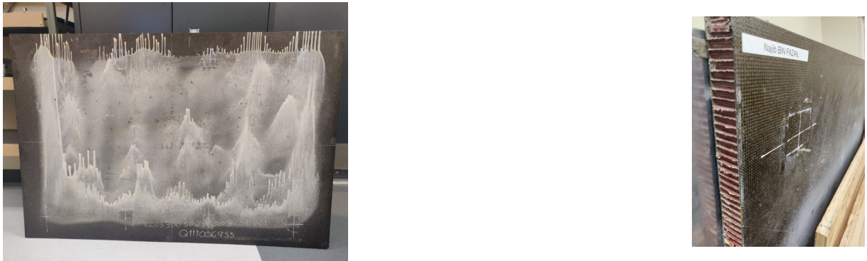
Figure III.17: Sandwich carbon fiber honeycomb panel.
