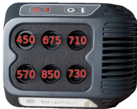
Figure 3.13 – Disposition of each band on the Airphen multi-sensors camera
