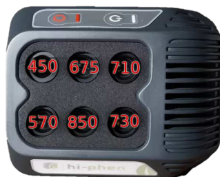
Figure 6.3 – The Airphen six-band multispectral camera
