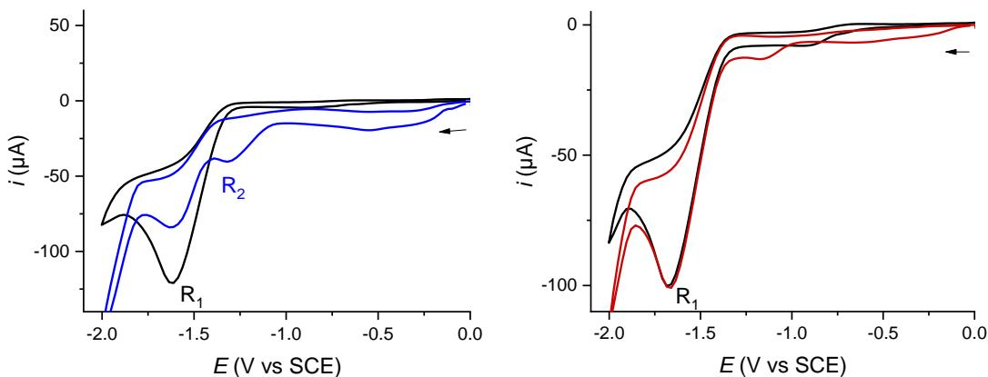
**Figure 11:** Cyclic voltammetry (CV) performed toward reduction potential of a 4 mM solution in CH<sub>2</sub>Cl<sub>2</sub> containing 0.1 M of *n*-Bu<sub>4</sub>NBF<sub>4</sub> using a glassy carbon working electrode (d = 3 mm) with a Pt wire as counter-electrode and saturated calomel electrode (SCE) as reference electrode, at a scan rate of 0.1 V s<sup>-1</sup> at 20 °C. Left: Black curve: **267** alone, Blue curve: **267**
