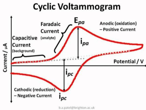
**Figure 9:** Cyclic voltammetry profile
