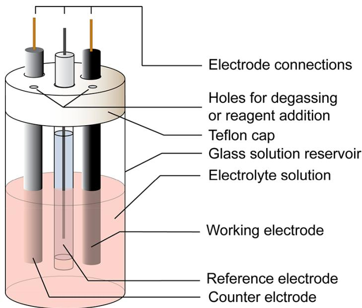
**Figure 10 :** Schematic representation of an electrochemical cell for CV experiments
